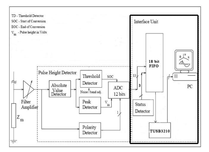
A) The Pulse Height Detector transmits a 12- bit resolution absolute value detector data, and a 1-bit polarity bit detector data. Along with this, the ADC used to digitize the Pulse Height transmits an EOC( End Of Conversion) Signal.
