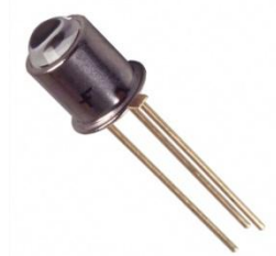
L14G2: The Phototransistor we are using
