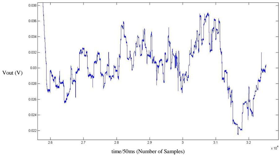
The above figure shows the variation of the LPF output for a fixed input. We can see the value to vary by around  $\pm 10$  mV. We should note here that the minimum resolution of the microcontroller ADC used to take in the output values is 5 mV. Hence the observed errors are quite reasonable for the resolution of ADC we have used.
