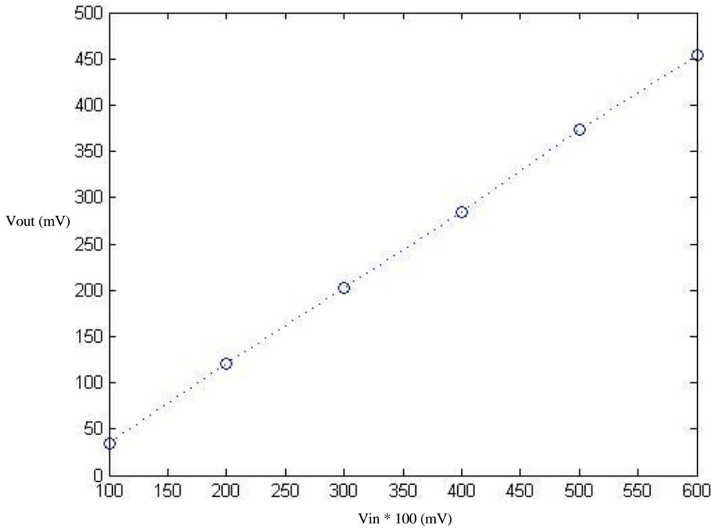
The plot is still quite linear which displays the ability of the instrument to work at these low SNR values.
