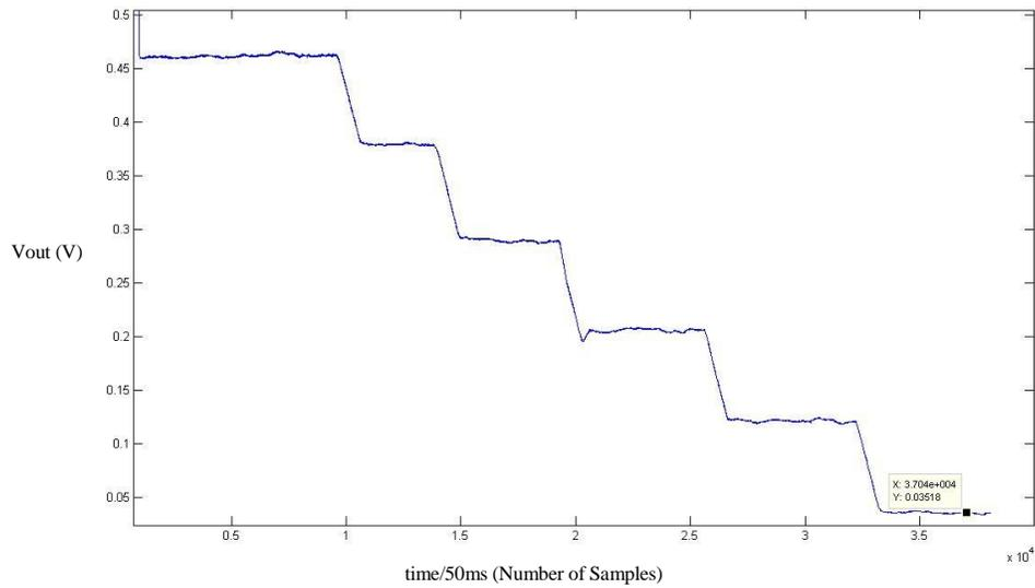
The output of the LPF is shown in the above figure. The  $V_i$  was decreased in the steps of 1mV each time.
