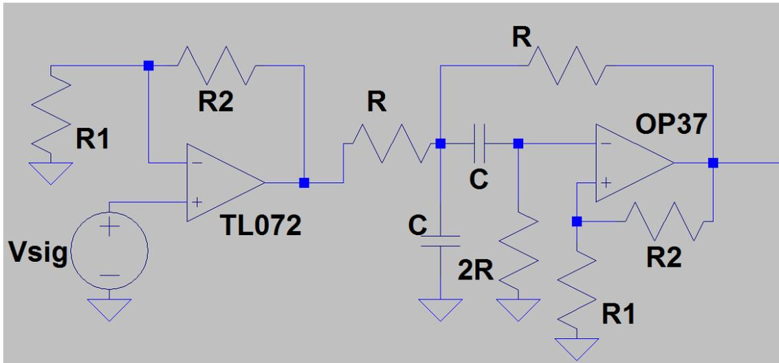
The Center frequency of the Sallen key can be changed simply by changing the resistor value R. For this we used digital potentiometer ICs from Analog Electronics (AD5421BRZxx) that can be controlled by I2C protocol from a microcontroller. For this we also wrote an automatic frequency detection code that would detect the frequency of the reference signal. Then we can accordingly set the value of R for the center frequency.
