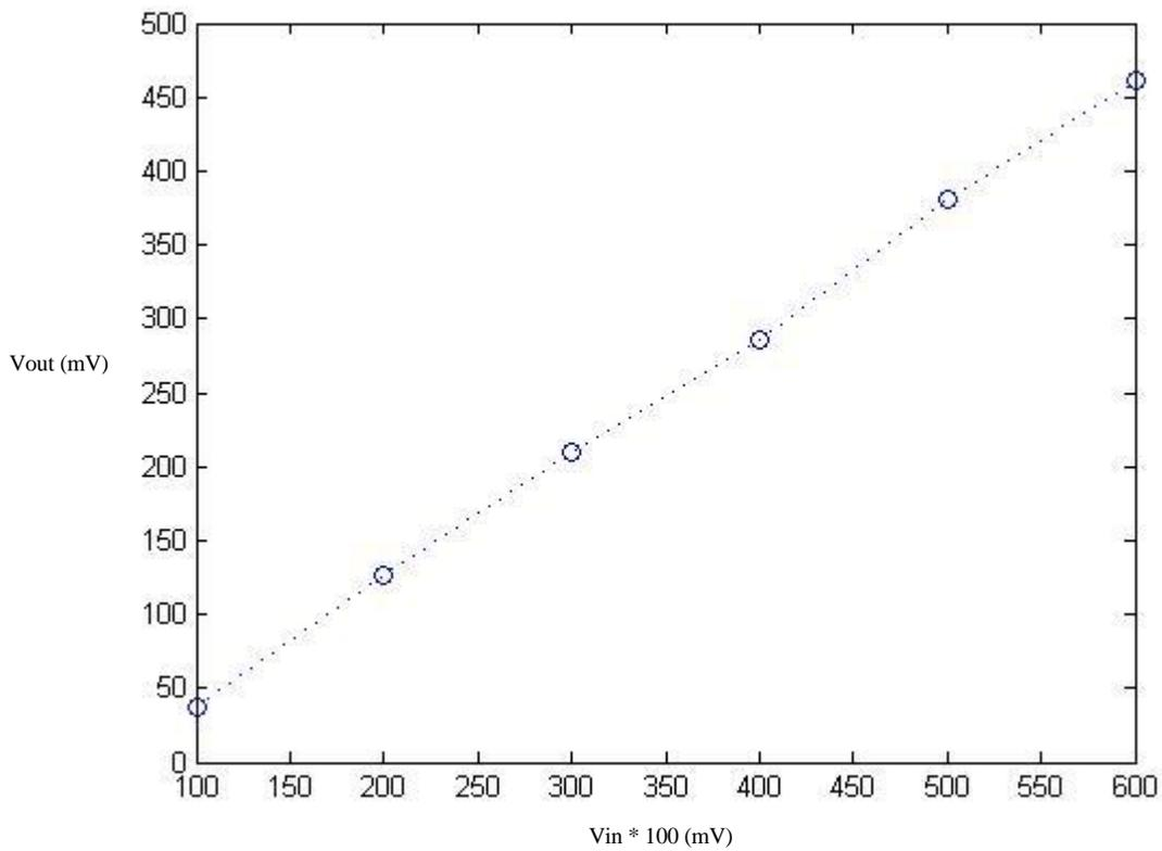
The above figure is a zoomed image of the previous figure. We can see the rise in the LPF output as the input voltage was increased in steps of 1mV.
