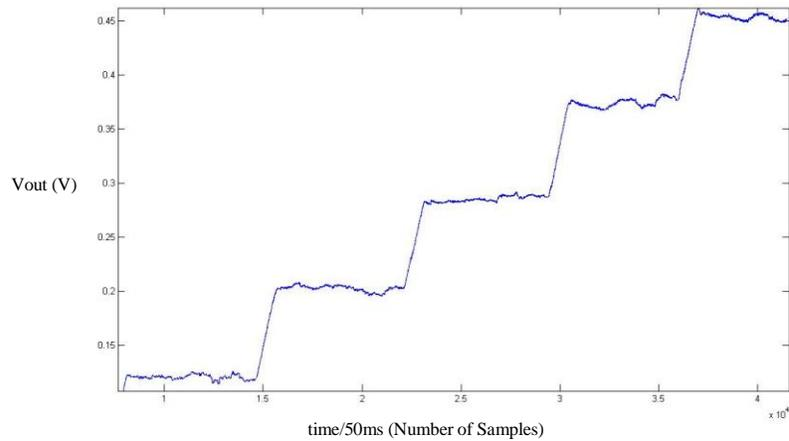
The above figure shows the LPF output. We can see now that because of the increased noise power, the output of the LPF is not very stable and deviates by a small amount from the expected result. This is an indication of the failure of the instrument to give correct results as the SNR decreases. We quantify this value a little later.
