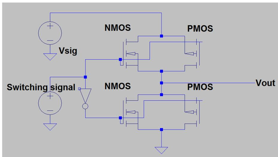
The phase sensitive detection is performed by switching the output of the preprocessing block on two parallel channels with the switching signals 90 degrees out of phase.
