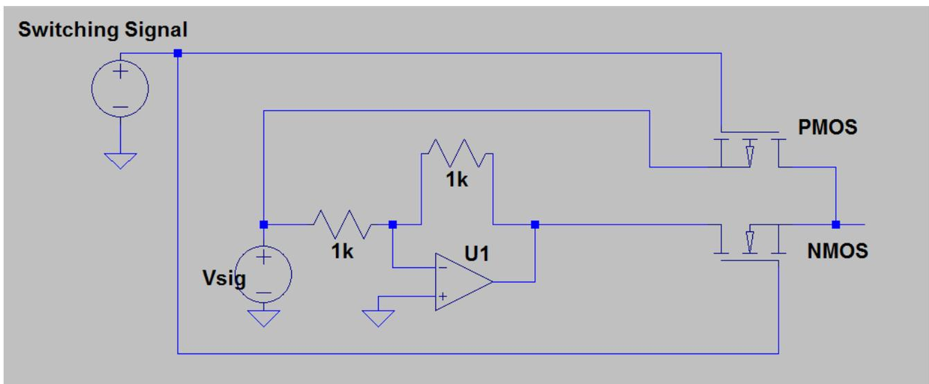
The above circuit allows us to have a bipolar mixing giving the desired mixing by -1 and 1.
