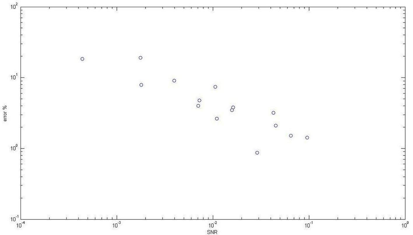
The above plot depicts the trend in the variation of the error % with the SNR. The error in the measurement increases with the decrease in SNR as expected.
