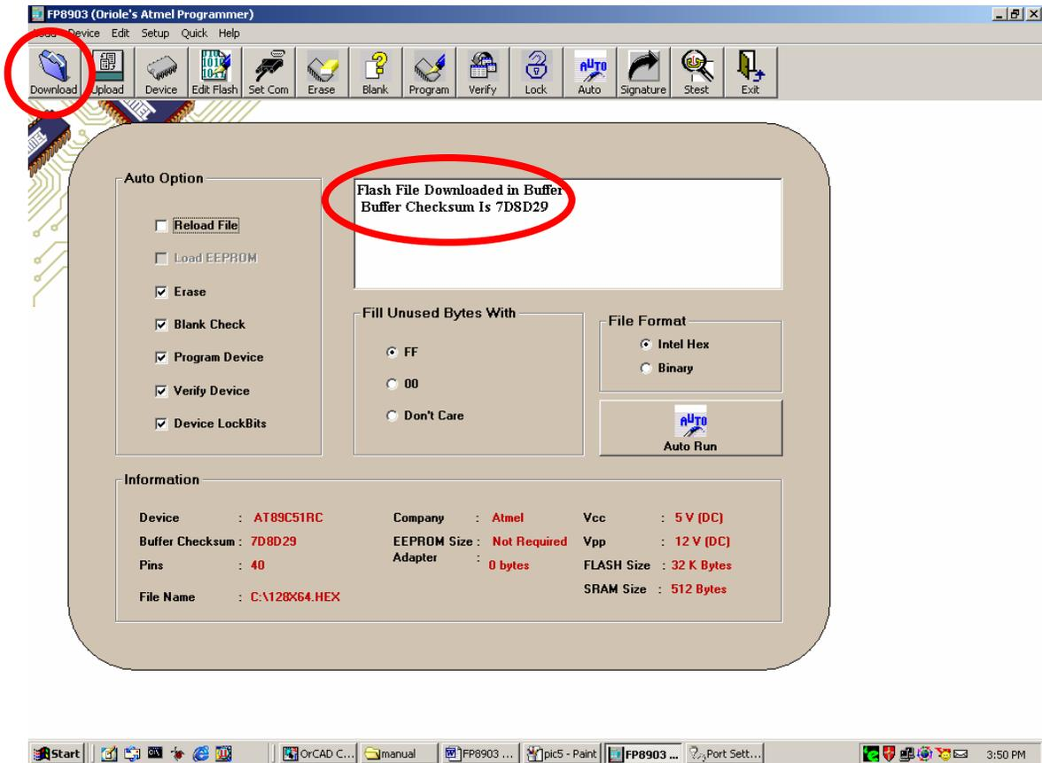
If the device is having the EEPROM along with FLASH, command will ask you for EEPROM file and FLASH file separately, Follow the same procedure to select the file from its location.
