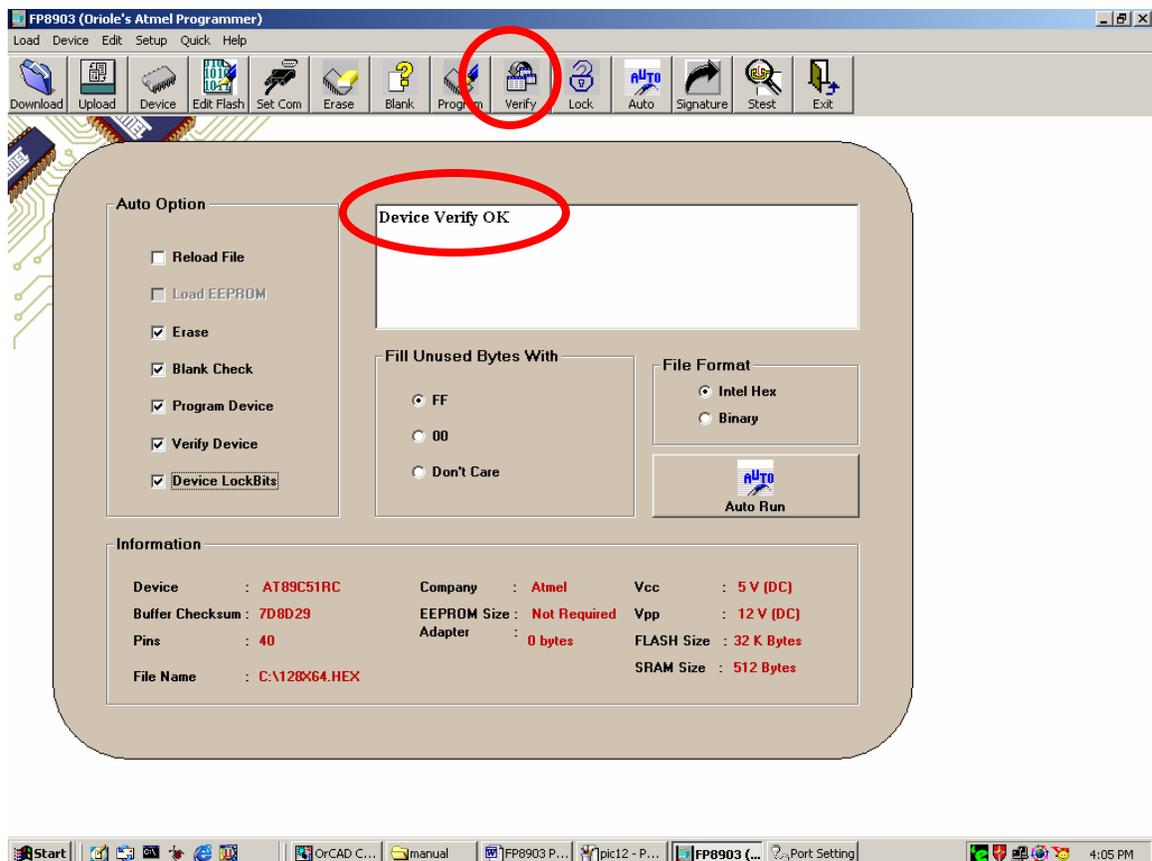
If the command is not executed successfully then the Status Window displays the following error message as
