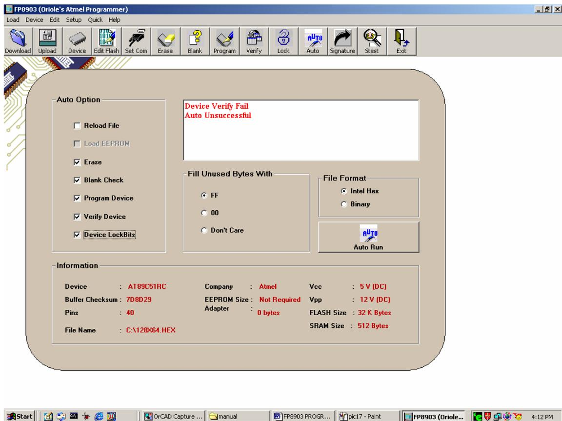
If the “Load EEPROM “ command in the AUTO OPTION window is not checked, then the selected EEPROM file is not loaded in the HEX EDITOR.
