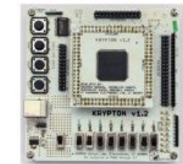
Krypton: Higher-end CPLD board Currently used for IITB lab courses, and provided to IIIT-B, IIT-G, and used in workshops
