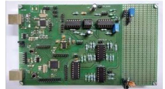
Aurum: PIC microcontroller developer board Currently used for IITB EDL lab course, and used in workshops
