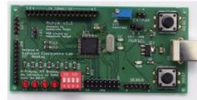
Aurum: PIC microcontroller developer board Currently used for IITB EDL lab course, and used in workshops
