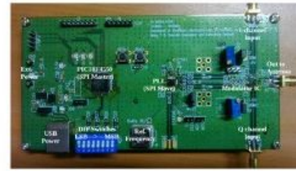
I-Q modulator board: used for IIT Bombay communications lab course
