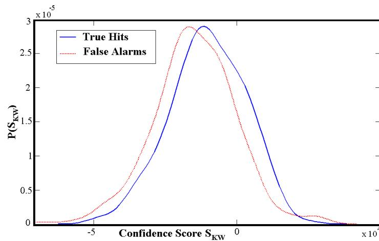
Figure 10: Distribution of confidence score  $S_{KW}$  over true hits and false alarms obtained on the KWS development set. The pdf has been smoothed in Matlab
