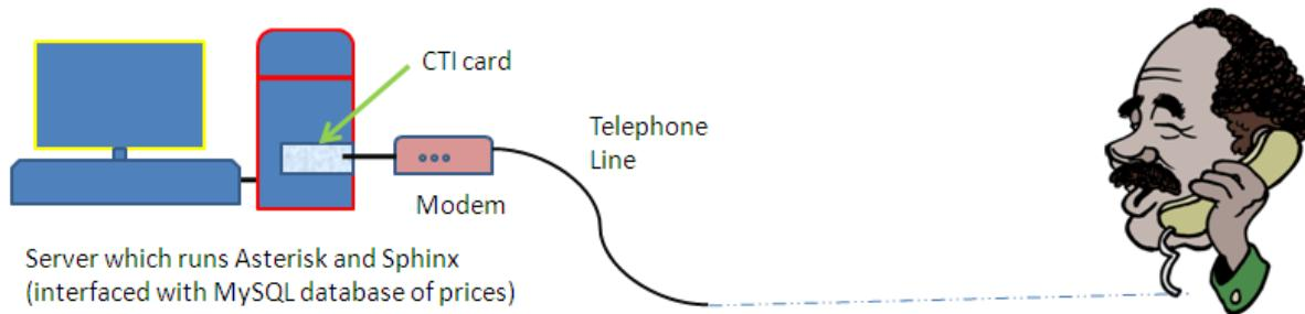
Figure 2: Various hardware and software components of AgroAccess system (Image partially taken from <http://www.clipartmojo.com/>)
