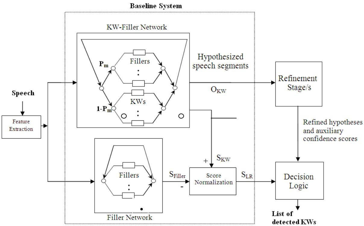
Figure 8: Overall KWS system configuration - the baseline and refinement stages
