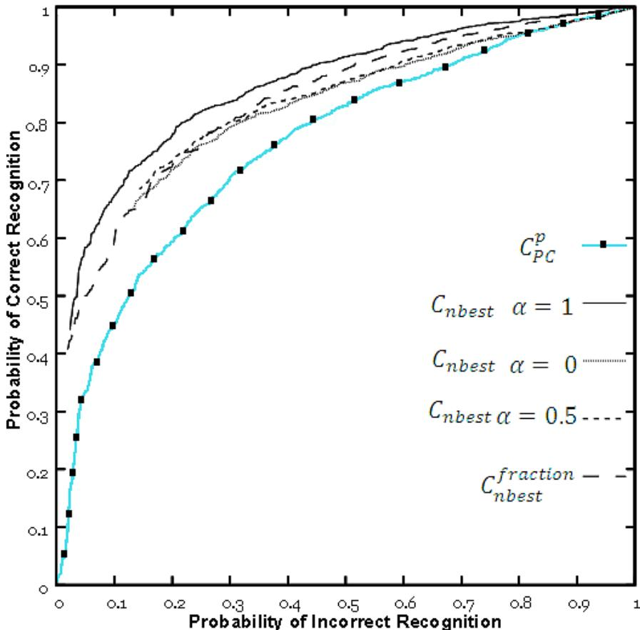
Figure 17: ROC curves for  $C_{nbest}^{fraction}$ ,  $C_{PC}^p$ , and  $C_{nbest}$  (at  $\alpha = 0, \alpha = 0.5$  and  $\alpha = 1$ ) for testing on **283spkrSubset**. Total number of (5 phone) hypothesized words = 3808, total number of correct words = 2768; total number of incorrect words = 1040.
