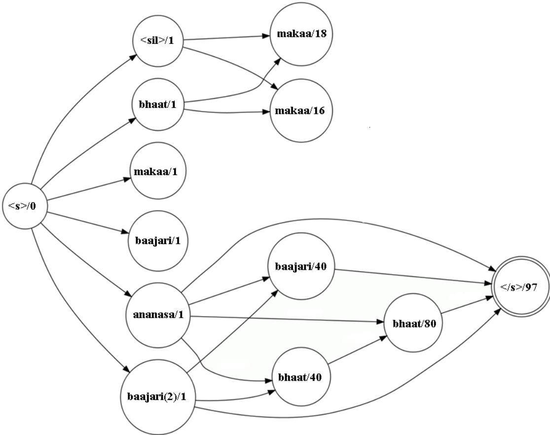
Figure 7: A word lattice created after recognition; in each hypothesis (denoted by a circle) the recognized word and its starting frame are shown;  $<s>$  and  $</s>$  denote start and end of the utterance respectively. Image created by porting the lattice file to GraphViz software.
