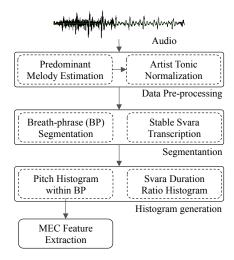
Figure 1. Block diagram for data processing
