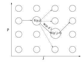
**Fig. 9.** State space representation of dynamic programming. The states and edges are labeled by their costs. The dashed edges indicate the possible transitions for state (p, j) while the solid edges indicate the minimum cost path found by dynamic programming.
