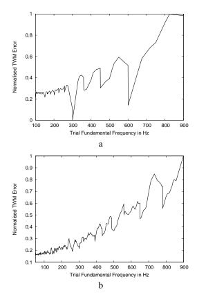
**Fig. 4**. a. TWM Error plot for complex tone of 300 Hz containing harmonics at 600, 900, 1200, 1500, 1800 Hz all having equal amplitude. b. Similar plot for the same complex tone mixed with tabla stroke Na.
