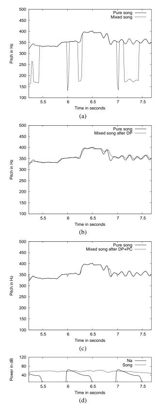
**Fig. 6.** a. Pitch Contours of portion of song (pure and mixed with stroke Na) obtained by TWM based PDA. b. Pitch Contour of same sample after applying DP. c. Pitch Contour of same song after applying pitch correction. d. Power contour of stroke Na and the song.
