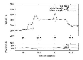
**Fig. 10**. Pitch contours of a portion of song mixed with tabla stroke Na obtained by TDC and TDP. The solid line indicates the pitch contour of pure song obtained by TWM. Lower plot gives power contour of stroke Na and the song
