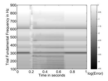
**Fig. 5.** Correlogram of the log of normalized TWM error of a complex tone of 300 Hz as described in Fig. 4.a, mixed with tabla stroke Na. The stroke starts about .2s and lasts for .45s. The darkness of a pixel d(p, t) indicates the log of normalised error for frequency p at time instance t, according to the scale shown on the right. Thus darker the point lower is error.
