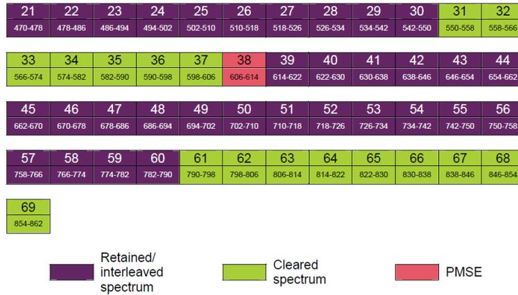
Figure 2.5: UHF Band channels in the UK after Digital Switchover. Adapted from [31]
