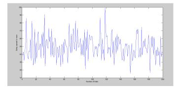
Fig. 2. Delay spread of the channel for several trials
