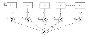
Fig. 1. Tapped delay line model for wideband wireless systems
