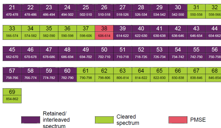
Figure 2.5: UHF Band channels in the UK after Digital Switchover. Adopted from [14]
