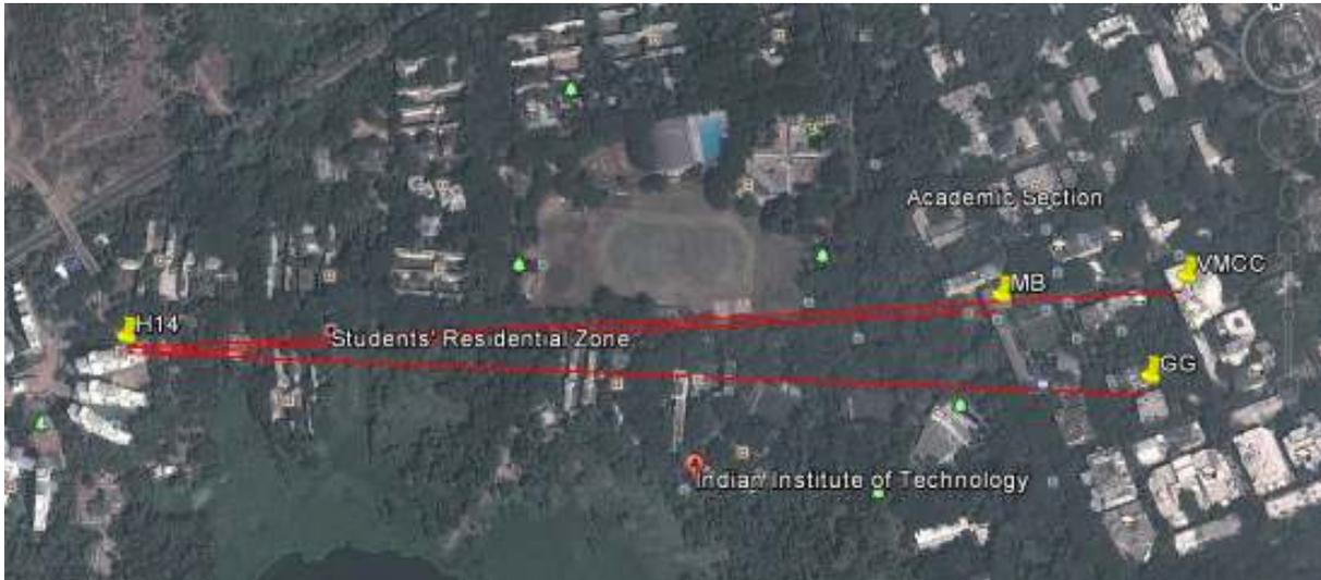
Figure 3: Point to multipoint topology. All non-root nodes (GG, MB and VMCC) connect directly to the root node (H14).
