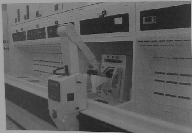
Figure 4-10 A typical cleaning station in a modern IC manufacturing facility. Wet chemical cleaning baths are in the sinks. The robot is loading a cassette of wafers into a spin dryer. Photo courtesy of Ruth Carranza.
