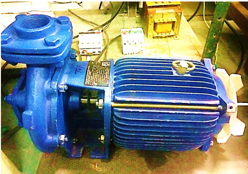
Fabricated BLDC motor integrated with the surface pump
