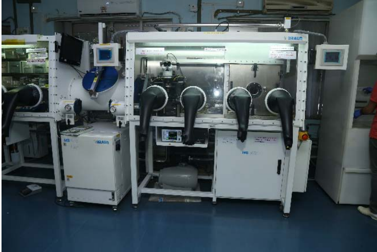
Glove Box integrated with Evaporator and Probe Station
