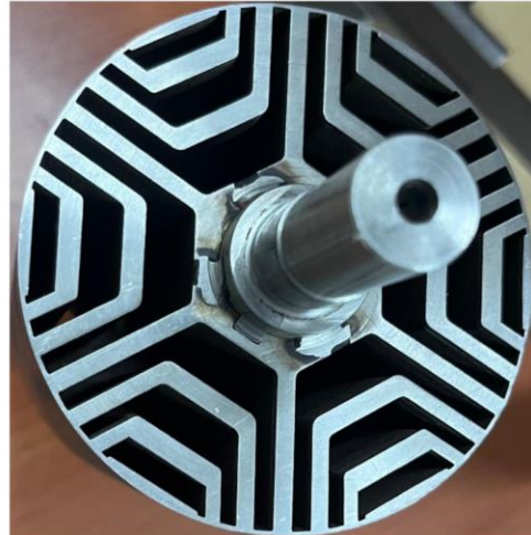
Ferrite IPM-SyRM prototype for electric 2W
