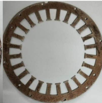
Ferrite IPM-SyRM prototype for electric 3W
