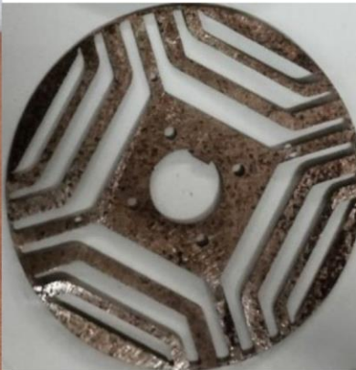
Ferrite IPM-SyRM prototype for electric 3W
