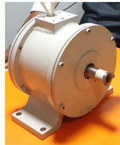
Fig. FEM model, stator, rotor and the final assembly of the manufactured prototype.
