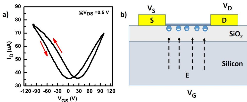
Figure 7.2.1: Hysteresis behavior of exfoliated GFET fabricated using e-beam lithography; (a)Hysteresis in transfer curve, (b)charge screening mechanism in GFETs.
