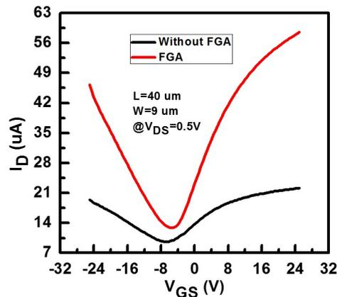
Figure 7.4.3: Comparison of transfer char. of devices fabricated using  $\text{SiO}_2$  with and without FGA
