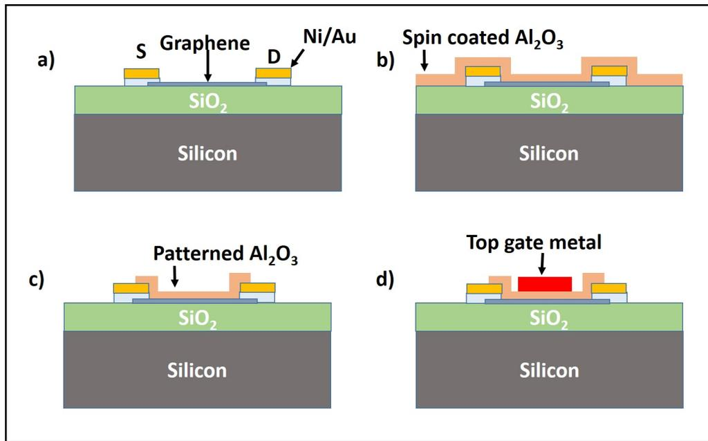
Figure 6.2.1: Fabrication steps for top-gated GFETs; a) Back-gated device, b) Conformal dielectric deposition using spin coating technique, c) Dielectric patterning, d) Top gate metal deposition.
