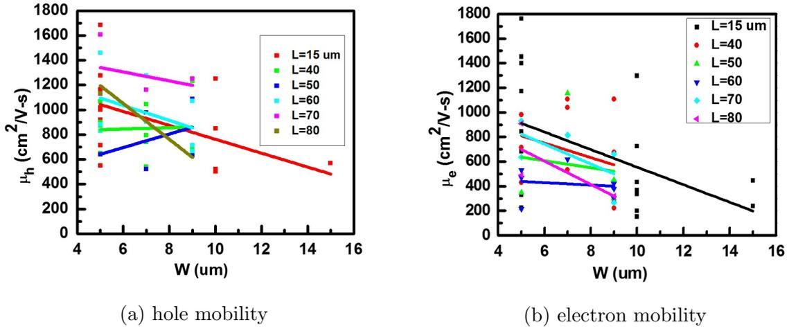
Figure 6.4.1: Dependence of carrier mobility on dimensions of graphene.
