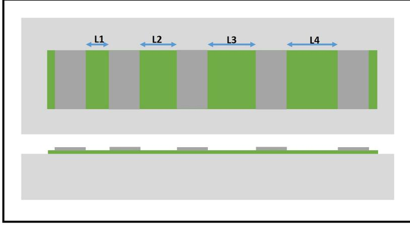
Figure 4.1.2: Typical TLM measurement structure
