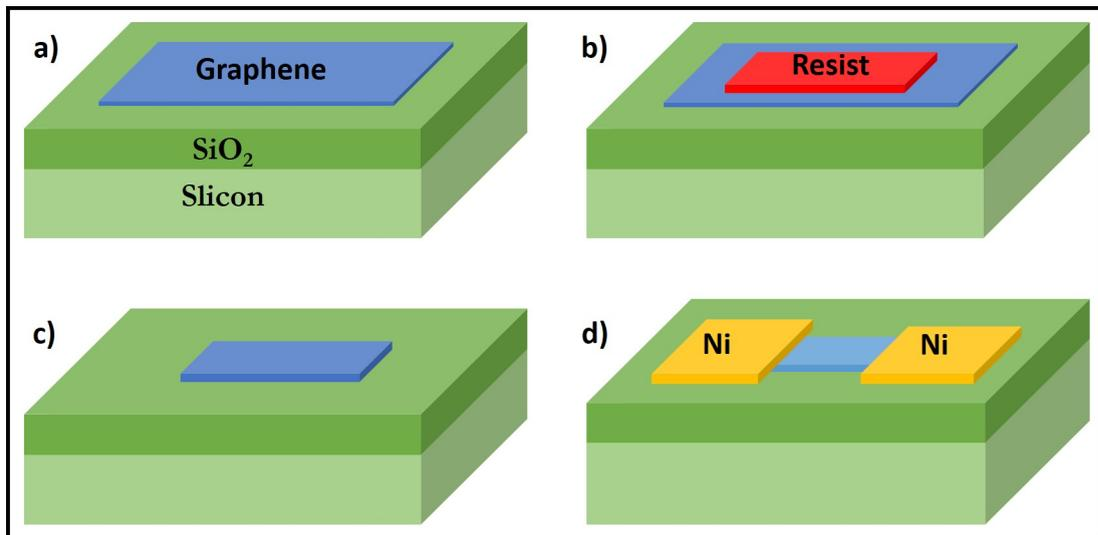
Figure 6.1.1: CVD GFET fabrication process; a) Graphene transfer on  $SiO_2$ , b) Graphene patterning lithography, c) Patterned graphene, d) device structure after metal deposition and lift-off.
