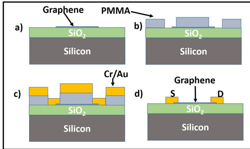
Figure 5.1.1: GFET fabrication steps; a) graphene transfer, b) resist patterning, c) metal deposition, d) Fabricated device after lift-off.
