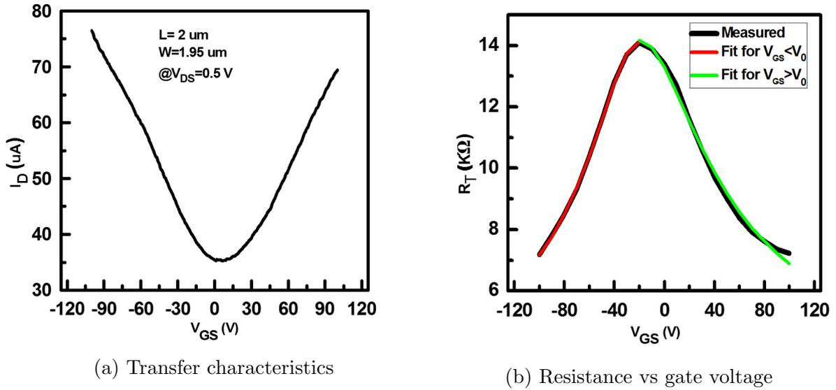
Figure 5.2.4: Electrical characteristics of GFET.
