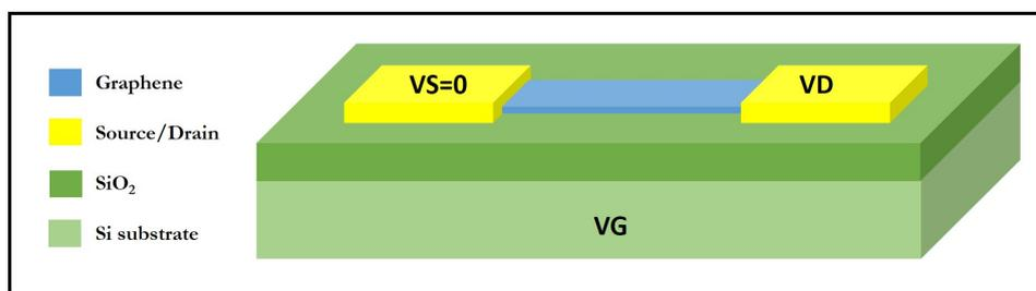
Figure 3.1.1: Structure of back-gated GFET.
