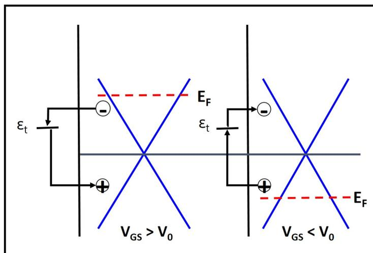
Figure 7.4.2: Mechanism of charge trapping and de-trapping depending on position of fermi level with respect to interface trap state.
