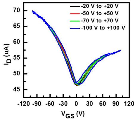
Figure 7.2.2: Shift in Dirac point of voltage of exfoliated GFET with gate voltage sweep range.
