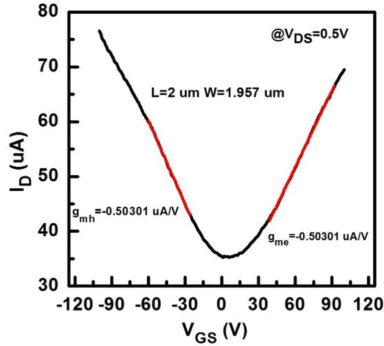
Figure 4.2.1: Illustrative example to find transconductance from transfer characteristics.
