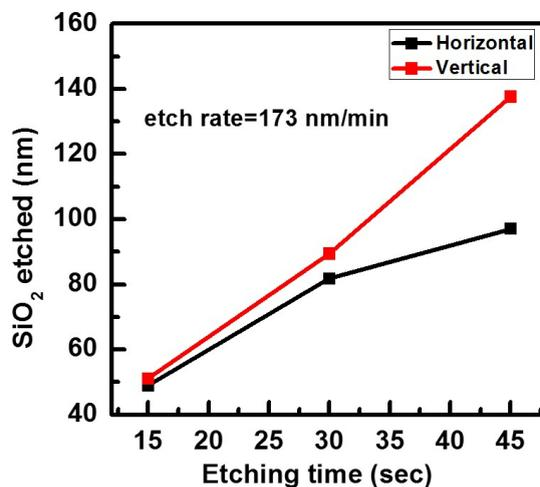
Figure 6.1.2: Comparison of SiO<sub>2</sub> etching in horizontal and vertical position using 5:1 BHF
