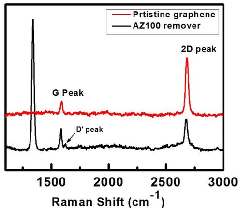
Figure 7.1.4: Raman spectrum of pristine CVD graphene, AZ5214E spin coated and removed using AZ 100 remover and graphene treated with AZ 100 remover.
