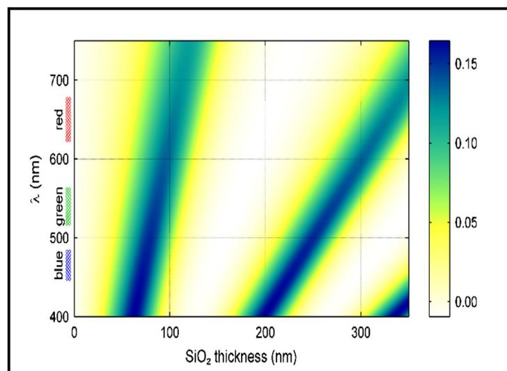
Figure 5.1.3: Contrast of graphene as function of  $SiO_2$  thickness and wavelength of light.
