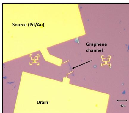
Figure 5.1.4: Optical image of fabricated device showing source, drain and graphene channel.
