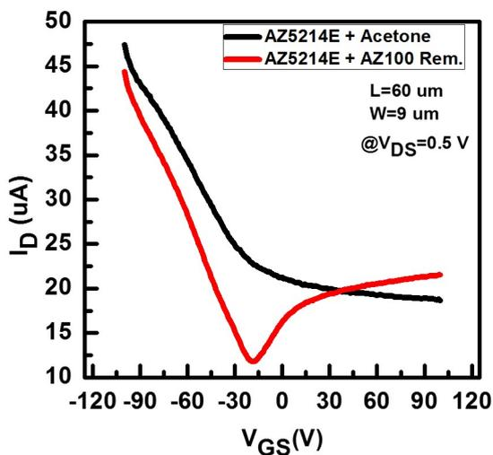
Figure 6.3.3: Comparison of AZ5214E resist removal using Acetone and AZ 100 remover.
