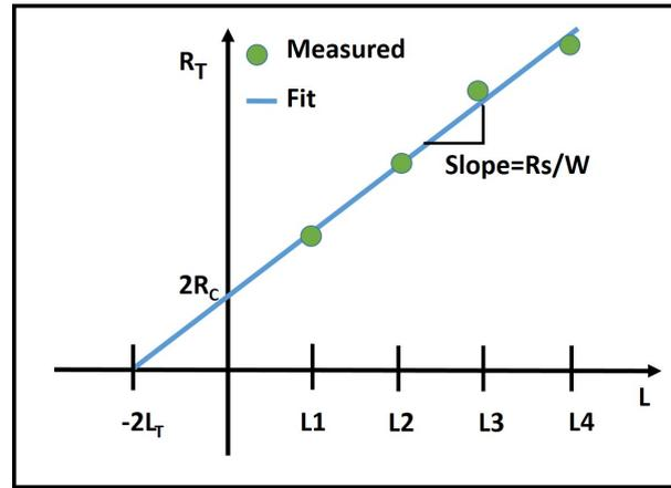
Figure 4.1.1: Fitting of total resistance equation to measured data.
