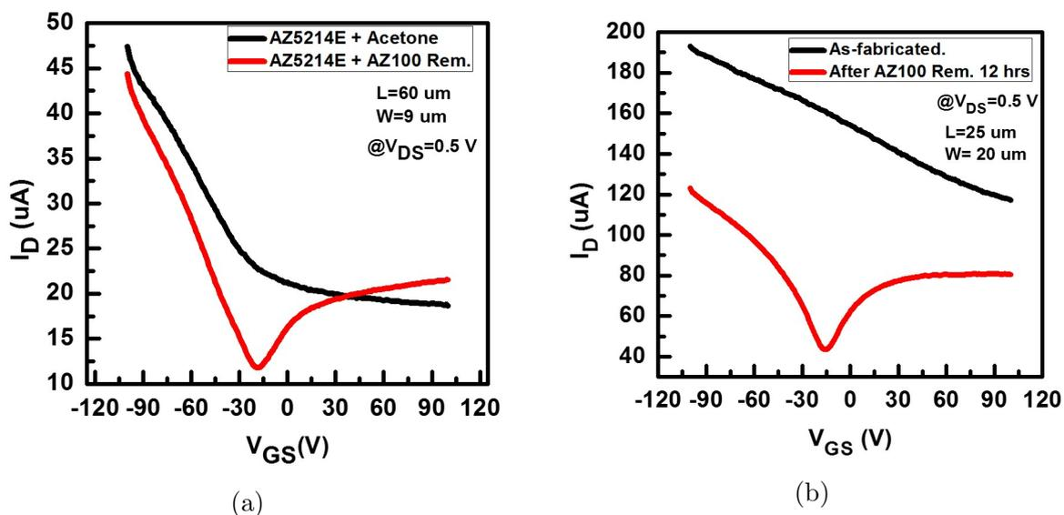
Figure 7.1.3: Effect of treating CVD graphene with AZ 100 remover; (a) devices fabricated using AZ5214E resist, acetone and AZ 100 remover used for stripping resist, (b) Devices fabricated using PMMA resist and treated with AZ 100 remover for 12 hours.
