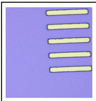
Figure 6.1.3: Optical image of patterned resist on top of graphene.
