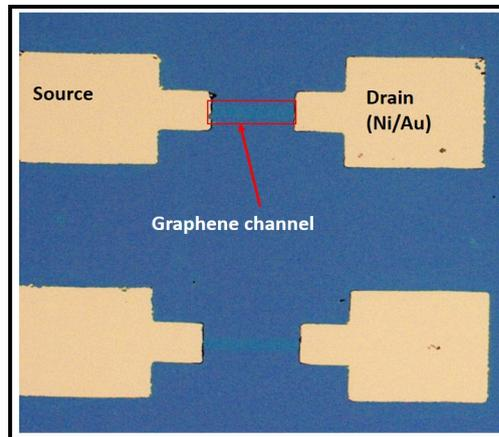
Figure 6.1.4: Optical image of fabricated CVD GFETs showing source, drain and patterned graphene channel.
