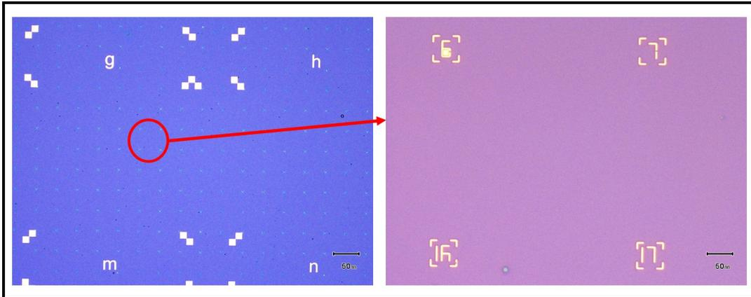
Figure 5.1.2: Optical image of marker used to identify graphene flakes for electrode design.
