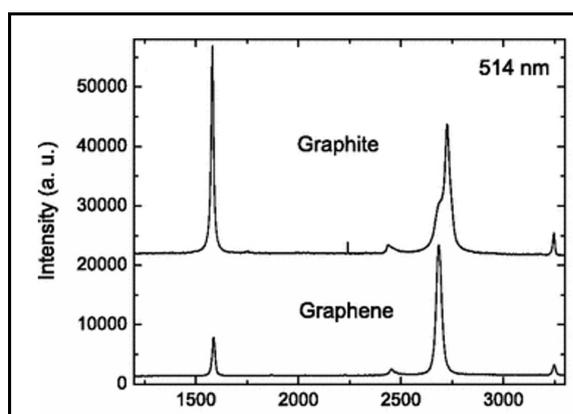
Figure 5.2.1: Raman spectrum of graphite and single layer graphene.
