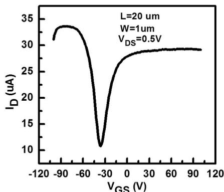
Figure 6.3.5: Transfer characteristics of highest mobility device fabricated using CVD graphene and e-beam lithography. Treated with AZ 100 remover for 12 hours.
