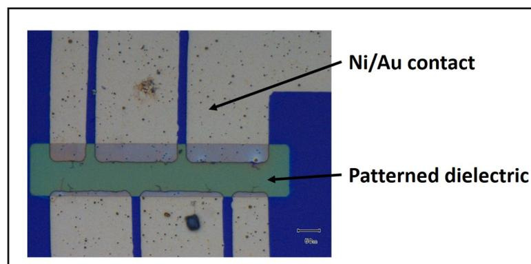
Figure 6.2.2: Optical image of patterned top gate dielectric.
