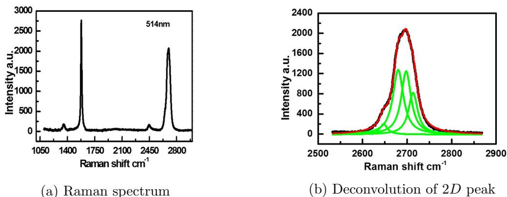
Figure 5.2.3: Raman spectrum of bilayer graphene and deconvolution of 2D peak.
