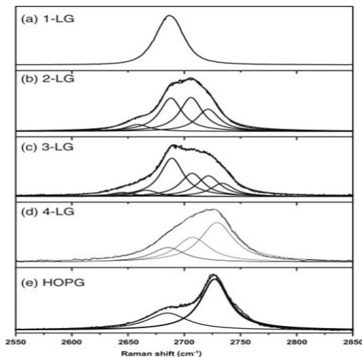
Figure 5.2.2: Number of layer identification using deconvolution of 2D peak
