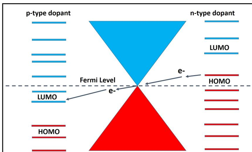
Figure 7.1.1: Mechanism of chemical doping by charge transfer due to surface adsorbates.
