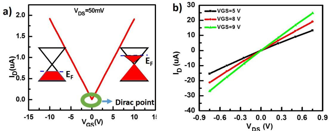
Figure 3.3.1: Simulated current-voltage char. of GFETs; a) Transfer, b) Output.
