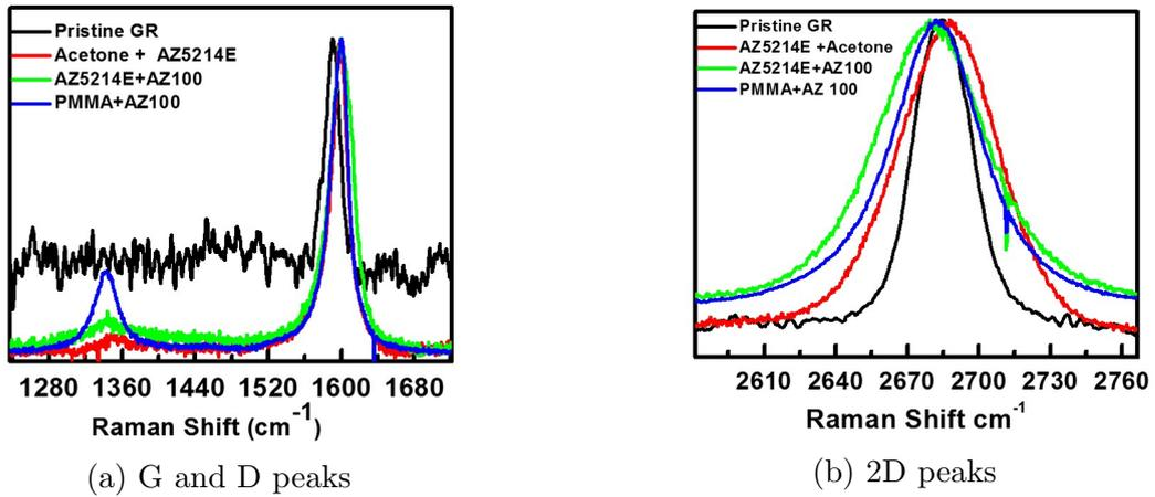
Figure 7.1.5: Comparison of shift in G and 2D peaks of Raman spectrum of fabricated devices. Devices fabricated using CVD graphene, AZ5214E and PMMA resists, resist removal using acetone and AZ 100 remover.
