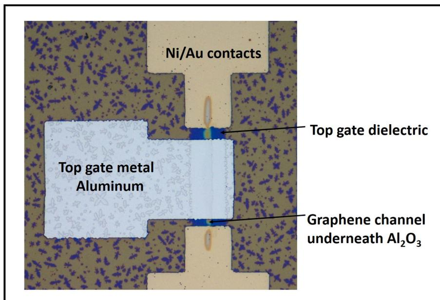
Figure 6.2.3: Optical image of top-gate GFET after metal deposition.
