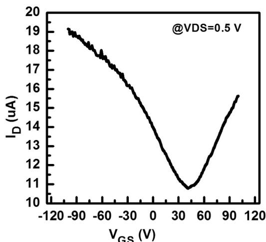
Figure 7.1.2: Shift in Dirac point of p-doped as-fabricated device due to unintentional doping. Devices were fabricated using exfoliated graphene and e-beam lithography.
