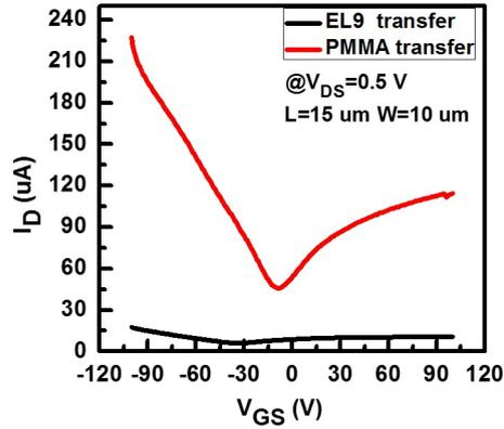
Figure 6.3.2: Comparison of graphene transfer using PMMA and EL9. Devices are fabricated using AZ5214E resist and optical lithography.
