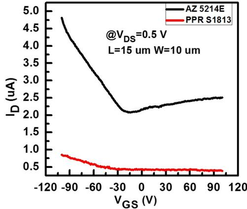
Figure 6.3.1: Comparison of CVD GFETs fabricated using S1813 and AZ5214E photoresist and graphene transfer using EL9 copolymer.
