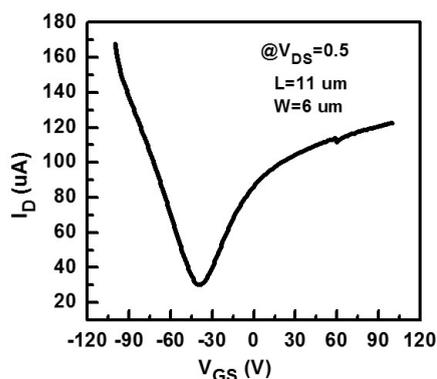
Figure 7.3.1: Asymmetry observed in transfer characteristics of CVD GFETs because of p-doping from Nickel contacts. Devices are fabricated using CVD graphene and optical lithography.
