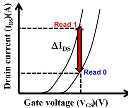
FIGURE 2.12: State ‘1’ and state ‘0’ are differentiated by two different threshold voltages in the transfer characteristics of the device [58].  $V_{GS}$  and  $I_{DS}$  are the gate to source voltage and drain to source current respectively.  $\Delta I_{DS}$  is the drain current difference between read state ‘1’ and read state ‘0’.
