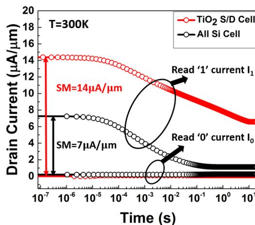
FIGURE 3.9: Comparison of the transient characteristics of  $\text{TiO}_2$  S/D cell and all-Si Z-RAM cell at  $T = 300\text{ K}$ .
