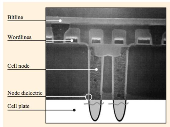
FIGURE 2.5: SEM photomicrograph of  $0.25\text{-}\mu\text{m}$  trench DRAM cell suitable for scaling to  $0.15\ \mu\text{m}$  and below. Figure taken from reference [12].
