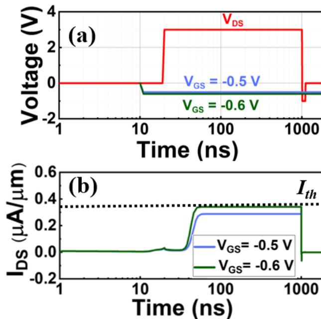
FIGURE 5.15: (a-b) Output drain current does not make any spike as long as  $V_{in} \leq V_{th} = 0.6 V$ . Drain current is taken for  $V_{in} = 0.5$  and  $0.6 V$  and it saturate before reaching  $I_{th}$ .
