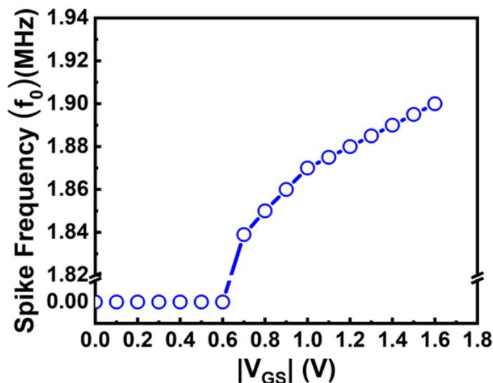
FIGURE 5.17: Spiking frequency ( $f_0$ ) versus input ( $|V_{GS}|$ ) shows that, for  $V_{in} \leq V_{th} = 0.6$  V, the frequency is zero while for  $V_{in} \geq V_{th}$ ,  $f_0$  increases with input bias.
