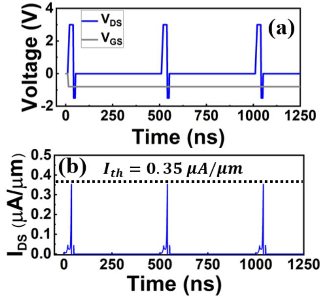
FIGURE 5.16: (a-b) Biasing scheme for neuron firing and reset of the proposed neuron. For  $V_{in} = 0.8 V$ , when  $I_{DS}$  reaches  $I_{th} = 0.35 \mu A/\mu m$ ,  $V_{DS}$  is reset by the reset circuit and a spike is generated.
