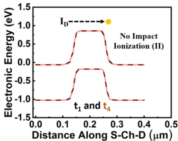
FIGURE 5.11: Energy band diagram of the proposed device along source-channel-drain at  $t = t_1$  and  $t_4$  i.e., for initial and reset conditions.
