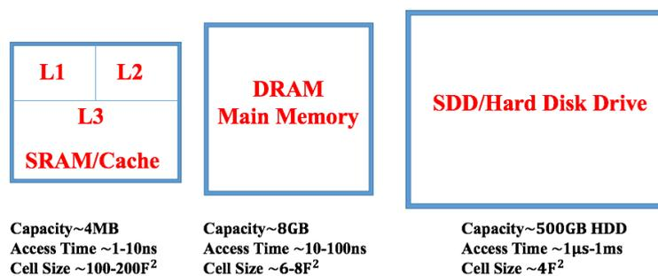
FIGURE 2.1: Semiconductor memory architecture.
