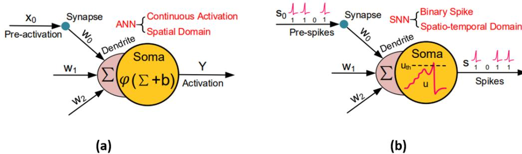
FIGURE 2.21: (a) Basic neuron model in ANNs. (b) Basic neuron model in SNNs. The figures are taken from reference [95].
