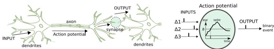
FIGURE 2.20: Biological neuron and its association with an artificial spiking neuron [93].
