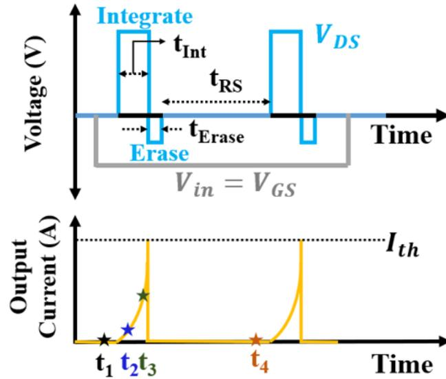
FIGURE 5.10: Schematics of the biasing mechanism for LIF functionality and corresponding output current  $I_{out}$ .
