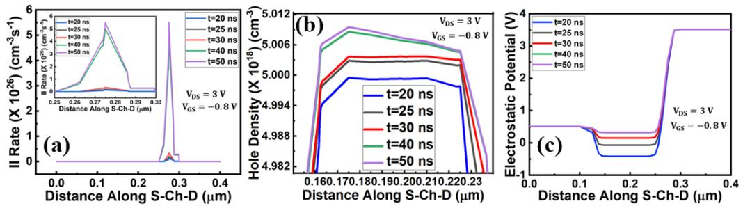
FIGURE 5.14: (a) Impact ionization (II) rate is plotted along source-channel-drain for different time. Inset is the zoomed figure. (b) Hole density is plotted along source-channel-drain for different time. (c) Variation of electrostatic potential along source-channel-drain for different time. The time reference is the same as in Fig. 5.13.
