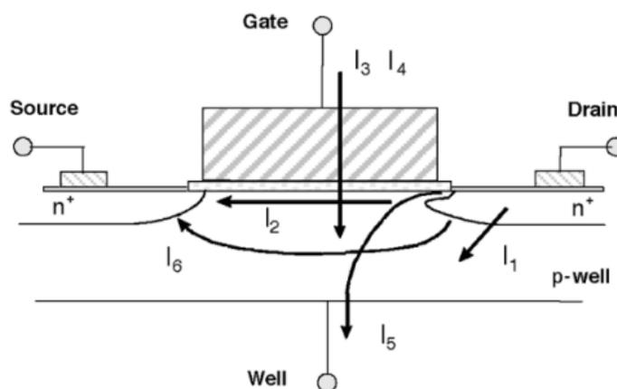
FIGURE 2.7: Summary of leakage current mechanisms of deep sub-micrometer transistors. Figure is taken from reference [16].
