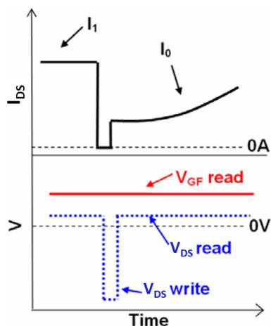
FIGURE 2.16: The drain and front gate biasing sequences and schematics for both the write/read state ‘0’ for forward bias based erasing.  $V_{DS}$  and  $V_{GF}$  are the drain to source voltage and front gate voltage respectively.  $I_1$  and  $I_0$  are the read state ‘1’ and read state ‘0’ currents respectively. This image is taken from reference [59].
