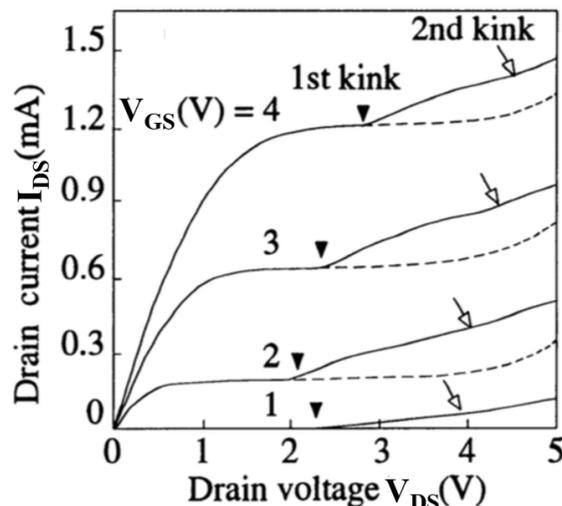
FIGURE 2.9: Experimental drain current ( $I_{DS}$ ) versus drain voltage ( $V_{DS}$ ) characteristics in SOI MOSFETs showing kink effect (solid line), which may be cancelled by grounding the body (dotted line). Figure taken from reference [43].
