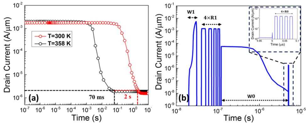
FIGURE 4.12: (a) Variation of read ‘1’ current as a function of time at both  $T = 300 \text{ K}$  and  $T = 358 \text{ K}$  respectively. (b) Multiple reading operation of the proposed cell at  $T = 300 \text{ K}$ . This shows the non-destructive read-out mechanism in the proposed Z-RAM cell.
