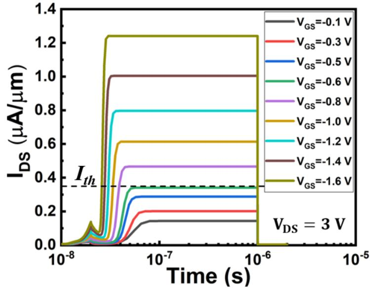
FIGURE 5.13: Transient simulation shows the  $I_{DS} - Time$  characteristics under different  $V_{in}$ . The  $I_{th}$  is set at  $0.35 \mu A/\mu m$ .
