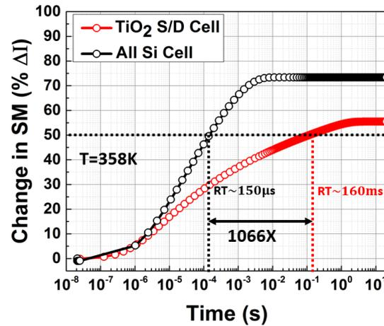
FIGURE 3.12: Comparison of the change in sense margin as a function of time between TiO<sub>2</sub> source/drain cell and all-Si cell at  $T = 358K$ .
