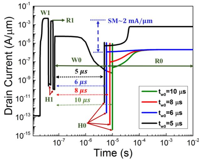
FIGURE 4.10: Drain current transients in the sequence of operation with the given biasing scheme under different write '0' time ( $t_{w0}$ ): Write '1':  $V_{GS} = 0$  V,  $V_{DS} = 0.8$  V. Hold:  $V_{GS} = -0.8$  V,  $V_{DS} = 0$  V Read:  $V_{GS} = -0.8$  V,  $V_{DS} = 0.5$  V.
