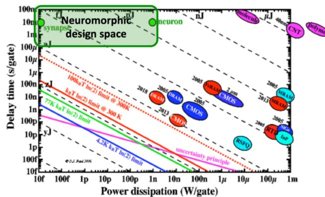
FIGURE 2.19: Delay time per transistor versus the power dissipation plot. The operating regime for neuromorphic devices is in the upper left corner indicating the extremely low power dissipation of biological synapses and the corresponding delay time. Systems built in this region would be more “brain-like” in their power and cycle times. The image is taken from reference [73].
