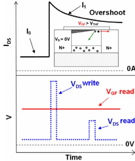
FIGURE 2.13: The front gate and drain biasing sequences and schematics for both the write/read state ‘1’ programming by impact ionization.  $V_{DS}$  and  $V_{GF}$  are the drain to source voltage and front gate voltage respectively.  $V_{THF}$  is the front channel threshold voltage.  $I_1$  and  $I_0$  are the read state ‘1’ and read state ‘0’ currents respectively. The image is taken from reference [59].
