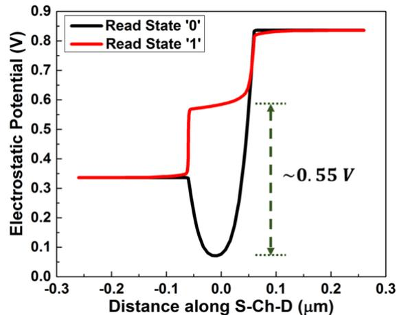
FIGURE 3.8: Electrostatic potential at the body of the  $\text{TiO}_2$  S/D cell during read '1' and read '0'.
