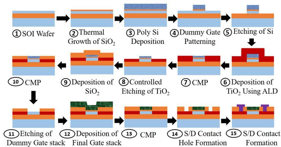
FIGURE 4.14: Proposed fabrication process flow of the  $\text{TiO}_2$  S/D Z-RAM Cell.
