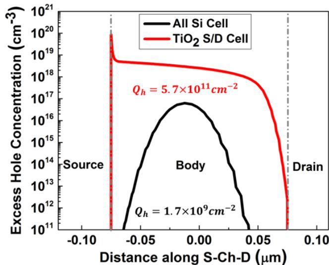
FIGURE 3.7: Comparison of the excess hole concentration between  $\text{TiO}_2$  S/D cell and all-Si cell at time  $t = 25 \text{ ns}$  i.e.,  $4 \text{ ns}$  after the read '1' operation starts (time reference is shown in Fig. 3.6).  $Q_h$  is the excess hole density in the body, obtained by integrating the hole concentration in the body.
