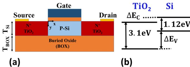
FIGURE 4.1: (a) Schematic of the proposed  $\text{TiO}_2$  source/drain FD-SOI Z-RAM cell. (b)  $\text{TiO}_2$  and Si band line up.  $\Delta E_C \approx 0.05 eV$  and  $\Delta E_V \approx 2 eV$  [126].
