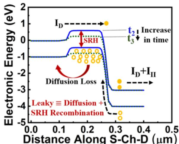
FIGURE 5.12: Energy band diagram of the proposed device along source-channel-drain at  $t = t_2$  and  $t_3$  which describes charge integration and leak phenomena.
