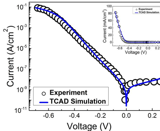
FIGURE 3.3: Comparison of simulated diode characteristics for n-TiO<sub>2</sub> - p-Si heterostructure diode with published result [126], demonstrating the calibration of the simulation models used.
