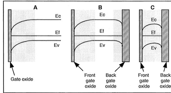
FIGURE 2.11: Energy band diagrams in (a) bulk, (b) partially depleted SOI and (c) fully depleted SOI. All devices are represented at threshold (front gate voltage = threshold voltage). The shaded areas represent the depleted zones. SOI devices are represented for a condition of weak inversion (below threshold) at the back interface [57].  $E_C$ ,  $E_V$ , and  $E_i$  are the conduction band energy, valence band energy and Fermi energy levels respectively.
