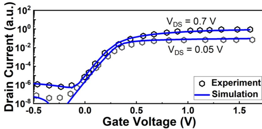
FIGURE 5.6: Comparison of simulated  $I_{DS} - V_{GS}$  characteristics with experimental data [151], demonstrating the calibration of the simulation models used.
