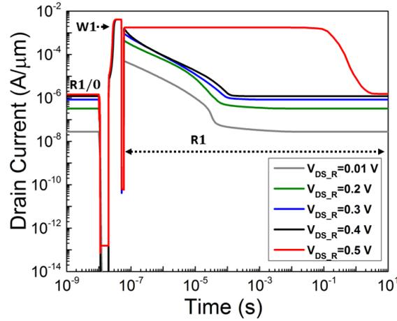
FIGURE 4.9: Optimization of  $V_{DS}$  for reading operation.  $V_{GS}$  is kept fixed at  $-0.8$  V.
