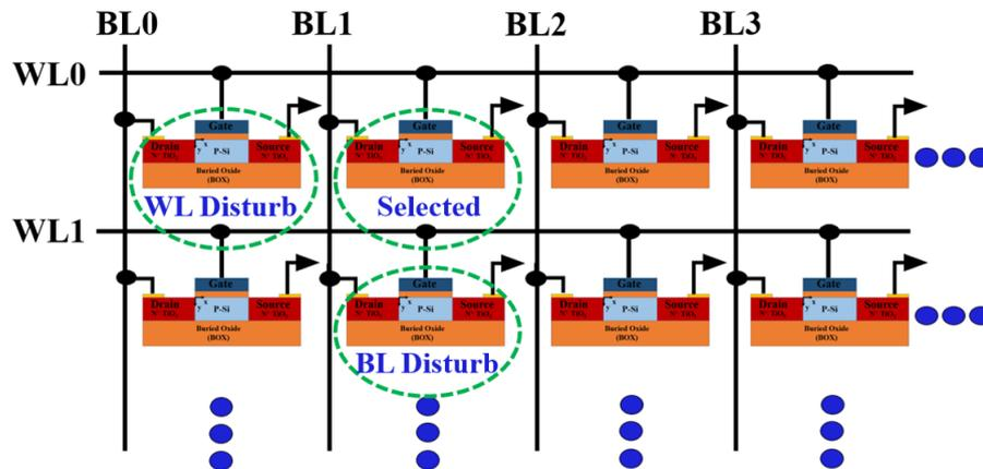
FIGURE 4.13:  $TiO_2$  S/D Z-RAM cell array and disturbances among neighbouring cells.
