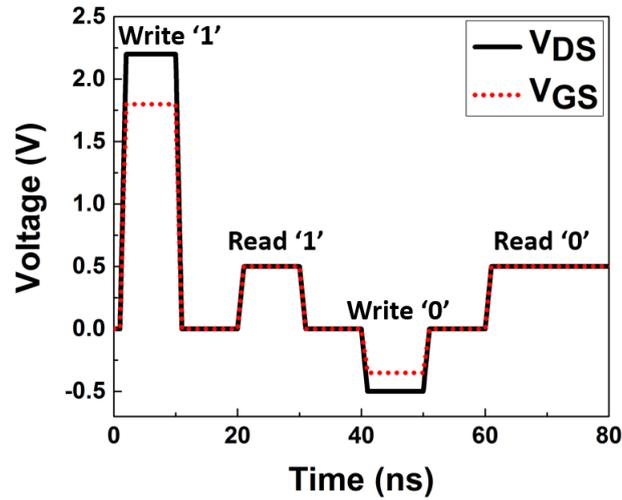
FIGURE 3.6: Biasing scheme for both  $\text{TiO}_2$  source/drain and all-Si Z-RAM cell. Time in the x-axis is shown for reference.
