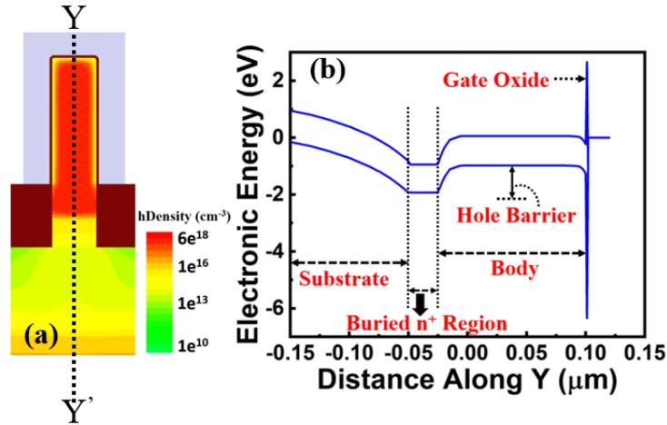
FIGURE 5.7: (a) Simulated contour plot of excess hole density at the body along  $c1$ . Corresponding biases are  $V_{DS} = 2\text{ V}$  and  $V_{GS} = -1\text{ V}$ . (b) Energy band diagram along  $YY'$ . Buried  $n^+$  layer, creates a barrier for excess majority carriers at the body.
