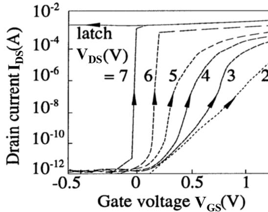
FIGURE 2.8: Experimental drain current ( $I_{DS}$ ) versus gate voltage ( $V_{GS}$ ) characteristics in SOI MOSFETs illustrating the sub-threshold slope steepening and the single transistor latch. Figure taken from reference [44].
