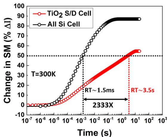
FIGURE 3.10: Comparison of the change in sense margin as a function of time between  $TiO_2$  source/drain cell and all-Si cell at  $T = 300K$ .
