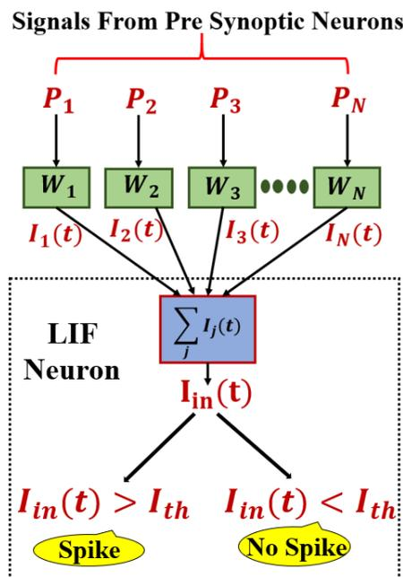
FIGURE 5.3: Schematic representation of a spiking neural network (SNN) with several pre-synaptic neurons and one post synaptic LIF neuron. Weighted signals are coming from pre-synaptic neurons through synapse and integrated in the LIF neuron. The algorithm for SNN is taken from reference [150].
