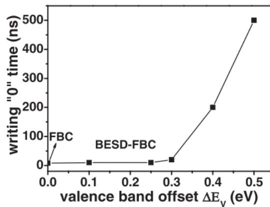
FIGURE 4.11: Writing '0' time dependence of valence band offset ( $\Delta E_V$ ).  $\Delta E_V = 0$  eV means normal floating body cell (FBC). The writing time increase dramatically for band-gap engineered source/drain FBC when  $\Delta E_V > 0.3$  eV [67].
