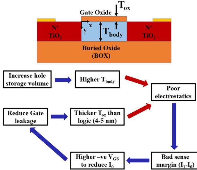
FIGURE 4.2: Design constraints of the transistor parameter for zero capacitor random access memory (Z-RAM) cell.
