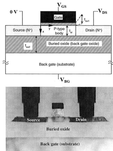
FIGURE 2.10: Schematic cross section of an n-channel SOI MOSFET.  $V_{GS}$ ,  $V_{DS}$ , and  $V_{BG}$  represent the gate to source voltage and drain to source voltage, and back gate voltage.  $t_{si}$ ,  $t_{ox1}$ , and  $t_{ox2}$  are the silicon body thickness, gate oxide thickness and buried oxide thickness respectively. Bottom is the SEM cross-section image of an actual SOI MOSFET [56].
