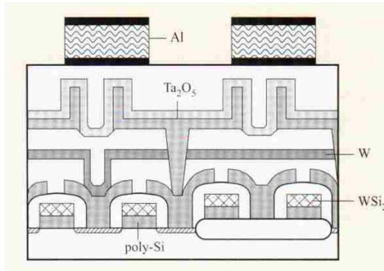
FIGURE 2.6: Schematic cross section of stacked capacitor cell suitable for  $0.15 \mu\text{m}$ .
