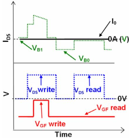
FIGURE 2.17: The drain and front gate biasing sequences and schematics for both the write/read state ‘0’ for capacitive coupling based erasing.  $V_{DS}$  and  $V_{GF}$  are the drain to source voltage and front gate voltage respectively.  $I_1$  and  $I_0$  are the read state ‘1’ and read state ‘0’ currents respectively.  $V_{B0}$  and  $V_{B1}$  are the body potential during read state ‘1’ and read state ‘0’. This image is taken from reference [59].
