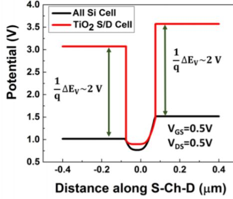
FIGURE 3.5: Comparison of the simulated potential between  $\text{TiO}_2$  S/D cell and all-Si cell under read ‘1’ condition.
