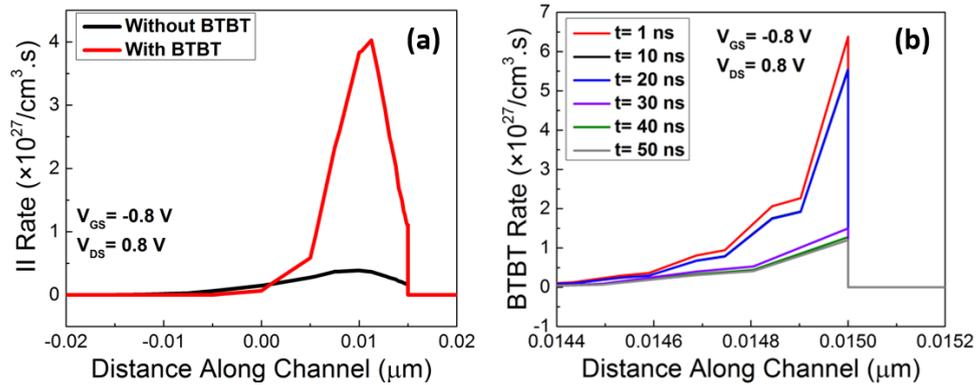
FIGURE 4.5: (a) Impact ionization rate at the drain junction with and without BTBT (taken at  $t = 1 \text{ s}$ ). (b) BTBT rate taken at different time at the drain-channel junction ( $1 \text{ nm}$  below the gate oxide-body interface).
