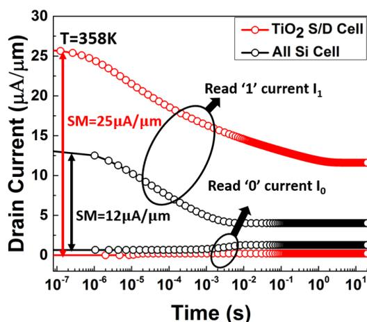
FIGURE 3.11: Comparison of the transient characteristics of  $TiO_2$  S/D cell and all-Si Z-RAM cell at  $T = 358K$ .
