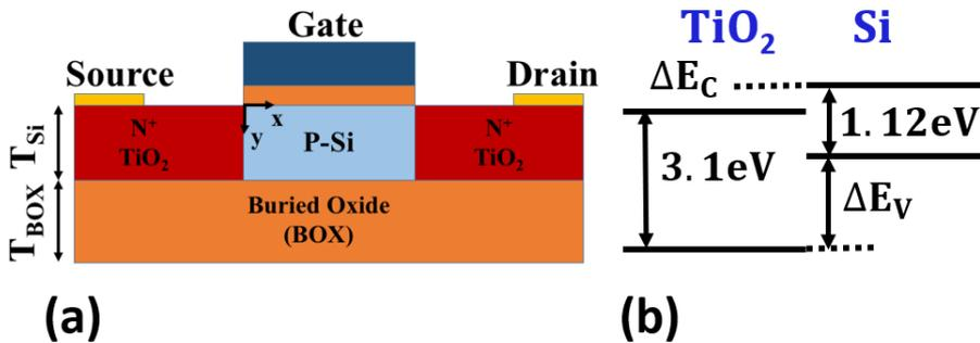
FIGURE 3.1: (a) Schematic of the proposed  $TiO_2$  source/drain Z-RAM cell. (b)  $TiO_2$  and Si band line up.  $\Delta E_C \approx 0.05 eV$  and  $\Delta E_V \approx 2 eV$  [126].
