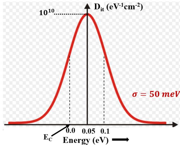
FIGURE 3.4: Gaussian distribution of interface trap density ( $D_{it}$ ) with a maximum value of  $10^{10} eV^{-1} cm^{-2}$ , energetically located at  $50 meV$  (mean position) below the conduction band and with a standard deviation of  $50 meV$ .
