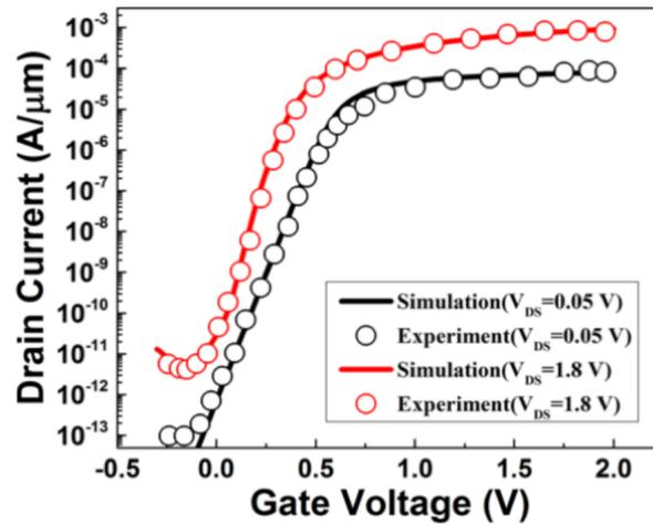
FIGURE 3.2: Comparison of simulated drain current ( $I_{DS}$ ) vs. gate voltage ( $V_{GS}$ ) characteristics of an all Si n-channel PD-SOI MOSFET with published result [133], demonstrating the calibration of the simulation models used.
