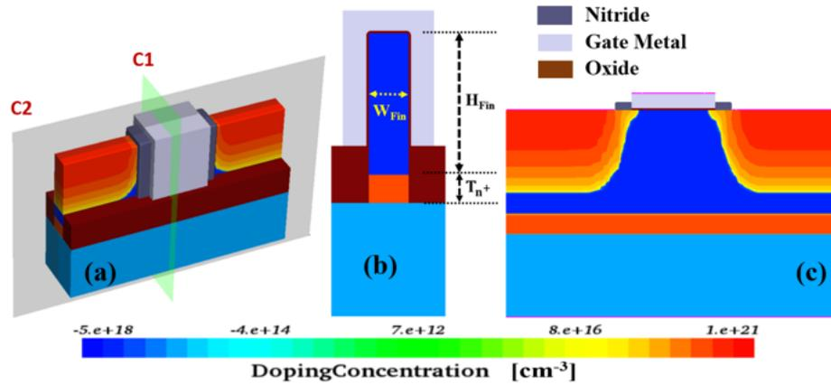
FIGURE 5.5: (a) Simulated bulk FinFET with  $n^+$  buried layer. (b) 2D structure along  $c1$ . (c) 2D structure along  $c2$ . Gaussian doping profile with a peak concentration of  $10^{21} \text{ cm}^{-3}$  is used at source/drain and the channel is uniformly doped. Doping gradient along source/drain to channel is kept at  $2 \text{ nm/decade}$ . The +ve (-ve) sign indicates n-type (p-type) doping.
