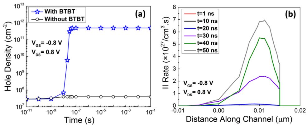
FIGURE 4.6: (a) Hole density ( $20 \text{ nm}$  below the gate oxide-body interface) as a function of time at  $V_{GS} = -0.8 V$  and  $V_{DS} = 0.8 V$  with and without BTBT. (b) Impact ionization rate at the drain-channel junction taken at different time instances.
