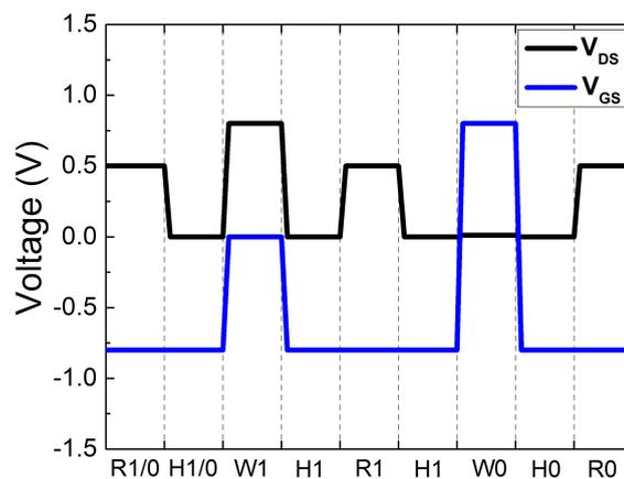
FIGURE 4.7: Biasing scheme for the proposed  $\text{TiO}_2$  source/drain Z-RAM cell. ‘W’, ‘R’ and ‘H’ stands for ‘Write’, ‘Read’ and ‘Hold’.
