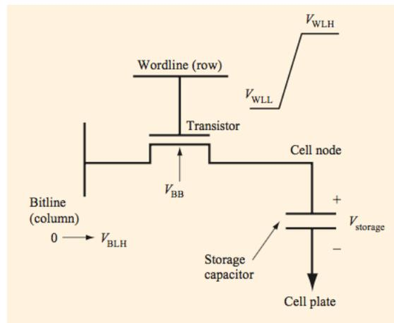
FIGURE 2.4: Conventional one transistor one capacitor DRAM Cell. Each cell consists of one transistor as a switch and a capacitor as storage node.  $V_{BL,H}$ ,  $V_{WL,H}$ ,  $V_{WLL}$ ,  $V_{BB}$  are the bit-line high voltage, word-line high voltage, word-line low voltage, and body supply respectively.  $V_{storage}$  is the voltage across the storage capacitor. This schematic is taken from reference [12].
