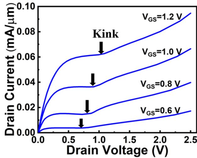
FIGURE 5.8: Kink arises in the output characteristics of the proposed device. This is a signature of hole storage at the body of the transistor.
