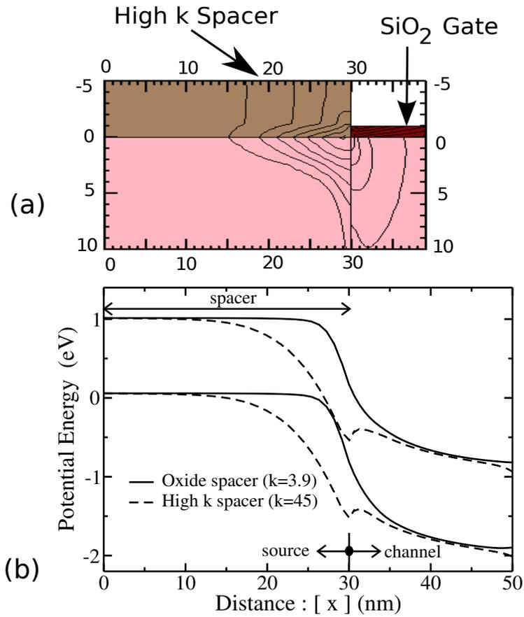
Figure 4.15: (a) Fringe field coupling through spacer (dimensions are in nanometers) and (b) band diagram for nTFET with high- $k$  ( $k = 45$ ) spacer of 30 nm width.  $V_{GS} = 1$  V and  $V_{DS} = 1$  V.
