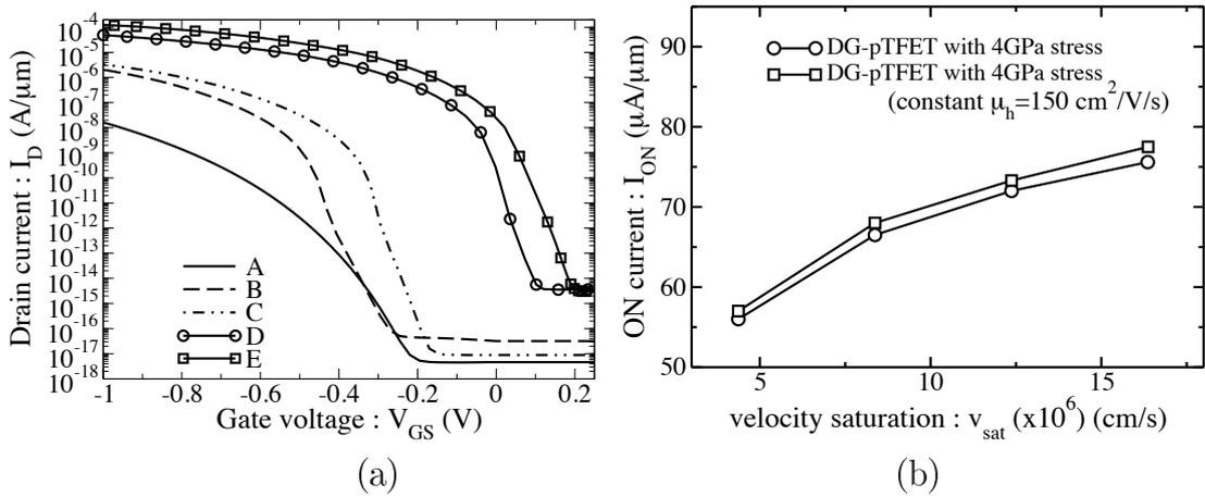
Figure 8.11: (a) The  $I_D$ - $V_{GS}$  characteristics for different technology boosters. (A) non-underlap pTFET with SiO<sub>2</sub> spacer; (B) non-underlap pTFET with dual- $k$  spacer; (C) same as B with underlap structure; (D) same as C with 4 GPa uniaxial tensile stress in the source/drain direction; (E) underlap DG-pTFET with dual- $k$  spacer and 4 GPa uniaxial tensile stress in the source/drain direction. (b) The ON current versus velocity saturation in DG-pTFET with 4 GPa stress.
