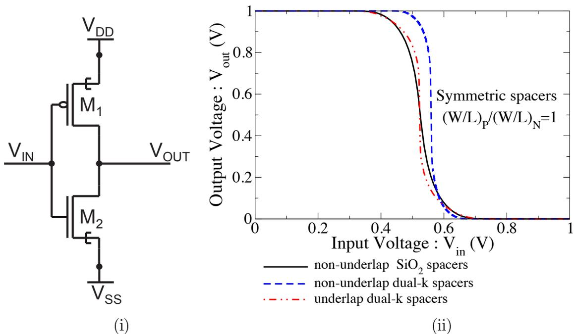
Figure 7.1: (i) Circuit schematic of inverter with TFET. (ii) Simulated DC Transfer characteristic of inverter using symmetric TFETs with (a) non-underlap oxide spacer, (b) non-underlap dual- $k$  spacer, and (c) underlap dual- $k$  spacer.
