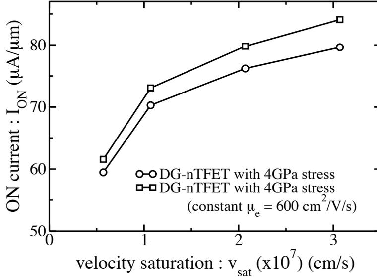
Figure 8.8: The ON current versus velocity saturation in DG-nTFET.
