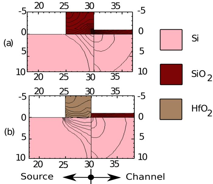
Figure 4.10: Fringe field coupling ( $V_{DS} = 1$  V and  $V_{GS} = 1$  V) through spacer for (a) oxide ( $k = 3.9$ ) and (b) high- $k$  ( $k = 45$ ) spacers. Dimensions are in nanometers.
