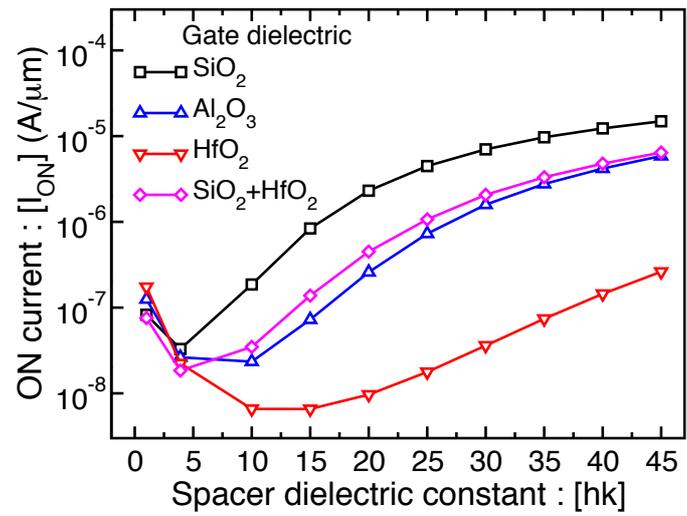
Figure 5.17: Effect of variation of hk spacer dielectric on  $I_{ON}$  of an underlap pTFET with dual-*k* spacer and gate dielectric (EOT = 1.1 nm) of (i) SiO<sub>2</sub> (ii) Al<sub>2</sub>O<sub>3</sub> ( $k = 9.6$ ) (iii) HfO<sub>2</sub> ( $k = 25$ ) and (iv) SiO<sub>2</sub> (physical thickness = 0.8 nm) + HfO<sub>2</sub> (physical thickness = 1.9 nm). The physical thickness of hk spacer is 2 nm and the *k* is varied. The lk spacer is 10 nm of SiO<sub>2</sub>
