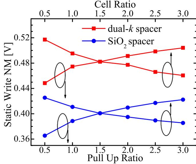
Figure 7.11: WNM of SRAM based on SiO<sub>2</sub> spacer and dual-*k* spacer TFETs for different cell ratios and pull-up ratios
