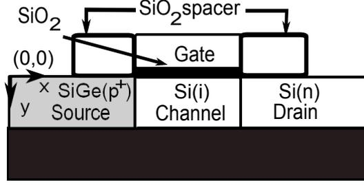
Figure 4.1: Schematic of gated p-i-n structure built on SOI substrates and used as TFET. The source is made of  $\text{Si}_{0.6}\text{Ge}_{0.4}$  and the channel and drain regions are made of Si.
