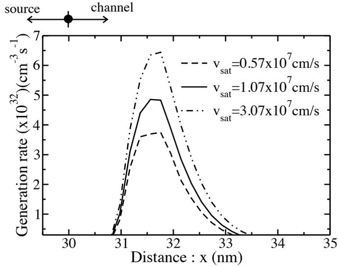
Figure 8.5: The electron generation rate along the channel.
