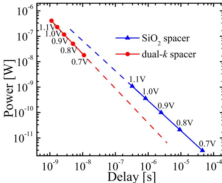
Figure 7.15: Power v/s Delay for ring oscillator circuit using TFET with (i) dual- $k$  spacer (ii) SiO<sub>2</sub> spacer for different  $V_{DD}$ .
