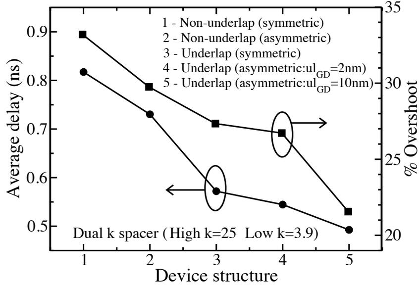
Figure 7.6: Effect of spacer engineering on delay and overshoot of inverter for fanout=1. The gate-to-drain underlap is indicated by  $ul_{GD}$ .
