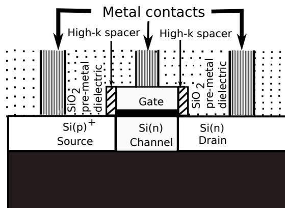
Figure 5.1: Si nTFET with thin layer of high- $k$  spacer. The  $\text{SiO}_2$  pre-metal dielectric layer isolates the gate contact from the source/drain contacts giving a dual- $k$  spacer configuration.
