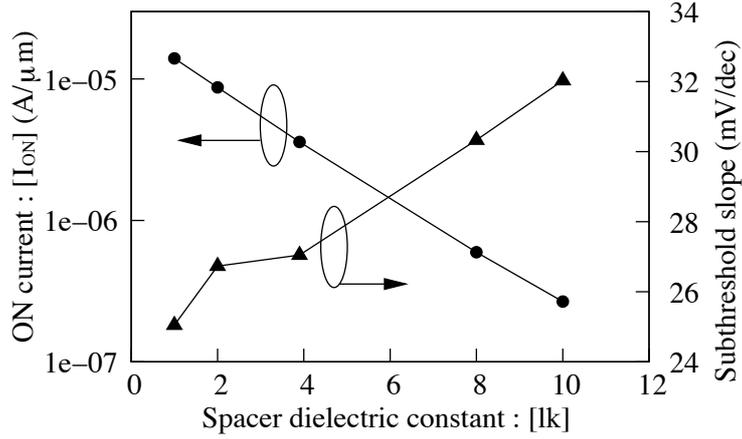
Figure 5.11: Effect of the  $k$  of the lk spacer on DC characteristics of underlap nTFET with HfO<sub>2</sub> ( $k = 25$ ) inner spacer of width 2 nm. The gate dielectric is SiO<sub>2</sub> of 1.1 nm.
