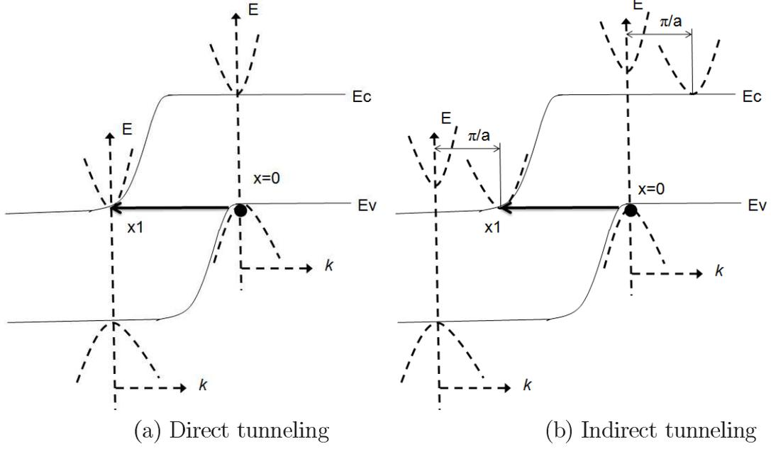
Figure 3.1: Direct and indirect tunneling processes demonstrated by E-k relationship superimposed on the classical turning points ( $x = 0$  and  $x_1$ ) of the tunnel junction. (a) Direct tunneling process with  $k_{min} = k_{max}$  (b) Indirect tunneling process with  $k_{min} \neq k_{max}$  [112].
