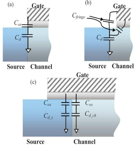
Figure 2.13: (a) Direct gate to channel coupling with aligned gate, (b) gate to channel coupling via fringing capacitance with gate-source underlap, and (c) gate coupling to both source and channel with gate source-overlap. [93].
