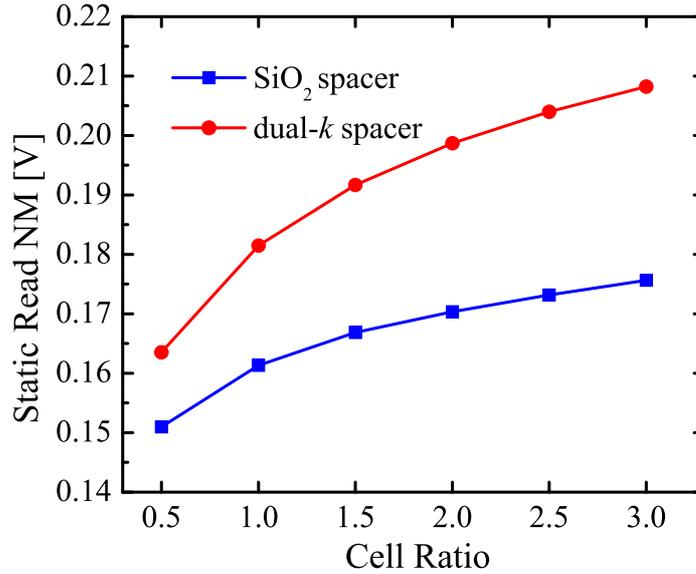
Figure 7.10: RNM vs cell ratios at fixed pull up ratio of 1.5
