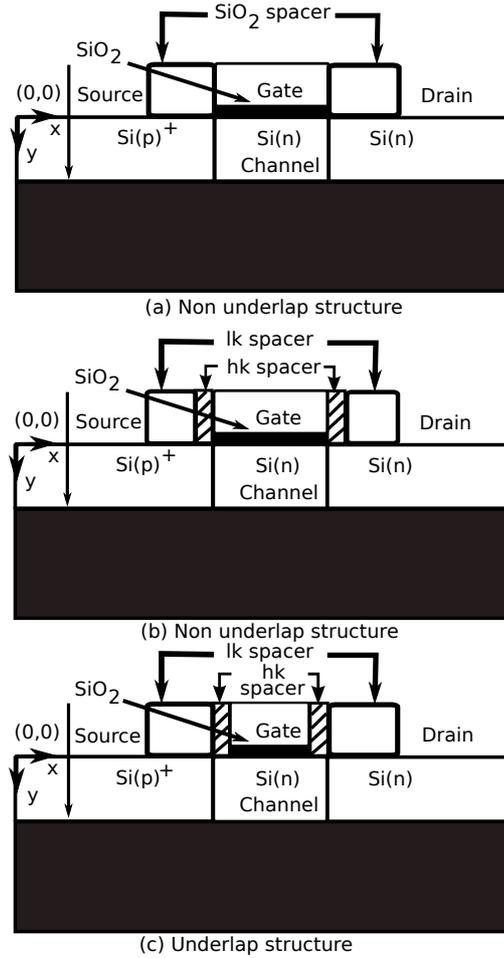
Figure 5.2: Silicon nTFET structures with dual- $k$  spacer investigated in this chapter. (a) Non-underlap structure with SiO<sub>2</sub> spacer, (b) Non-underlap structure with dual- $k$  spacer and (c) Underlap structure with dual- $k$  spacer.
