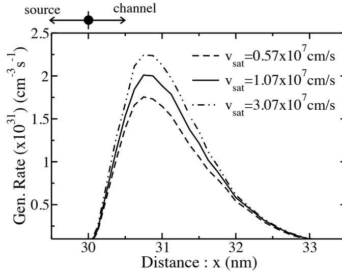
Figure 8.9: The generation rate along the channel in DG-nTFET.
