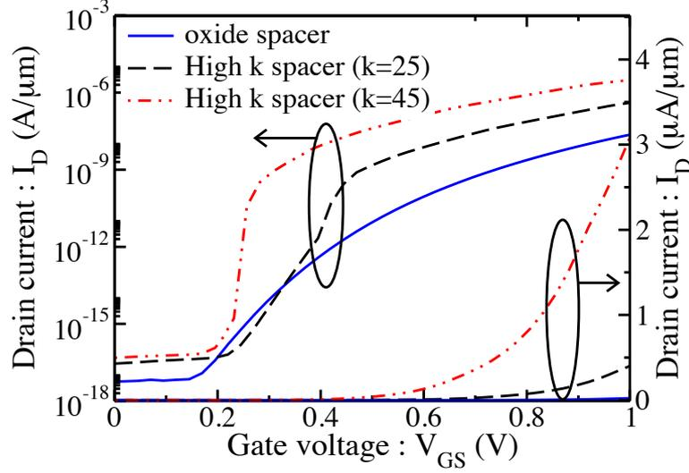
Figure 4.8:  $I_D$ - $V_{GS}$  characteristics of Si nTFETs with spacer of various dielectric constants. Gate length = 20 nm, spacer thickness = 5 nm and  $V_{DS} = 1$  V.
