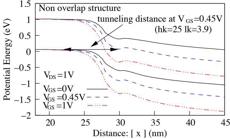
Figure 5.6: Band diagram of the nTFET with dual- $k$  spacer and non-underlap structure. The spacer  $k$  is 25 and the band diagrams are shown for various values of  $V_{GS}$ . The gate dielectric is  $\text{SiO}_2$  of 1.1 nm thickness.
