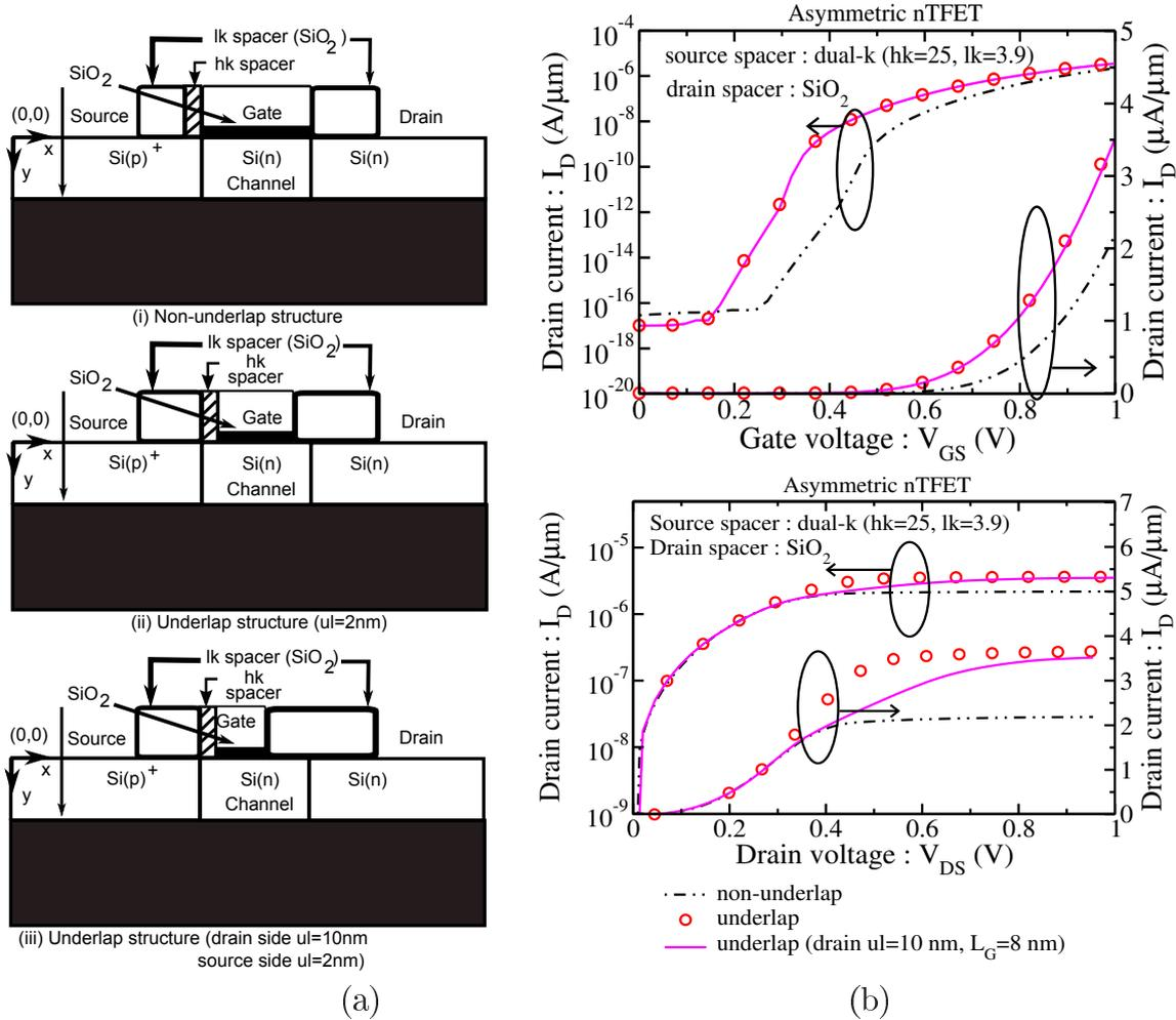
Figure 5.18: (a) **Asymmetric nTFET** structures with dual- $k$  spacer. (i) Non-underlap structure, (ii) Underlap structure (drain side  $ul = 2$  nm) and (iii) Underlap structure (drain side  $ul = 10$  nm). (b)  $I_D$ - $V_{GS}$  and  $I_D$ - $V_{DS}$  characteristics of TFETs shown in (a).
