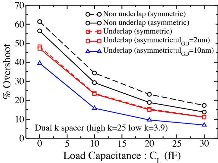
Figure 7.5: Effect of spacer engineering on peak overshoot of inverter for different  $C_L$  ( $V_{in}$ :  $t_r = t_f = 1$  ns and  $T_p = 102$  ns). The gate-to-drain underlap is indicated by  $ul_{GD}$ .
