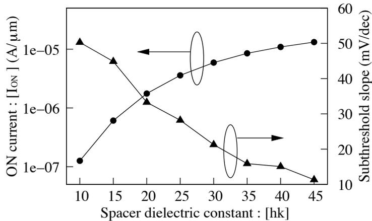
Figure 5.10: Effect of the  $k$  of the hk spacer on DC characteristics of the underlap nTFET with dual- $k$  spacer. The lk spacer is made of  $\text{SiO}_2$ . Thickness of the hk spacer is 2 nm and the thickness of the lk spacer is 10 nm. The gate dielectric is  $\text{SiO}_2$  of 1.1 nm thickness.
