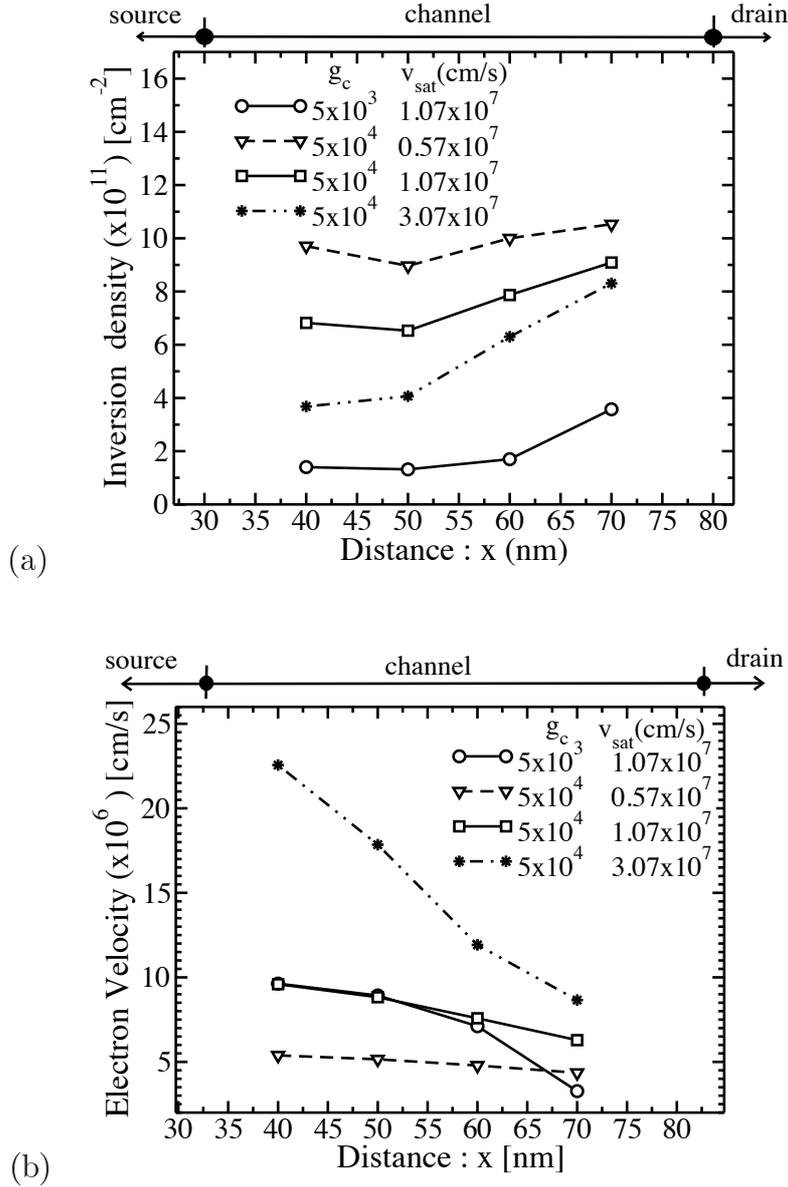
Figure 8.3: Effect of increasing the generation rate by increasing  $g_c$  and  $g_v$  in the non local tunneling model on (a) the inversion density and (b) the average velocity of electrons along the channel.
