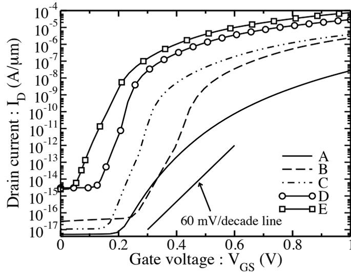
Figure 8.7: The  $I_D$ - $V_{GS}$  characteristics for different technology boosters. (A) non-underlap nTFET with  $\text{SiO}_2$  spacer (Fig. 5.2(a)); (B) non-underlap nTFET with dual- $k$  spacer (Fig. 5.2(b)); (C) same as B with underlap structure (Fig. 5.2(c)); (D) same as C with 4 GPa uniaxial tensile stress in the source/drain direction; (E) underlap DG-nTFET with dual- $k$  spacer and 4 GPa uniaxial tensile stress in the source/drain direction (Fig. 8.1).
