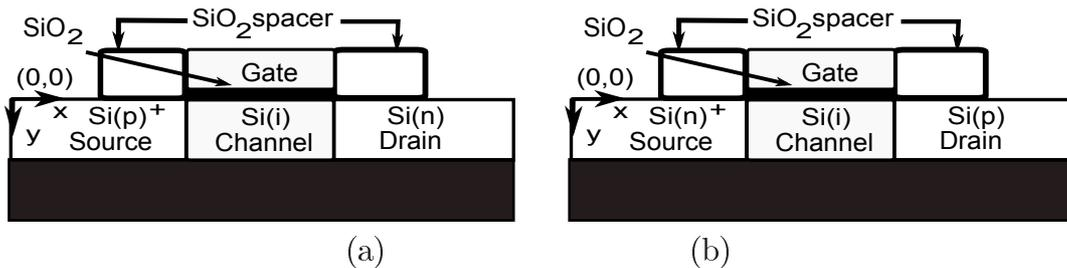
Figure 3.5: Lateral TFET structures. (a) n-channel TFET and (b) p-channel TFET.
