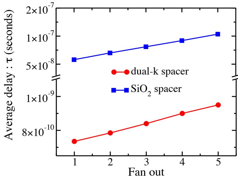
Figure 7.12: Average time delay as a function of fanout for inverter using (a) non-underlap TFET with SiO<sub>2</sub> spacer and (b) underlap TFET with dual-*k* spacer.
