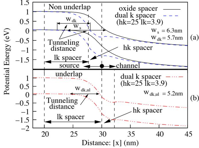
Figure 5.5: Band diagram for nTFET with (a) SiO<sub>2</sub> spacer and dual- $k$  spacer in non-underlap structure and (b) dual- $k$  spacer in underlap structure. The tunneling width is indicated by  $w_s$  and  $w_{dk}$  for the SiO<sub>2</sub> single spacer and dual- $k$  spacer non-underlap structures respectively. The same is referred in underlap structure with dual- $k$  spacer by  $w_{dk,ul}$ .  $V_{DS} = V_{GS} = 1$  V.
