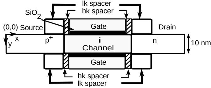
Figure 8.1: Underlap DG-nTFET structure ( $L_g = 46$  nm). Body thickness is 10 nm.
