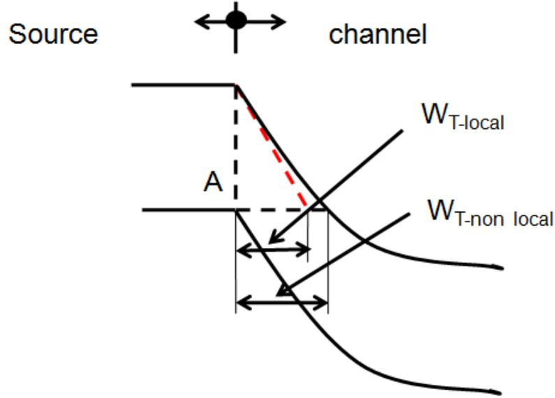
Figure 2.5: The local model for band to band tunneling computes smaller tunneling width ( $W_{T-local}$ ) as compared to that of non local model ( $W_{T-nonlocal}$ ).
