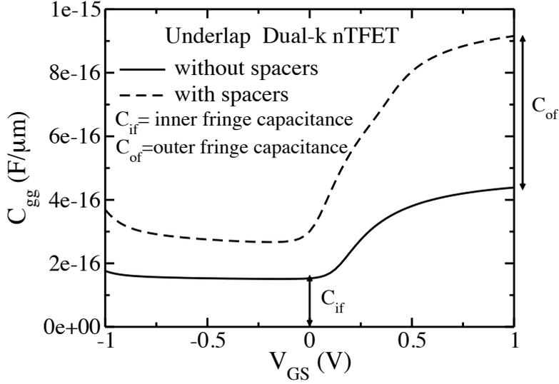
Figure 6.4: Capacitance - voltage characteristics for symmetric underlap TFET with dual- $k$  spacer (Fig. 5.2(c)) illustrating the computation of the inner and outer fringe capacitance. The gate dielectric is 1.1 nm  $\text{SiO}_2$ .  $V_{DS} = 0$  V.
