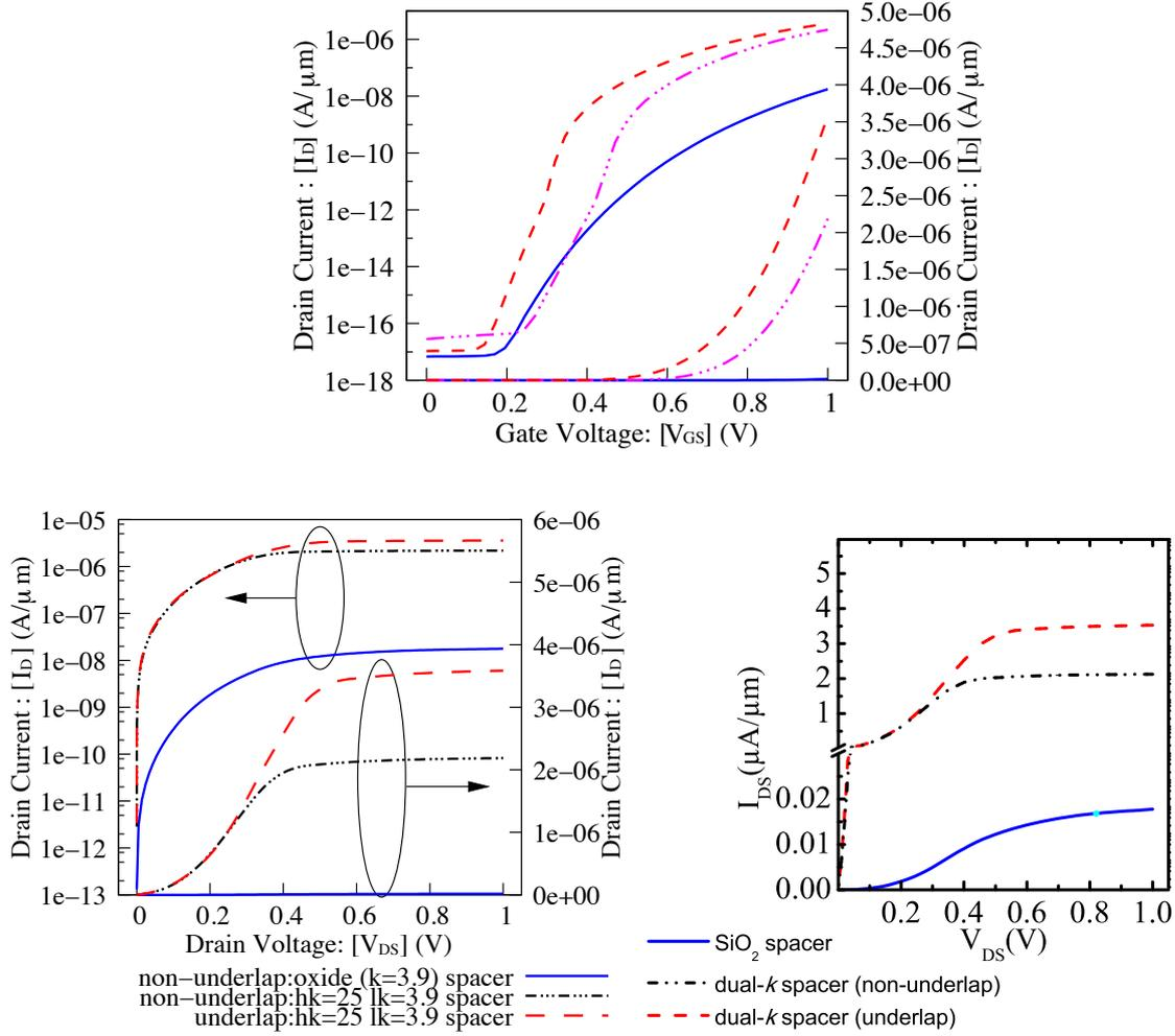
Figure 5.3:  $I_D$ - $V_{GS}$  characteristic ( $V_{DS} = 1$  V) and  $I_D$ - $V_{DS}$  characteristic ( $V_{GS} = 1$  V) for (a) non-underlap nTFET structure with SiO<sub>2</sub> spacer, (b) non-underlap nTFET structure with dual- $k$  spacer made of HfO<sub>2</sub> and SiO<sub>2</sub> and (c) underlap nTFET structure with dual- $k$  spacer made of HfO<sub>2</sub> and SiO<sub>2</sub>. The gate dielectric is SiO<sub>2</sub> of 1.1 nm thickness.
