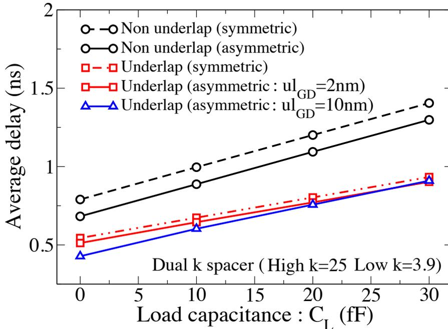
Figure 7.4: Effect of spacer engineering on delay of inverter for different  $C_L$  ( $V_{in}$ :  $t_r = t_f = 1$  ns and  $T_p = 102$  ns). The gate-to-drain underlap is indicated by  $ul_{GD}$ .
