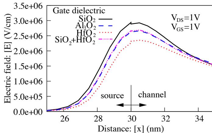
Figure 5.13: Effect of the gate dielectric on the electric field below the top surface of the semiconductor for an underlap nTFET with dual-k spacer for the four cases shown in Fig. 5.12. The  $hk$  spacer is  $\text{HfO}_2$  with physical thickness of 2 nm and  $k$  of 25. The  $lk$  spacer is 10 nm of  $\text{SiO}_2$ .
