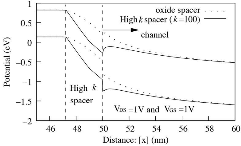
Figure 4.5: Band diagram showing the reduction of tunneling width in  $\text{Si}_{0.6}\text{Ge}_{0.4}$  hetero junction nTFET when a high- $k$  spacer ( $k = 100$ ) is used. A small bump (upward shift) is seen in the band diagram on the "i" side of the junction when a high- $k$  spacer is used.
