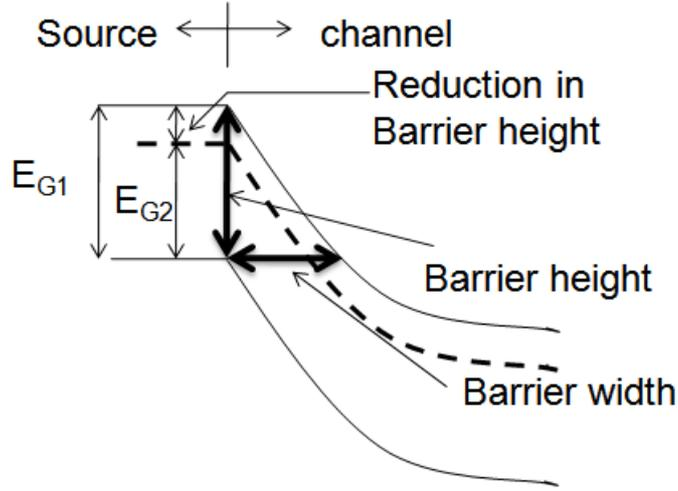
Figure 2.6: Reduction in tunneling barrier height.  $E_{G1}$  and  $E_{G2}$  are forbidden bandgap of material 1 and material 2.
