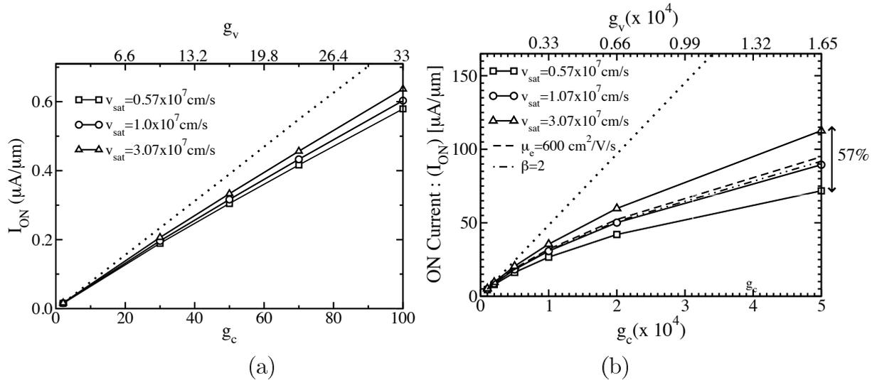
Figure 8.2: The effect of increasing the generation rate by increasing  $g_c$  and  $g_v$  in the non local tunneling model on  $I_{ON}$  for (a) low and (b) high values of  $g_c$  and  $g_v$ .  $I_{ON}$  for  $\mu_e = 600$   $\text{cm}^2/\text{V/s}$  and  $\beta = 2$  are computed for  $v_{sat} = 1.07 \times 10^7$   $\text{cm/s}$ . The dotted straight line corresponds to an  $I_{ON}$  proportional to  $g_c$ .
