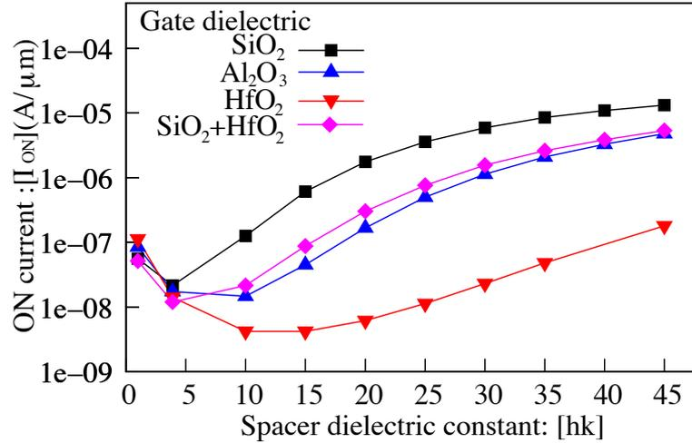
Figure 5.12: Effect of variation of hk spacer dielectric on  $I_{ON}$  of an underlap nTFET with dual-k spacer and gate dielectric (EOT = 1.1 nm) of (i) SiO<sub>2</sub> (ii) Al<sub>2</sub>O<sub>3</sub> ( $k = 9.6$ ) (iii) HfO<sub>2</sub> ( $k = 25$ ) and (iv) SiO<sub>2</sub> (physical thickness = 0.8 nm) + HfO<sub>2</sub> (physical thickness = 1.9 nm). The physical thickness of hk spacer is 2 nm and the  $k$  is varied. The lk spacer is 10 nm of SiO<sub>2</sub>.
