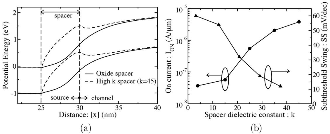
Figure 4.13: (a) Band diagram showing the reduction of tunneling width in pTFET when a high- $k$  spacer ( $k = 45$ ) is used.  $V_{GS} = -1$  V and  $V_{DS} = -1$  V. (b) Effect of spacer dielectric constant on  $I_{ON}$  and average Subthreshold Swing of pTFET.
