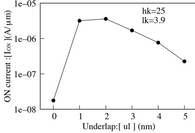
Figure 5.9: Effect of hk spacer width on  $I_{ON}$ . The hk spacer has a  $k$  of 25 ( $\text{HfO}_2$ ). The gate dielectric is  $\text{SiO}_2$  of 1.1 nm thickness.
