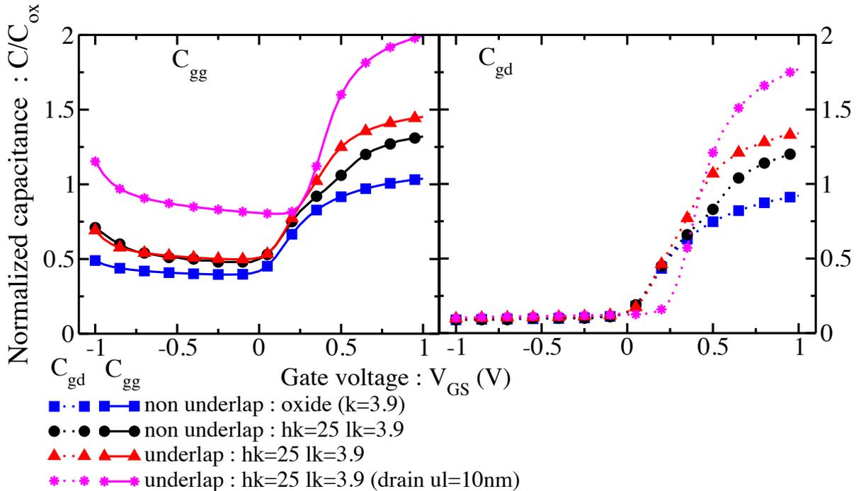
Figure 6.2: Capacitance - voltage characteristics for **asymmetric** structures showing the gate and gate-to-drain capacitances as a function of gate-to-source voltage,  $V_{GS}$  for the three cases shown in Fig. 5.18. The drain side spacer is replaced with a single  $\text{SiO}_2$  spacer. The gate dielectric is 1.1 nm  $\text{SiO}_2$ .  $V_{DS} = 0$  V.
