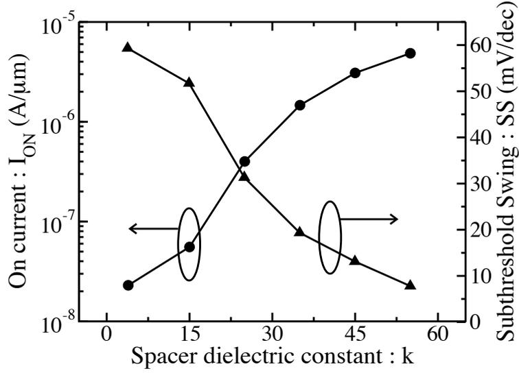
Figure 4.9: Effect of spacer dielectric constant on  $I_{ON}$  and average Subthreshold Swing of nTFET.
