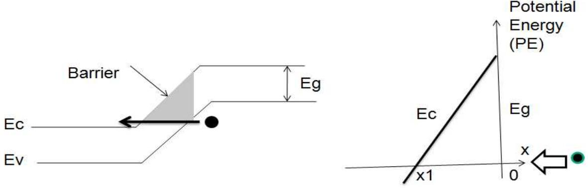
Figure 3.2: Tunneling in a tunnel diode can be analyzed by a triangular potential barrier [112].
