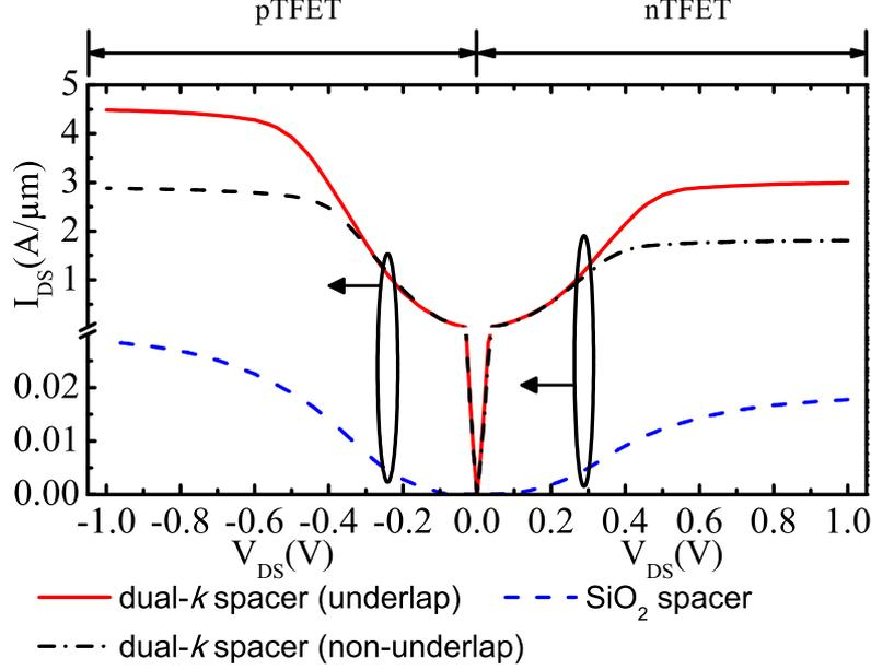
Figure 7.2:  $I_D$ - $V_{DS}$  characteristic ( $V_{GS} = 1$  V) for (a) non-underlap TFET structure with  $\text{SiO}_2$  spacer, (b) non-underlap TFET structure with dual- $k$  spacer made of  $\text{HfO}_2$  and  $\text{SiO}_2$  and (c) underlap TFET structure with dual- $k$  spacer made of  $\text{HfO}_2$  and  $\text{SiO}_2$ . The gate dielectric is  $\text{SiO}_2$  of 1.1 nm thickness.
