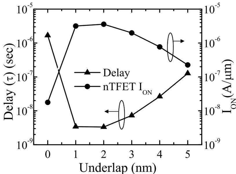
Figure 7.16: Effect of hk spacer width on I<sub>ON</sub> and inverter delay for the underlap TFET with dual-k spacer. The hk spacer has a *k* of 25 (HfO<sub>2</sub>). Gate dielectric is SiO<sub>2</sub> of 1.1 nm thickness.
