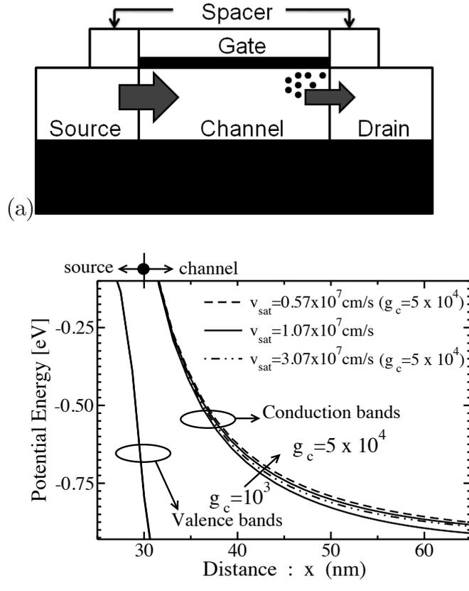
Figure 8.4: (a) Carrier accumulation near the drain. Thickness of the arrow is indicative of the magnitude of carriers moving in the direction of the arrow. (b) Effect of increasing the generation rate by increasing  $g_c$  and  $g_v$  in the non local tunneling model on the band diagram.
