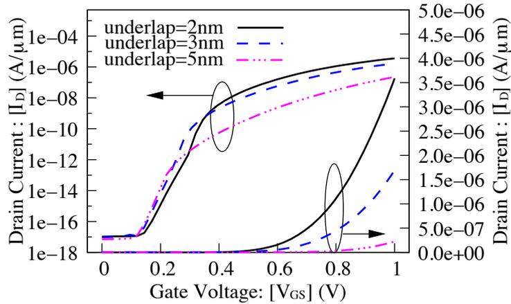
Figure 5.7: Effect of  $hk$  spacer width variation on  $I_D$ - $V_{GS}$  characteristic of the underlap structure ( $V_{DS} = 1$  V). The gate dielectric is  $\text{SiO}_2$  of 1.1 nm thickness.
