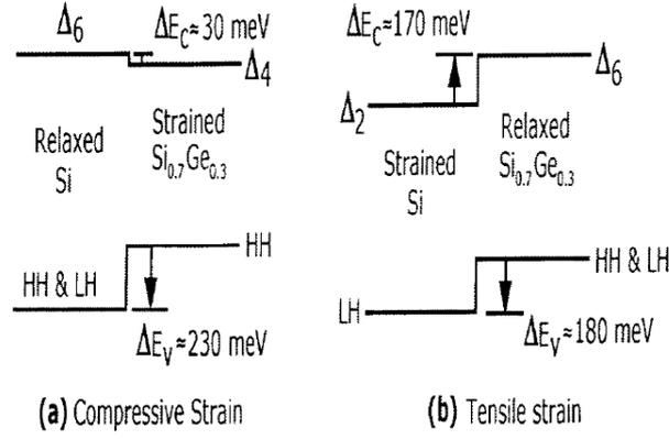
Figure 2.9: (a) Band alignments between Si and  $\text{Si}_{0.7}\text{Ge}_{0.3}$  on two substrates: (a) Si (Type I staggered junction) and (b)  $\text{Si}_{0.7}\text{Ge}_{0.3}$  (Type II staggered junction) [73].
