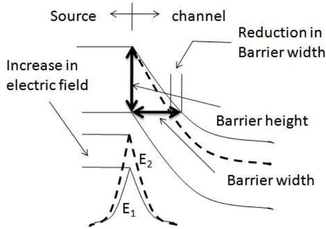
Figure 2.11: Reduction in tunneling barrier width when the electric field at the source-channel junction is enhanced from  $E_1$  to  $E_2$ .
