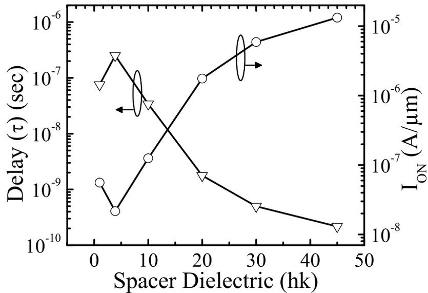
Figure 7.18: Effect of variation of hk spacer dielectric on DC characteristics of an underlap nTFET with dual- $k$  spacer and gate dielectric is  $SiO_2$  of 1.1 nm thickness. The hk spacer physical thickness is 2 nm and the  $k$  is varied. The lk spacer is 10 nm of  $SiO_2$ .
