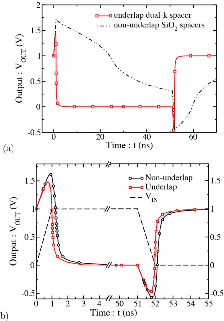
Figure 7.3: Transient characteristic of inverter using (a) symmetric non-underlap TFETs with  $\text{SiO}_2$  spacer and symmetric underlap TFETs with dual- $k$  spacer and (b) symmetric non-underlap and underlap TFETs with dual- $k$  spacers. (For both (a) and (b),  $V_{in}$ :  $t_r = t_f = 1$  ns,  $T_p = 102$  ns and  $C_L = 0$ ).
