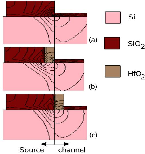
Figure 5.4: Fringe field coupling through spacer for the three cases shown in Fig. 5.3.  $V_{DS} = V_{GS} = 1$  V.
