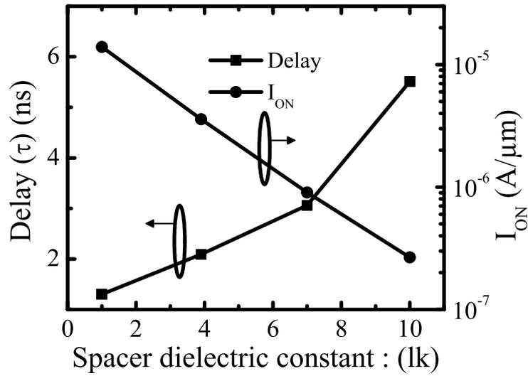
Figure 7.17: Effect of the dielectric constant of the lk spacer on performance of the underlap TFET with dual- $k$  spacer. The hk spacer is made of  $HfO_2$  ( $k = 25$ ). The  $I_{ON}$  of nTFET with dual- $k$  spacer is shown in the graph. The gate dielectric is  $SiO_2$  of 1.1 nm thickness.
