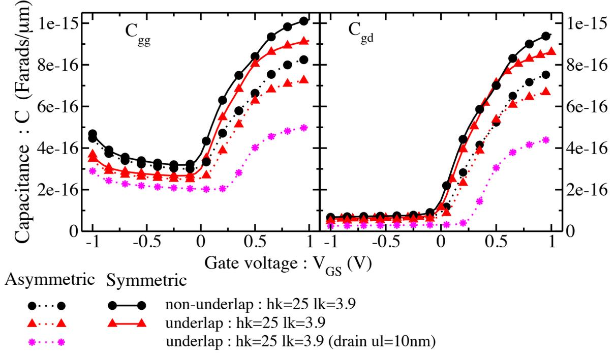
Figure 6.3: Capacitance - voltage characteristics showing a reduction in capacitance for asymmetric TFETs compared to that of symmetric TFETs. The gate dielectric is 1.1 nm  $\text{SiO}_2$ .  $V_{DS} = 0$  V.
