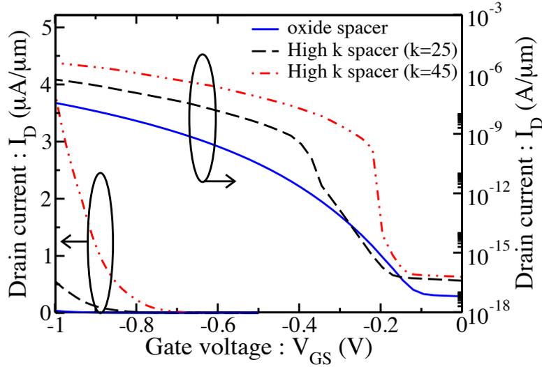
Figure 4.12:  $I_D$ - $V_{GS}$  characteristics of Si pTFETs with spacer of various dielectric constants. Gate length = 20 nm, spacer thickness = 5 nm and  $V_{DS} = -1$  V.
