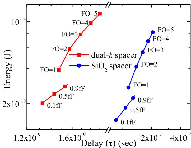
Figure 7.13: Energy vs Delay for different fan-outs and different load capacitances.
