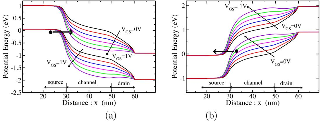
Figure 2.2: Band diagram of TFET for various gate bias. (a) nTFET ( $V_{DS} = 1$  V) and (b) pTFET ( $V_{DS} = -1$  V).
