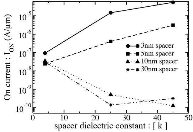
Figure 4.14: Impact of spacer width on  $I_{ON}$  of nTFET with the spacer  $k$  variation.
