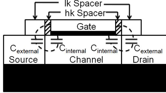
Figure 5.14: Conceptual model depicting electric field coupling through (a) external field (fringe field via the spacer) and (b) internal field (fringe field via gate dielectric).
