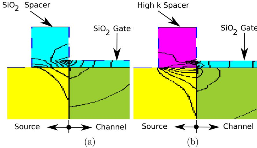
Figure 4.4: Fringe field coupling ( $V_{DS} = 1$  V and  $V_{GS} = 1$  V) through spacer for (a) oxide ( $k = 3.9$ ) and (b) high- $k$  ( $k = 100$ ) spacers. The gate dielectric is  $\text{SiO}_2$  with a thickness of 1.1 nm.
