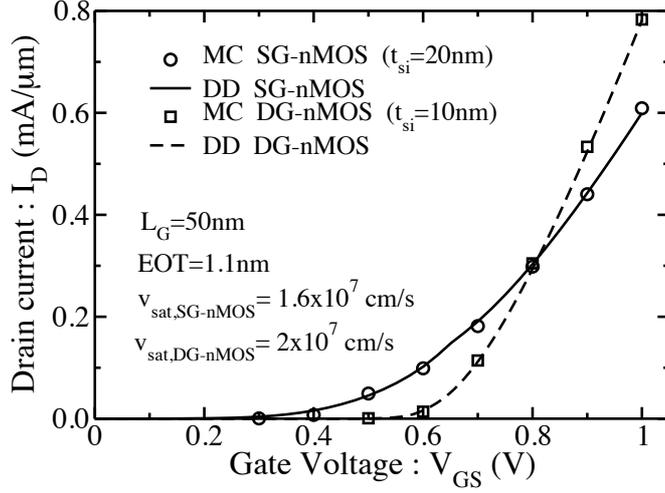
Figure 8.6: The simulated characteristic of SG-nMOS and DG-nMOS with  $v_{sat} = 1.6 \times 10^7$  cm/s and  $v_{sat} = 2 \times 10^7$  cm/s respectively. MSMC model as in [128].  $t_{si}$  is the thickness of silicon.
