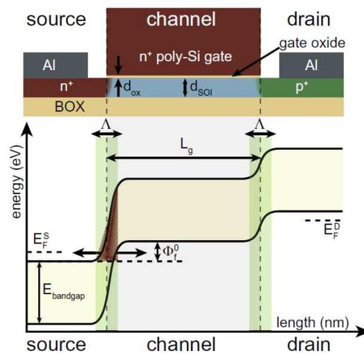
Figure 2.12: Structure of a TFET on SOI substrate and the band profile along current transport direction. The extent of the tunneling barrier is given by  $\Lambda$ , the screening length for potential variations. The barrier is approximated by the hatched triangular shape. [84].
