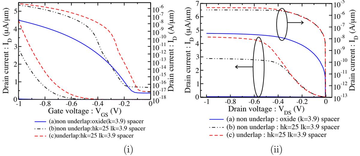
Figure 5.15: (i)  $I_D$ - $V_{GS}$  characteristic ( $V_{DS} = 1$  V) and (ii)  $I_D$ - $V_{DS}$  characteristic ( $V_{GS} = 1$  V) for (a) non-underlap pTFET structure with  $\text{SiO}_2$  spacer, (b) non-underlap pTFET structure with dual- $k$  spacer made of  $\text{HfO}_2$  and  $\text{SiO}_2$  and (c) underlap pTFET structure with dual- $k$  spacer made of  $\text{HfO}_2$  and  $\text{SiO}_2$ . The gate dielectric is 1.1 nm  $\text{SiO}_2$ .
