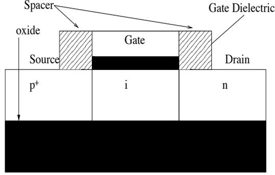
Figure 1.1: Schematic of gated p-i-n TFET structure built on SOI substrates.
