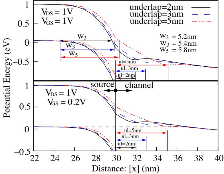
Figure 5.8: Band diagram corresponding to the  $I_D$ - $V_{GS}$  shown in Fig. 5.7 for two gate voltages. Tunneling width is indicated by  $w$  and  $ul$  refers to the the underlap. For  $V_{GS} = 0.2$  V, the tunneling path is indicated by the horizontal broken line.
