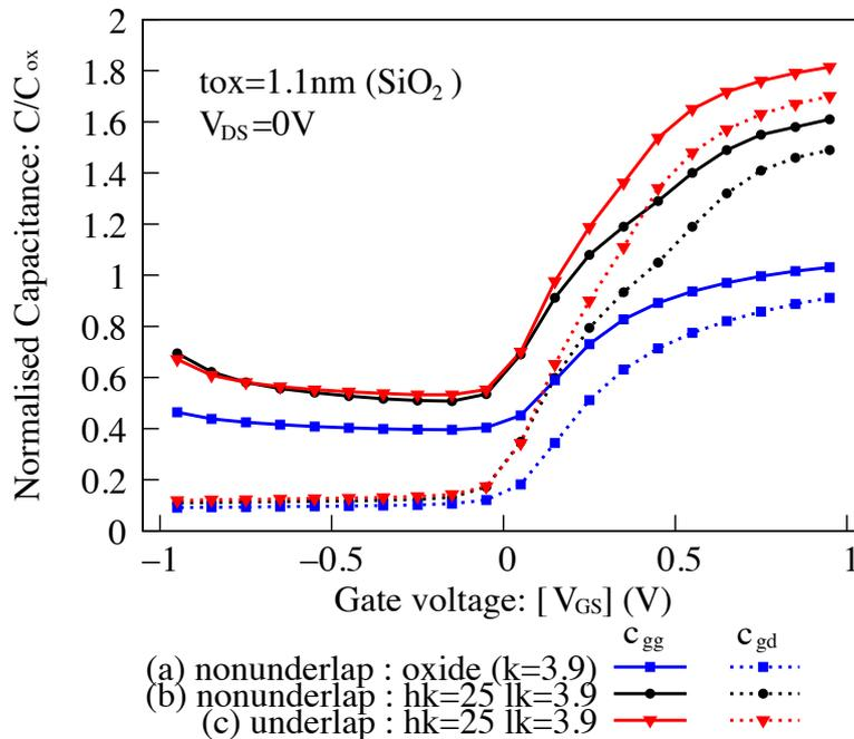
Figure 6.1: Capacitance - voltage characteristics for symmetric structures showing the gate and gate-to-drain capacitances as a function of gate-to-source voltage,  $V_{GS}$  for the three cases shown in Fig. 5.2. The gate dielectric is 1.1 nm SiO<sub>2</sub>.  $V_{DS} = 0$  V.
