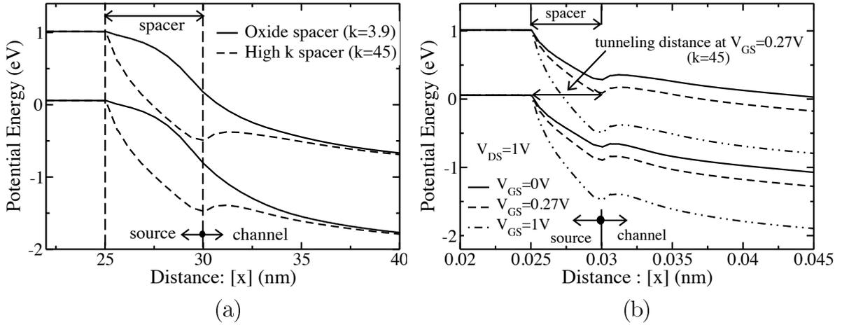
Figure 4.11: (a) Band diagram showing the reduction of tunneling width in nTFET when a high- $k$  spacer ( $k = 45$ ) is used.  $V_{GS} = 1$  V and  $V_{DS} = 1$  V. (b) Band diagram of the nTFET with spacer  $k$  of 45 for various values of  $V_{GS}$  ( $V_{DS} = 1$  V).
