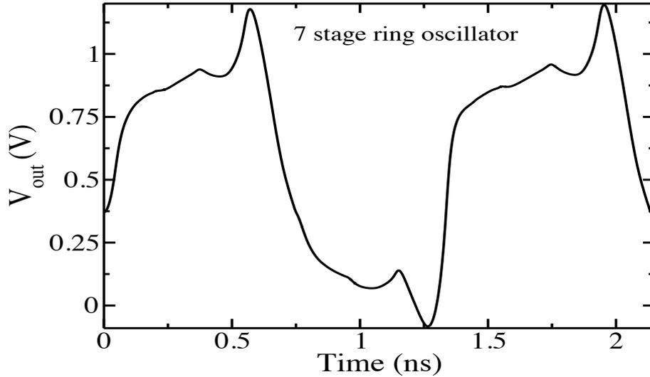
Figure 7.7: Output waveform of seven stage ring oscillator. The underlap structure with dual- $k$  spacer and stress = 4 GPa have been used.
