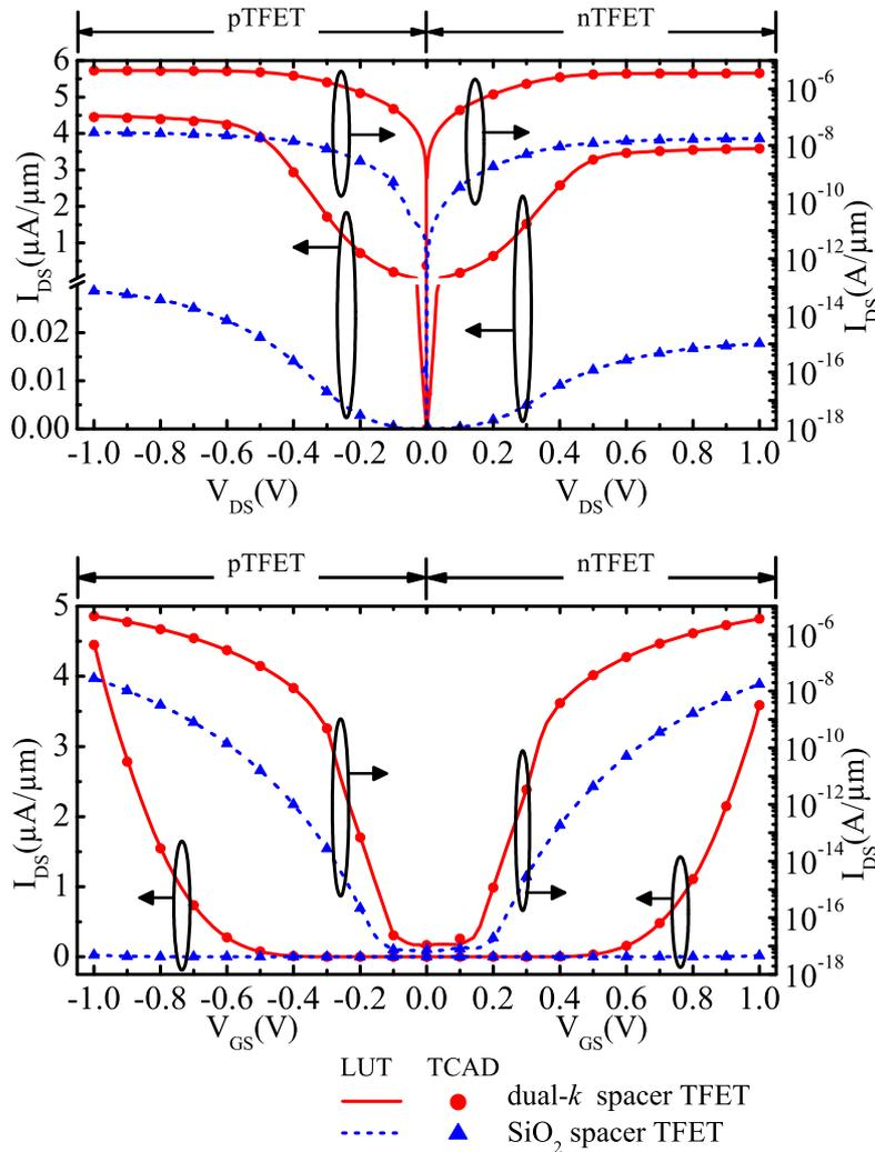
Figure 7.8: The  $I_D$ - $V_{DS}$  characteristic at  $V_{GS} = 1$  V and  $I_D$ - $V_{GS}$  characteristic at  $V_{DS} = 1$  V for nTFET and pTFET indicates an agreement with the TCAD generated characteristic.
