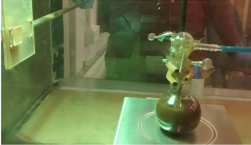
Figure 5.2: The experimental setup that was used to deposit dust on the solar glass samples.
