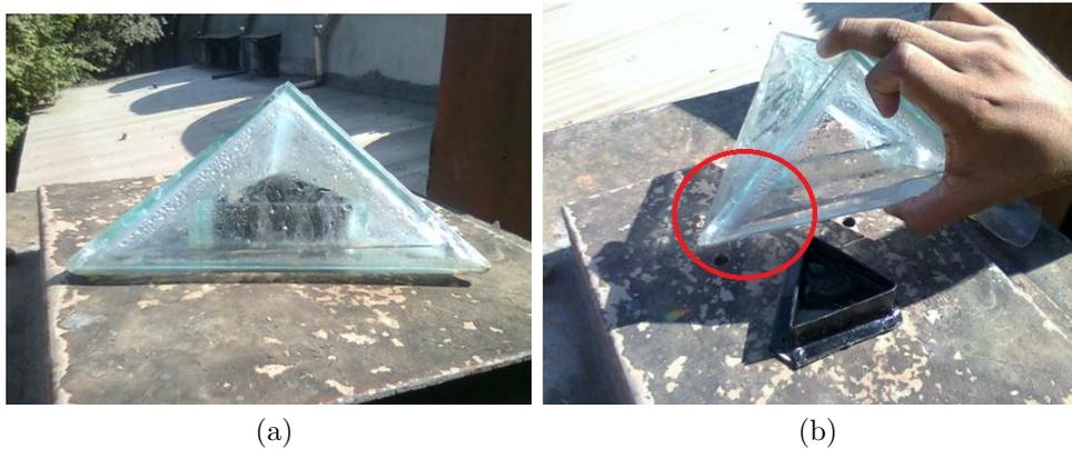
Figure 6.7: Filtration experiment using solar energy image showing evaporation (a), and condensation happening on the glass surface (b). Circled area shows the clean water collected during the evaporation and condensation.
