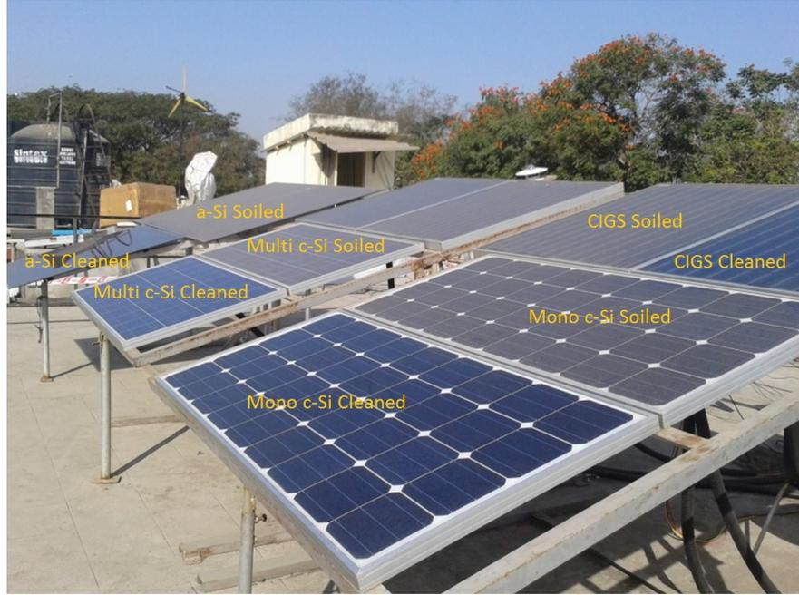
Figure 3.1: Soiling station installed in Mumbai, having 2 modules of each PV module technologies, such as monocrystalline silicon (mono c-Si), multi-crystalline silicon (multi c-Si), amorphous silicon (a-Si) and CIGS.
