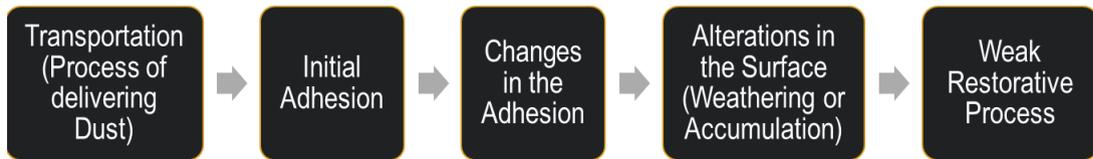
Figure 2.1: Process involved in soiling or dust deposition on surfaces such as PV modules.
