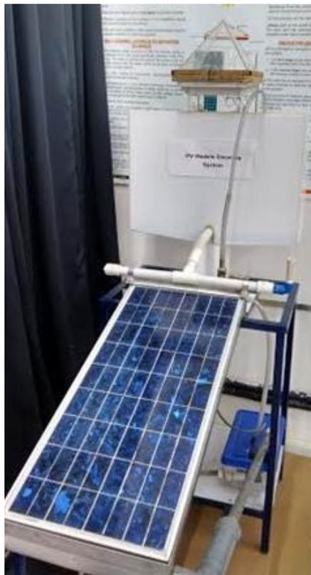
Figure 6.10: Prototype of water from humidity system, storage tank and pipe based dispersing mechanism.
