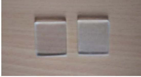
Figure 6.17: Image of the two solar glass coupons with  $TiO_2$  coating (Right) and without  $TiO_2$  coating (Left).
