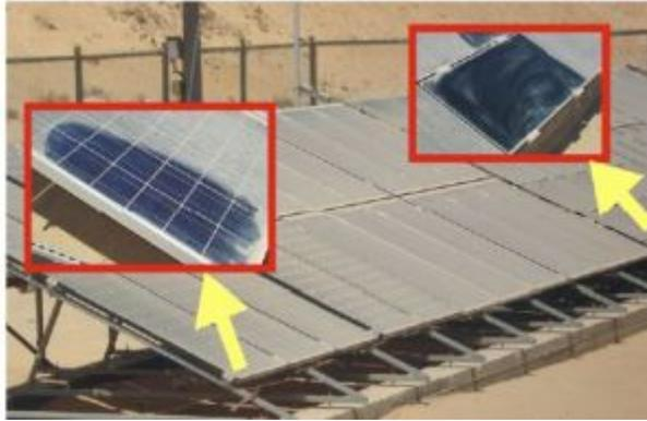
Figure 2.6: Dust accumulation on PV modules after a dust storm [34].
