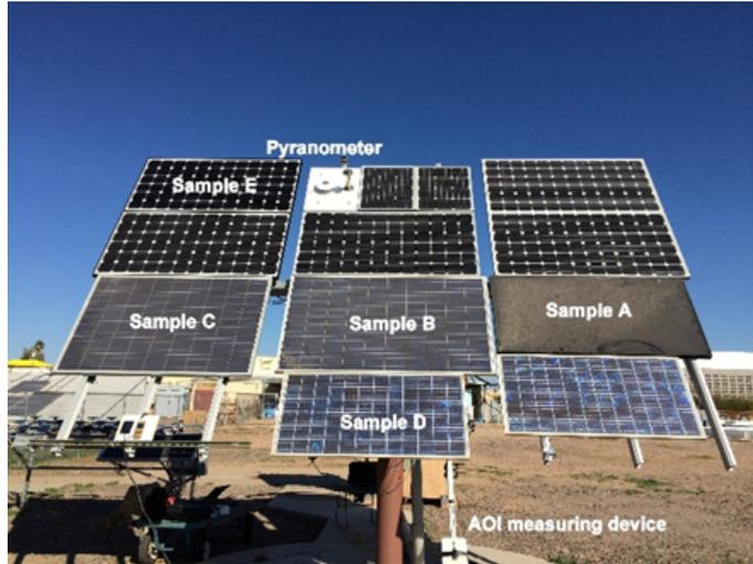
Figure 4.4: Outdoor experimental setup for AOI measurement [Soiling level: A – Heavy ( $11.8 \text{ g/m}^2$ ), B – Moderate ( $4.85 \text{ g/m}^2$ ), C – Moderate ( $2.74 \text{ g/m}^2$ ), D –Light ( $1.71 \text{ g/m}^2$ ); E – Cleaned].
