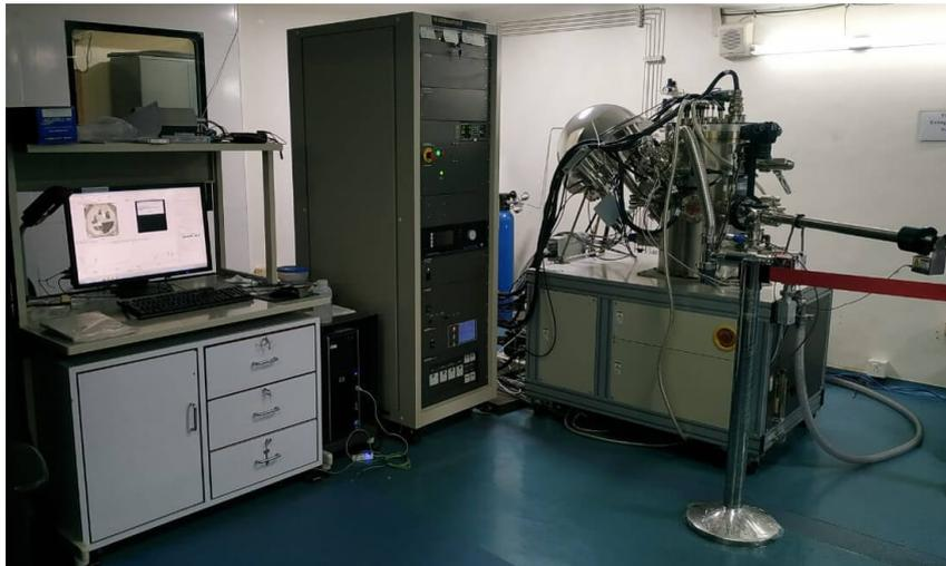
**Figure A.4:** Photograph of X-ray Photoelectron Spectroscopy instrument.
