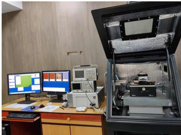
**Figure A.5:** Photograph of AFM measurement instrument.
