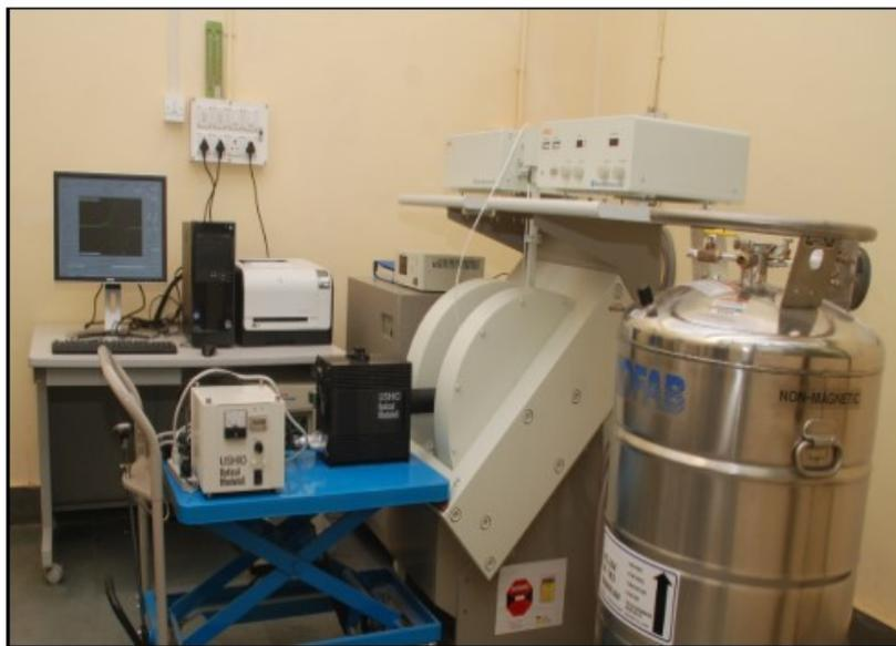
**Figure A.14:** Photograph of electron spin resonance spectrometer [149].
