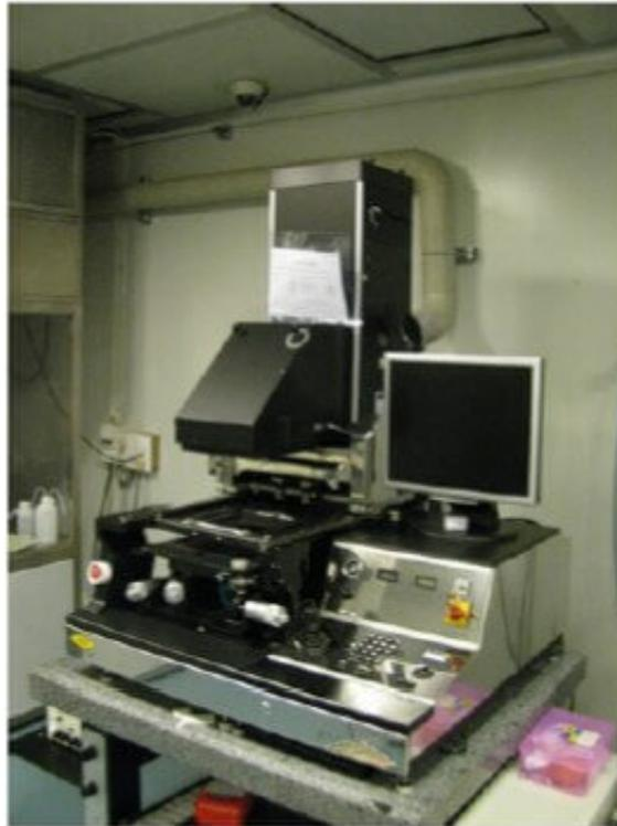
**Figure A.7:** A photograph of EVG 620 photolithography tool [148].
