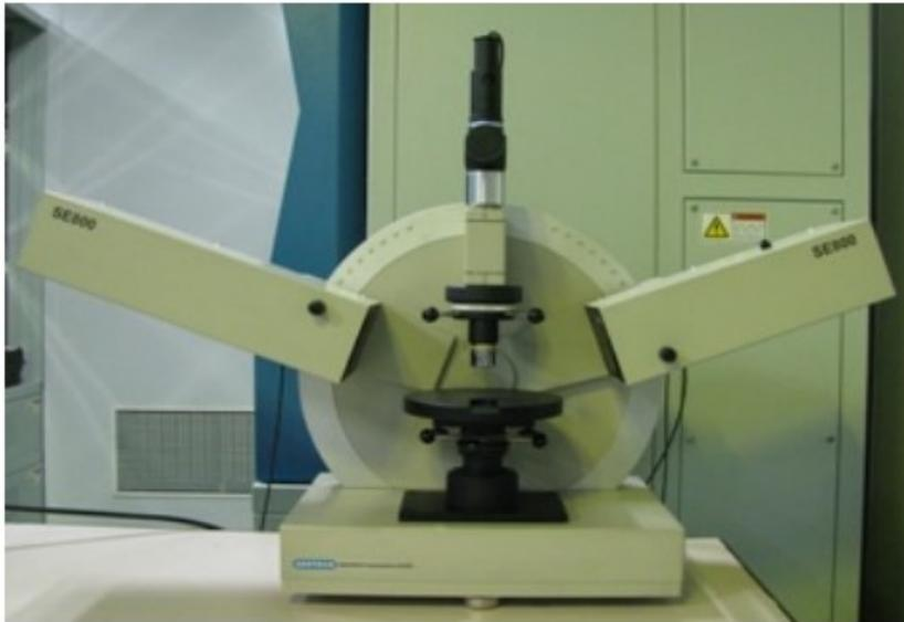
**Figure A.1:** Photograph of ellipsometer [148].
