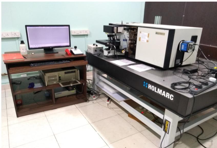
**Figure A.3:** Photograph of Raman spectroscopy instrument [149].
