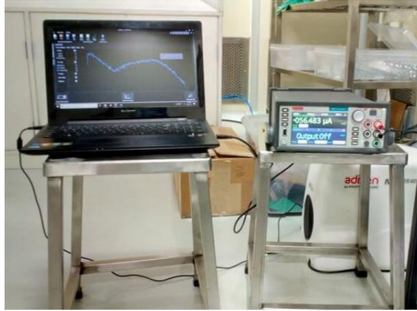
**Figure A.9:** Photograph of Keithley 2450 connected with a laptop for current measurement.
