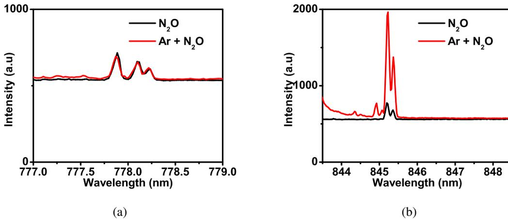
Fig. 6.12: Comparison of OES spectra for  $N_2O$  and  $Ar + N_2O$  plasma at (a) 777 nm (b) 844 nm.
