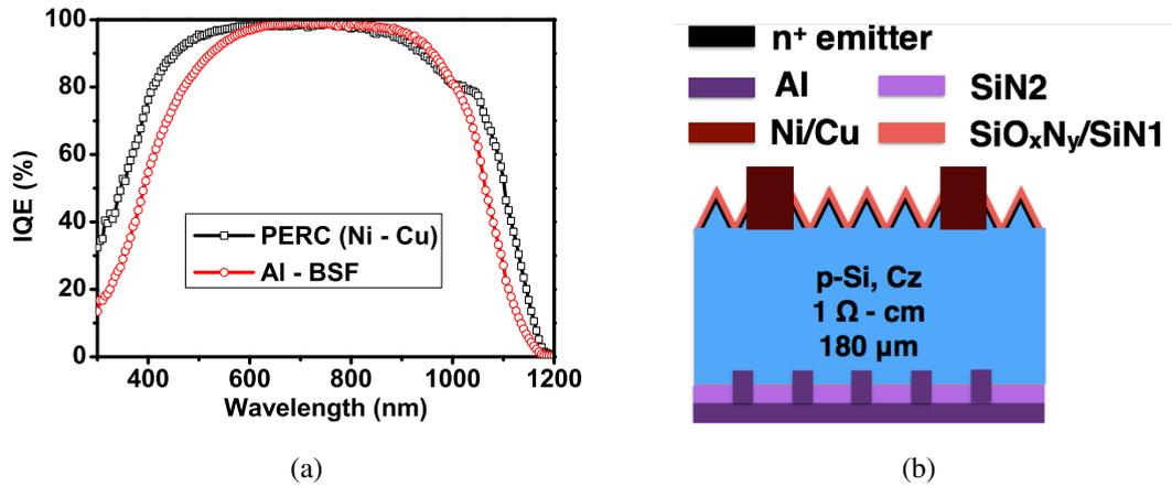
Fig. 7.12: (a) EQE of a PERC solar cell compared with a screen printed solar cell [153] (b) Schematic of the PERC solar cell fabricated.
