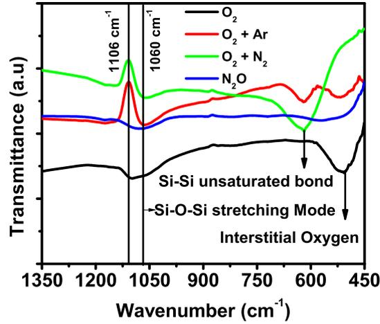
Fig. 5.5: FTIR spectrum for plasma grown films in different ambient.
