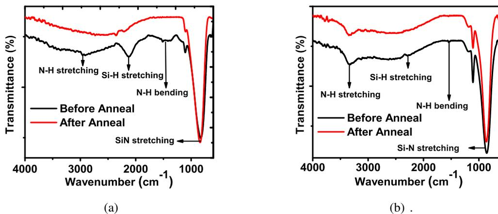
Fig. 8.8: FTIR spectrum before and after firing for (a) SiN<sub>x</sub>:H film deposited using a silane flow of 11 sccm. The film blistered upon firing at 800°C (b) SiN<sub>x</sub>:H film deposited using a silane flow of 3.5 sccm. The film did not exhibit any blistering upon firing at 800°C.
