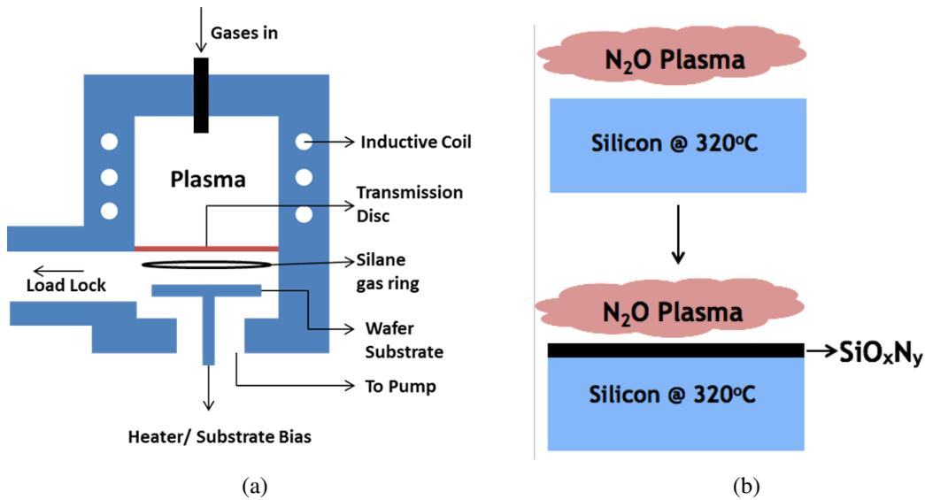
Fig. 5.2: (a) Schematic of ICP system used for experiments (b) Schematic of plasma oxidation process.
