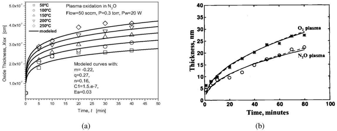
Fig. 2.6: (a) Modified power law based model for PECVD grown oxides [76] (b) Parabolic growth rate model for oxide films grown in ICP chamber [80].
