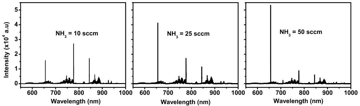
Fig. 5.12: Optical emission characteristics of  $N_2O + NH_3$  plasma for varying ammonia flow rates.
