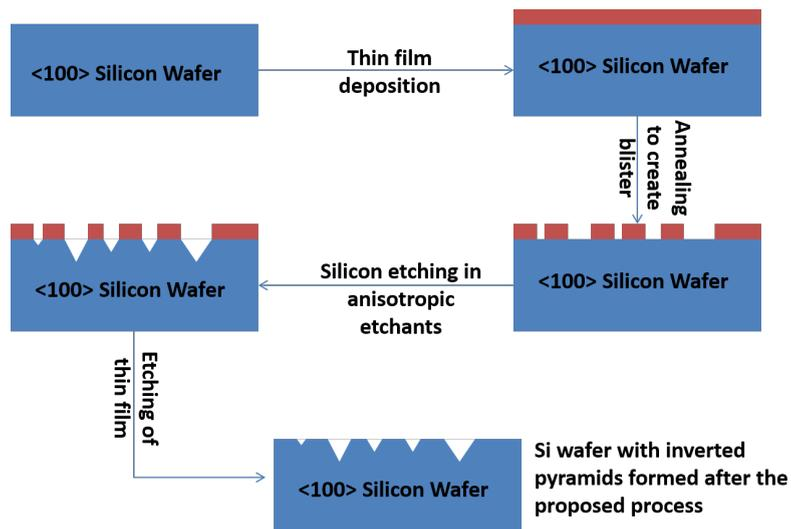
Fig. 8.2: Process flow for fabrication of inverted pyramids on silicon.
