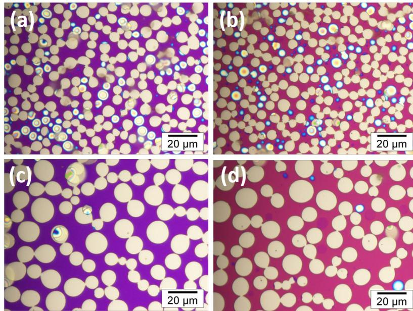
Fig. 8.12: Optical micrographs(100X magnification) of samples after 40 W argon pretreatment followed by anneal at (a) 550°C (b) 800°C and 100 W argon pretreatment after anneal at (c) 550°C (d) 800°C.
