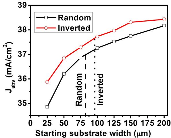
Fig. 8.1:  $J_{abs}$  versus starting wafer thickness for random and inverted pyramidal texturing. Also indicated (dotted lines) are  $J_{abs}$  after random and inverted texturing for a 100  $\mu\text{m}$  thick wafer.
