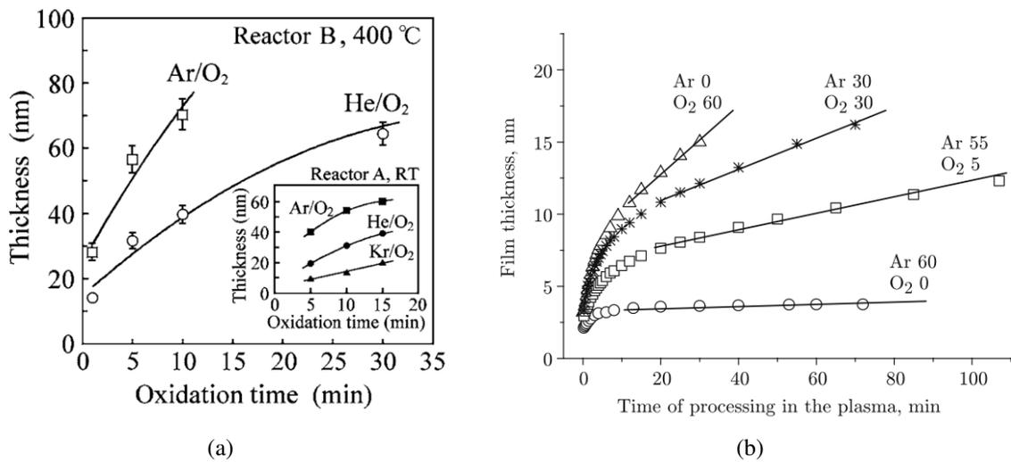
Fig. 2.8: (a) Oxidation in atmospheric pressure plasma chamber [82] (b) Oxidation rate for different O<sub>2</sub>/Ar ratios[83].
