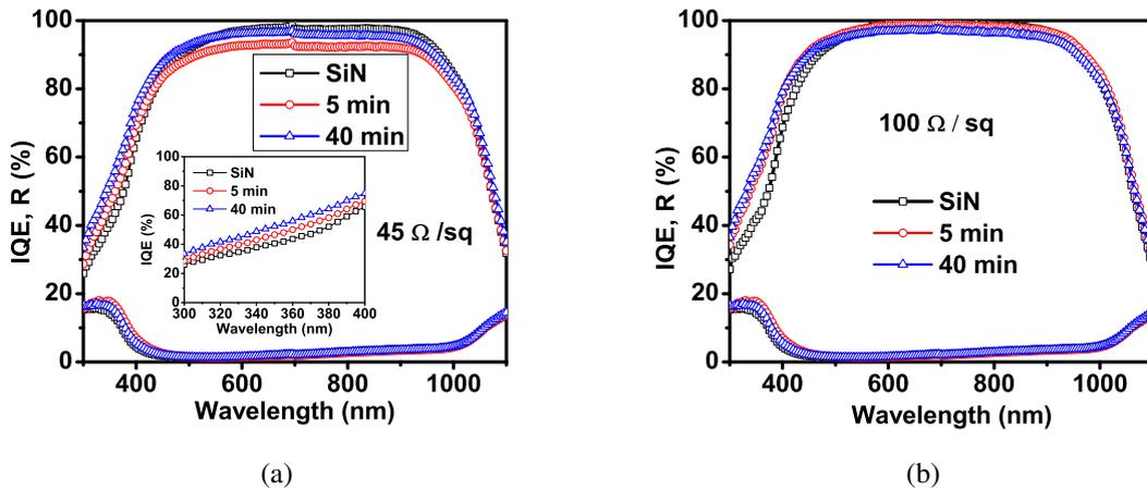
Fig. 6.10: IQE and reflectance curves for two sets of solar cells with different emitter sheet resistances (a)  $45 \Omega/\square$  emitter (b)  $100 \Omega/\square$  emitter.
