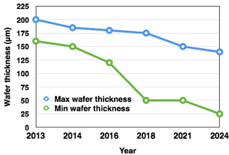
Fig. 1.2: Predicted maximum and minimum wafer thickness in coming years, data adapted from [3].
