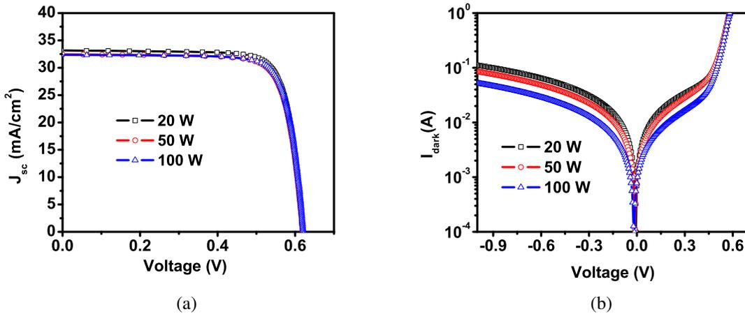
Fig. 6.26: (a) Illuminated and (b) dark IV characteristics for solar cells fabricated with different silicon nitride films.
