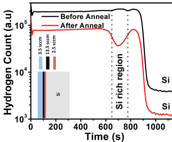
Fig. 8.9: TOF - SIMS data for a trilayer silicon nitride stack deposited by varying the silane flow rate (inset) showing a decrease in hydrogen count upon annealing. The decrease in H count was drastic in the Si rich SiN region, indicating the weak nature of Si - H bonds.
