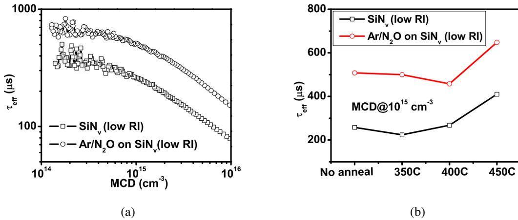
Fig. 7.9: (a)  $\tau_{eff}$  enhancement observed for plasma treated single layer silicon nitride film (b) Variation in  $\tau_{eff}$  for different annealing temperatures for plasma treated single layer silicon nitride ( $\text{SiN}_v$ ) film.  $\tau_{eff}$  was measured on 300  $\mu\text{m}$  thick n-type FZ wafers with a resistivity of 3  $\Omega\text{ cm}$ .
