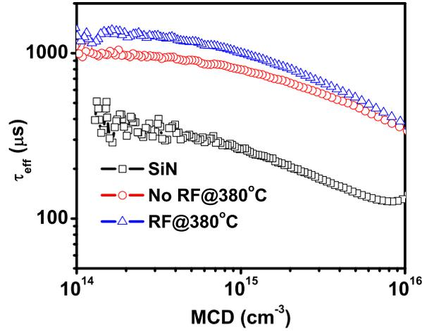
Fig. 7.11:  $\tau_{eff}$  measurement on n-type FZ wafers, before and after plasma (RF) treatment. No RF corresponds to the sample kept in the chamber without turning ON the RF supply.
