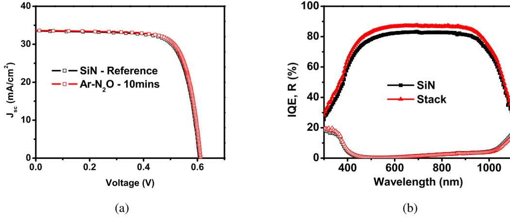
Fig. 6.15: (a) Illuminated IV and (b) internal quantum efficiency for solar cells fabricated with  $\text{SiO}_x\text{N}_y - \text{SiN}_v:\text{H}$ .
