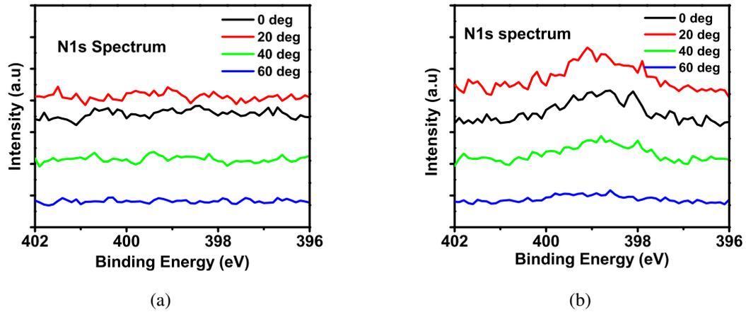
Fig. 5.14: ARXPS N1s spectrum for films grown in (a)  $N_2O$  and (b)  $N_2O + NH_3$  ambient. Presence of nitrogen is seen for sample grown in  $N_2O + NH_3$  plasma ambient.
