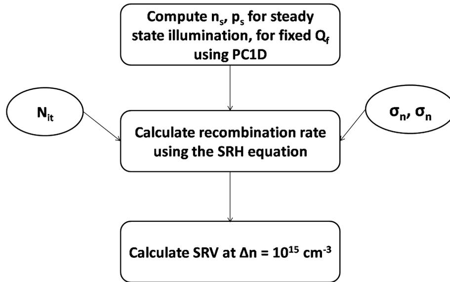
Fig. A.1: Flow chart for simulating impact of  $N_{it}$  and  $Q_f$  on  $S_{eff}$ .
