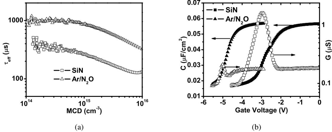
Fig. 7.4: (a) Improvement in  $\tau_{eff}$  following Ar + N<sub>2</sub>O plasma treatment of silicon nitride film.  $\tau_{eff}$  measured on n-type FZ wafers (b) HFCV curves (closed symbols) and HFGV curves (open symbols) before and after plasma treatment. A significant improvement in  $\tau_{eff}$  and a sharp reduction in  $D_{it}$  can be observed from the HFCV curves.
