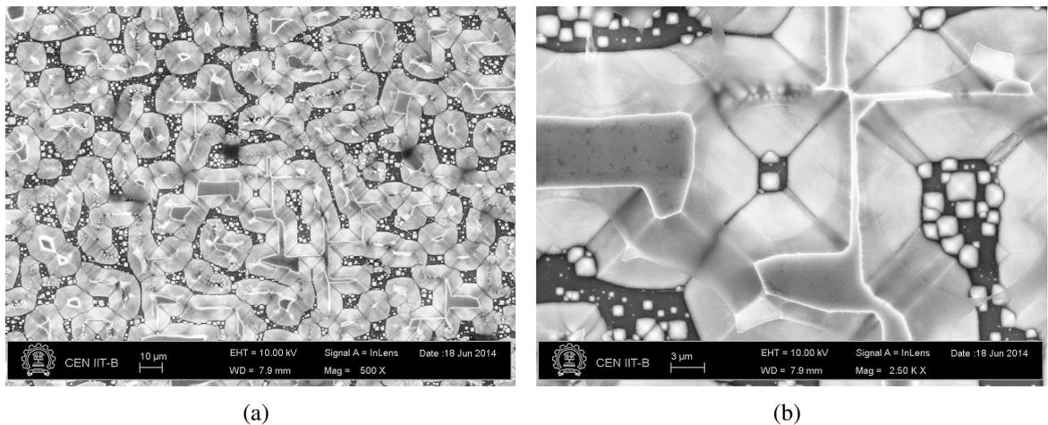
Fig. 8.13: SEM images (a) showing the formation of inverted pyramids after etching the sample in TMAH solution for 5 min (b) Magnified image showing an inverted pyramid, the undercut as a result of etching through the blister can also be seen. The sample prepared with 100 W Ar plasma pretreatment and annealed at 550°C was used for the experiment.
