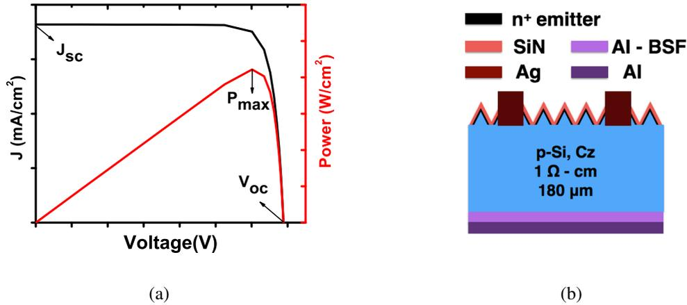
Fig. 4.4: (a) IV and PV curve of a solar cell (b) schematic of a screen printed p-type silicon solar cell used for experiments.
