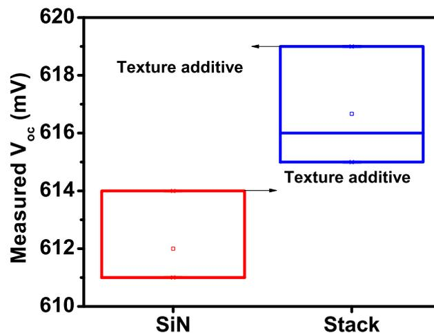
Fig. 6.20: Improvement in  $V_{oc}$  for the stack across different solar cell batches.
