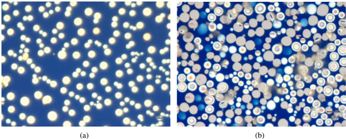
Fig. 8.11: Increase in blister coverage for increasing anneal duration (a) 2 s (b) 10 s. The samples were annealed at  $800^{\circ}\text{C}$  in  $\text{N}_2$  ambient in a RTP chamber.
