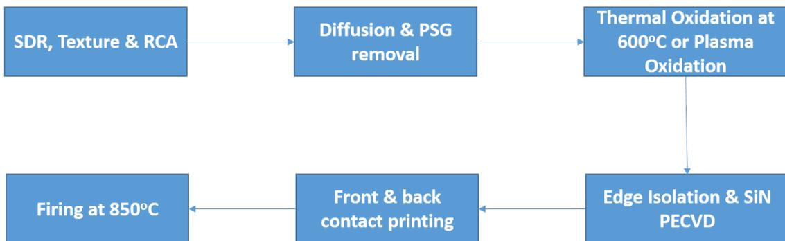
Fig. 6.17: Process flow used for solar cell fabrication.
