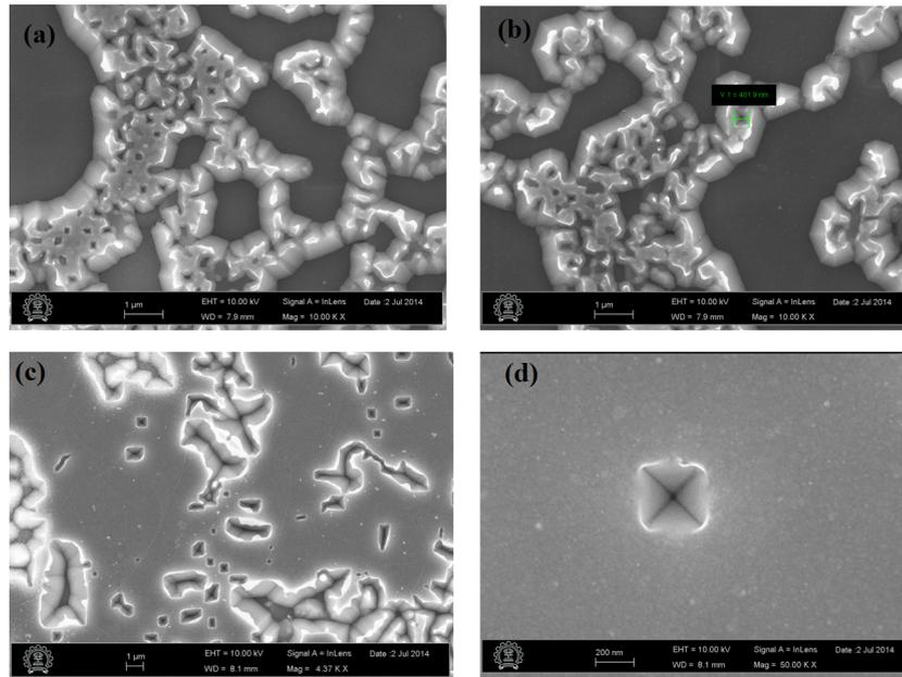
Fig. 8.18: SEM images after etching in TMAH showing the nano pyramids at different regions on the wafer.
