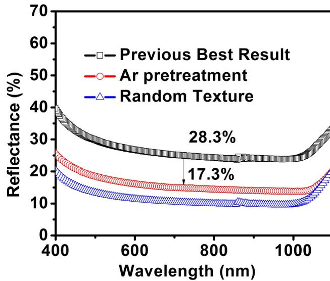
Fig. 8.14: Reflectance values showing a decrease in weighted average reflectance from 28.3% to 17.3%, owing to an increased surface coverage of open blisters as result of Ar pretreatment.  $W_{av}$  reflectance of 17.3% was obtained for the sample prepared with 100 W Ar plasma pretreatment and annealed at 550°C was used for the experiment. Previous best results refers to the results presented in Fig. 8.4.
