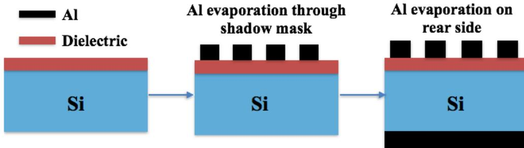
Fig. 4.2: Process flow for fabricating MIS capacitors.
