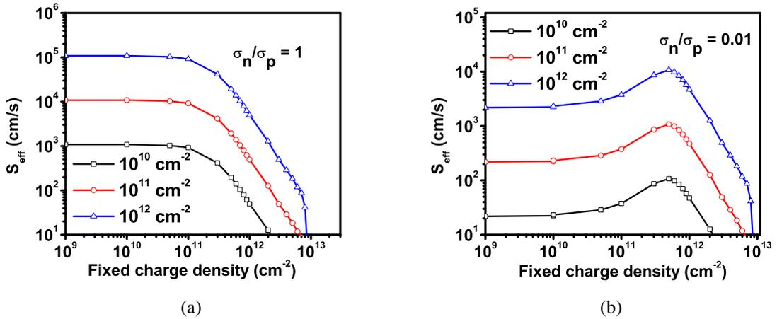
Fig. 2.2: Impact of  $N_{it}$  and positive  $Q_f$  on  $S_{eff}$  for two different capture cross section ratios (a)  $\sigma_n/\sigma_p = 1$  (b)  $\sigma_n/\sigma_p = 0.01$  on n - type wafer with  $\tau_{bulk} = 1 \text{ ms}$ .
