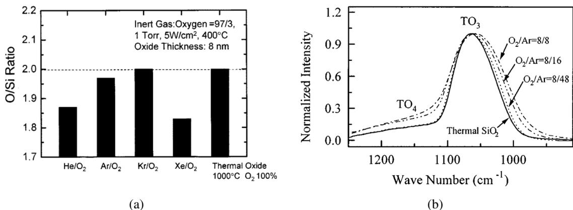
Fig. 2.9: (a) O/Si ratio from XPS measurements [14] (b) FTIR spectrum showing Si - O - Si vibrations for different O<sub>2</sub>/Ar ratios [84].
