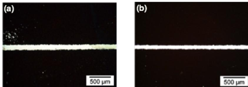
Fig. 7.1: (a) Background plating observed in untreated sample after Ni - Cu plating (b) Reduction in background plating in plasma treated sample after Ni - Cu plating[19].
