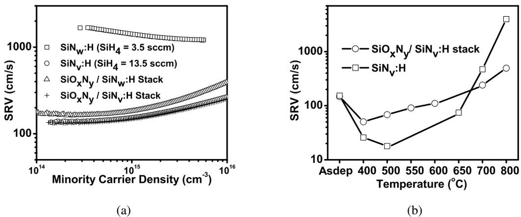
Fig. 5.11: (a) SRV for various silicon nitride layers and corresponding stacks (b) Thermal stability of stack compared with silicon nitride.
