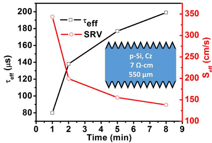
Fig. 7.8: Variation in  $\tau_{eff}$  for different plasma exposure durations for a p-type Cz wafer.
