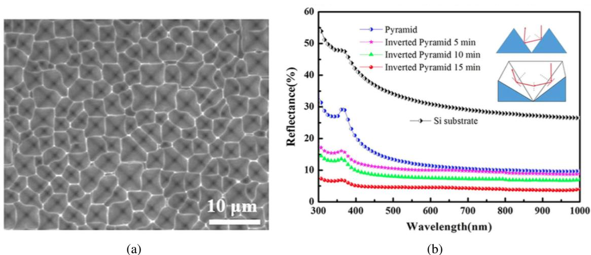
Fig. 3.7: Maskless inverted pyramid fabrication using  $\text{Cu}(\text{NO}_3)_2/\text{HF}/\text{H}_2\text{O}_2/\text{H}_2\text{O}$  as etch solution (a) Inverted pyramids after etching in solution (b)  $W_{av}$  reflectance for different time durations compared with random texturing process. [108].
