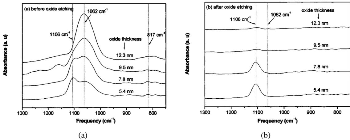
Fig. 2.10: FTIR spectrum for plasma grown oxide films of different thickness (a) before and (b) after etching in HF solution [85].
