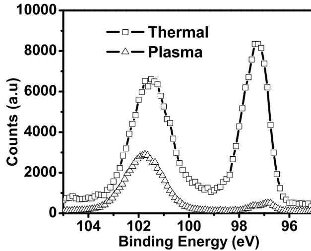
Fig. 6.18: Si2p spectrum for thermal and plasma grown films.
