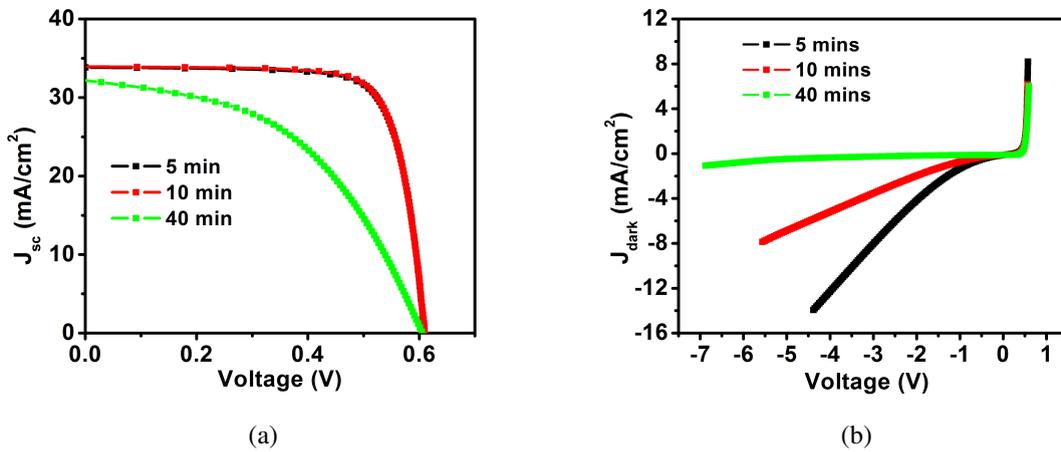
Fig. 6.23: (a) Illuminated and (b) dark IV characteristics of solar cells fabricated with  $\text{SiO}_x\text{N}_y - \text{SiN}_v:\text{H}$ .
