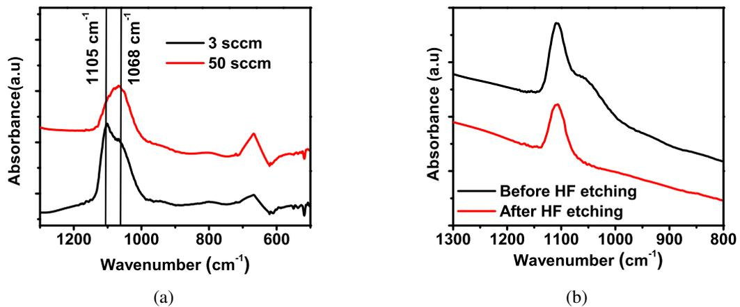
Fig. 5.18: (a) FTIR spectra comparing films grown at 3 sccm and 50 sccm  $N_2O$  flow rates. Time of growth was 10 min. Lower interstitial O content is observed for the 50 sccm sample (b) FTIR spectrum measured before and after removing the plasma grown film in 2% HF solution, confirming the trapping of interstitial oxygen within silicon.
