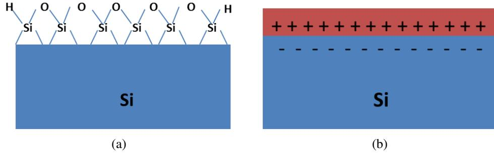
Fig. 2.1: Schematic representation of two surface passivation mechanisms (a) Chemical passivation (b) Field effect passivation
