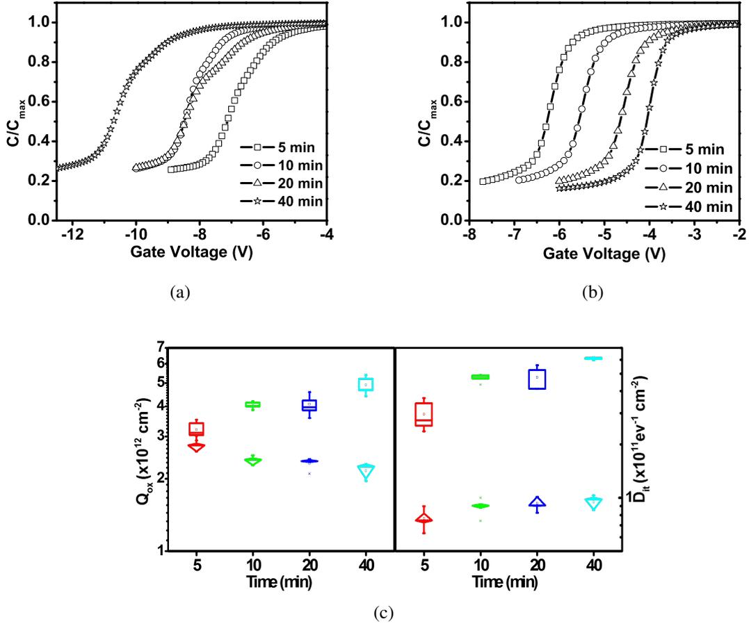
Fig. 6.6: HFCV curves for  $\text{SiO}_x\text{N}_y$  -  $\text{SiN}_v\text{:H}$  stacks (a) before firing (b) after firing (c)  $Q_{ox}$  and  $D_{it}$  versus plasma exposure time before ( $\square$ ) and after firing( $\diamond$ ).
