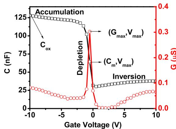
Fig. 4.3: HFCV and HFGV for an MIS capacitor on a p-type Si substrate.
