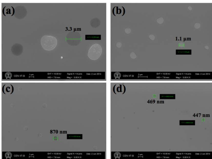
Fig. 8.16: SEM images showing the blister formation in a silicon nitride film as its thickness was reduced by etching it in BHF solution. For increasing etch durations (a) 0 s (b) 30 s (c) 60 s (d) 90 s, the size of the blisters came down from  $3\ \mu\text{m}$  to 450 - 470 nm.
