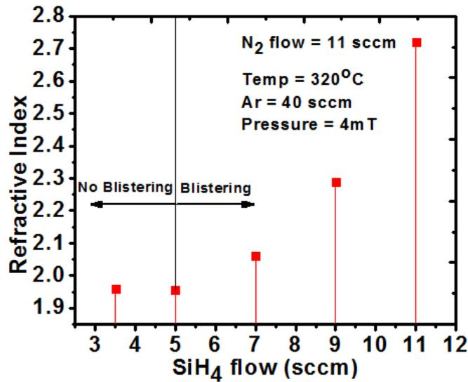
Fig. 8.7: Variation in RI with changing silane flow. The threshold silane flow rate beyond which blistering commences is also shown in figure.
