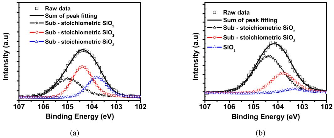
Fig. 5.13: Si2p XPS spectrum for films grown in (a)  $N_2O$  and (b)  $N_2O + NH_3$  ambient. A large amount of sub - stoichiometric phases of silicon oxide can be seen for both the films.
