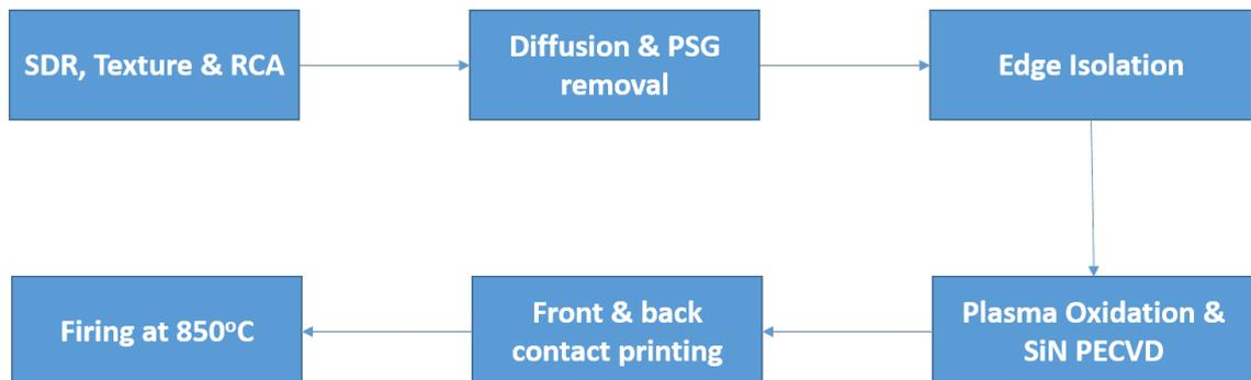
Fig. 6.2: Solar cell process flow.
