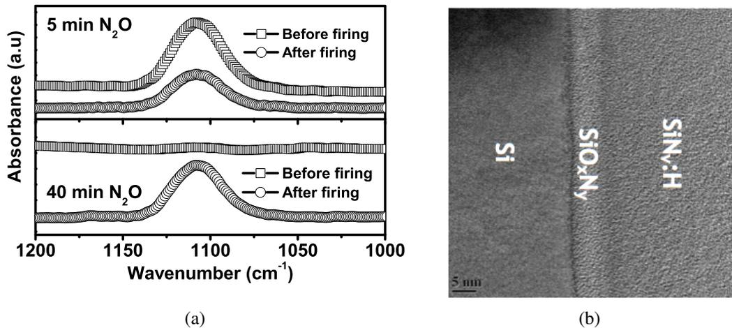
Fig. 6.5: FTIR measurements carried out on Si wafer after stripping the as deposited and fired  $SiO_xN_y - SiN_v:H$  stacks in buffered HF solution. A significant increase in peak at  $1105\text{ cm}^{-1}$  is seen for 40 min sample, after firing (b) HRTEM image of a (10 min)  $SiO_xN_y - SiN_v:H$  stack.
