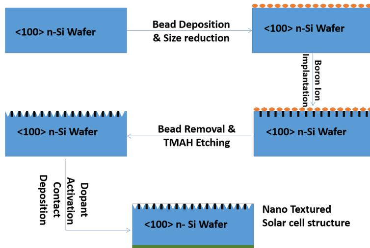
Fig. 8.17: Process flow for nano texturing of silicon using boron etch stop layer.
