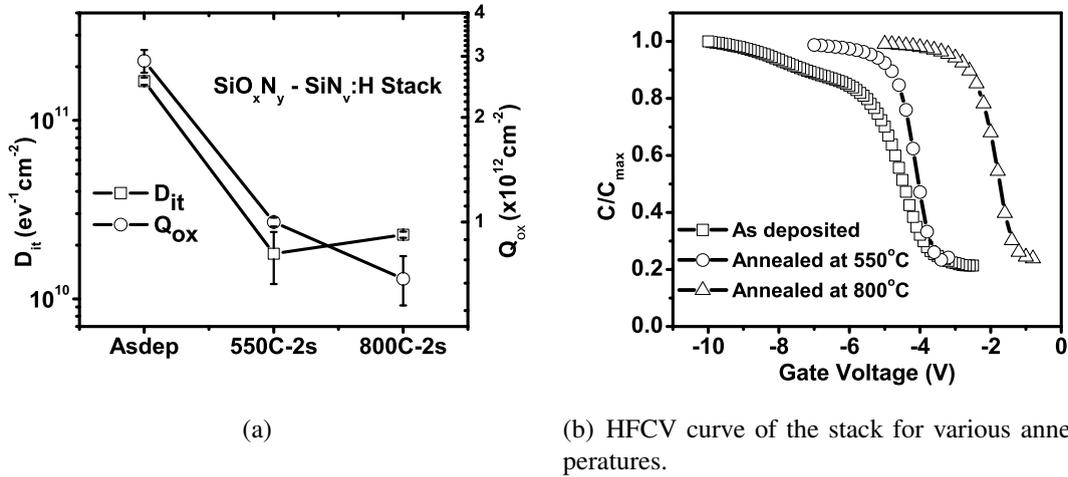
Fig. 5.10: HFCV Analysis of silicon oxy-nitride - silicon nitride stack at different annealing temperatures (a) Variation in  $D_{it}$  and  $Q_f$  for the stack and (b) respective HFCV curves.
