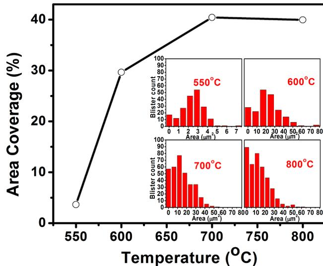
Fig. 8.10: Variation in blister coverage with increasing anneal temperature. Inset shows the distribution of blisters of different areas for varying anneal temperatures. Blister count is given as a percentage of the total number of blisters. The area used for the analysis was 140 μm x 105 μm.
