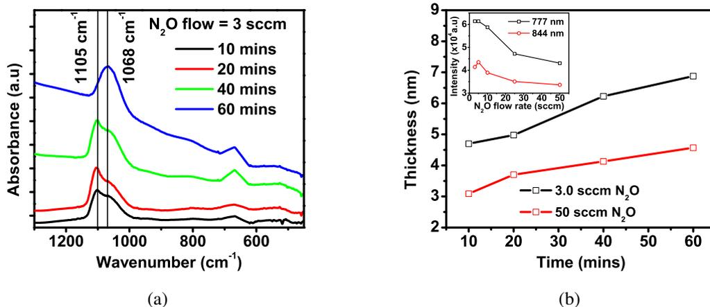
Fig. 5.17: (a) FTIR spectra for films grown in 3 sccm N<sub>2</sub>O flow rate showing a decrease in interstitial oxygen at 1105 cm<sup>-1</sup> for longer oxidation time (b) Ellipsometry data showing thickness versus growth duration for films grown in 3 sccm and 50 sccm N<sub>2</sub>O flow. Inset shows the O line intensities measured using OES, higher O line intensity is observed for plasma struck at lower flow rates
