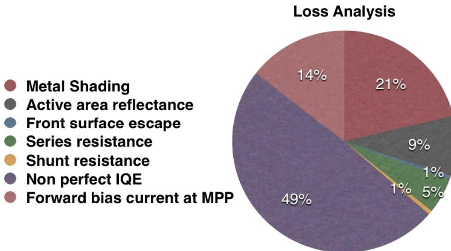
Fig. 6.21: Loss analysis carried out on the 16.4% solar cell. Non perfect IQE is seen to contribute close to 50% of the total loss in the solar cell under investigation.
