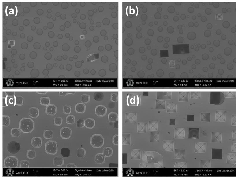
Fig. 8.3: (a), (b) SEM images of a sample with large density of unopened blisters after etching in TMAH solution for 1 min and 5 min respectively. No etching was observed under the unopened blister. (c), (d) SEM images of a sample with a large density of open blisters after etching in TMAH solution for 1 min and 5 min respectively. Etching can be seen to commence along the blister edges after 1 min and fully formed inverted pyramids can be seen after 5 min of etching.
