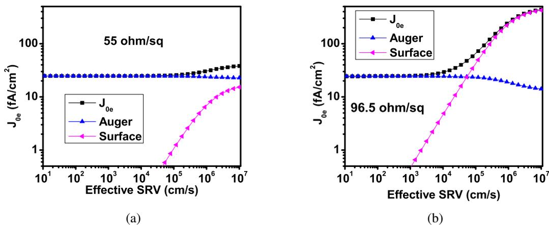
Fig. 6.22: Impact of surface SRH on different emitter sheet resistances (a) 55  $\Omega/\square$  (b) 100  $\Omega/\square$ .
