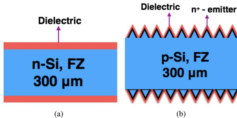
Fig. 4.1: Device schematic used for (a)  $\tau_{eff}$  measurement (b)  $J_{0e}$  measurement.
