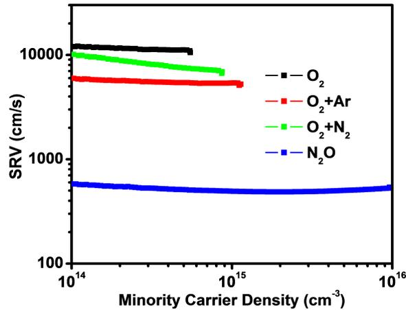
Fig. 5.7: SRV variation across samples after firing the stacks at  $800^\circ\text{C}$ .
