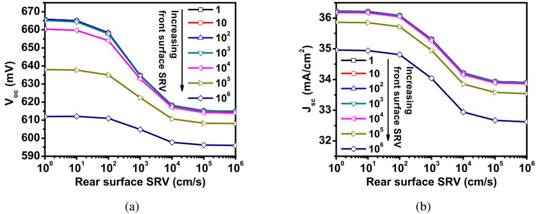
Fig. 2.4: PC1D simulation results showing the impact of front and rear surface recombination velocities (a) open circuit voltage (b) short circuit current density. The impact of surface recombination velocity (front and rear) is seen to be more dramatic on the open circuit voltage than on short circuit current density.
