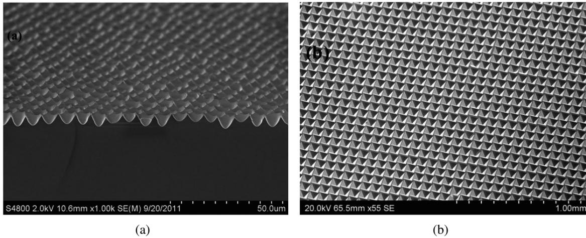
Fig. 3.4: Alternate surface texturing schemes demonstrated on  $\langle 100 \rangle$  wafers (a) Laser texturing of silicon [45] (b) Inverted pyramidal texturing using inkjet printing [8].
