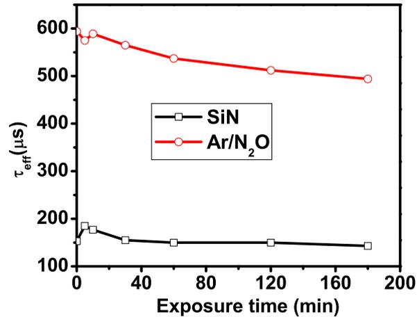
Fig. 7.6: Reduction in  $\tau_{eff}$  following UV exposure. For longer duration,  $\tau_{eff}$  can be seen to saturate.  $\tau_{eff}$  was measured on 300  $\mu$ m thick n-type FZ wafers with a resistivity of 3  $\Omega$  cm.
