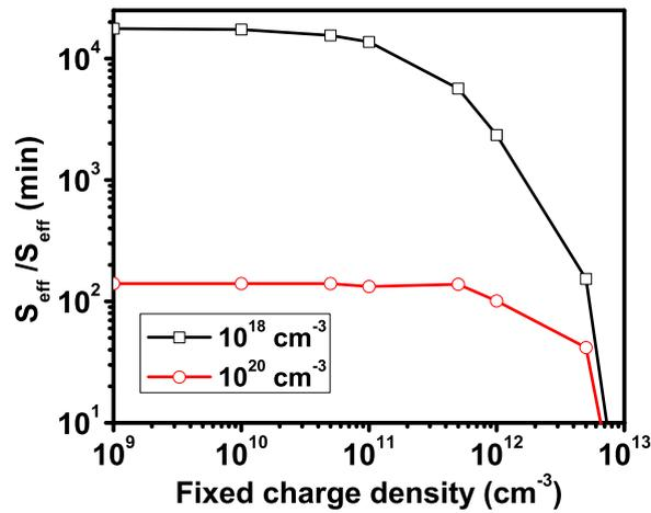
Fig. 2.3:  $S_{eff}$  normalised with  $S_{eff}(\text{min})$  for two different doping densities.  $N_{it}$  of  $10^{10} \text{ cm}^{-2}$  and  $\sigma_n/\sigma_p = 1$  was assumed for this simulation.
