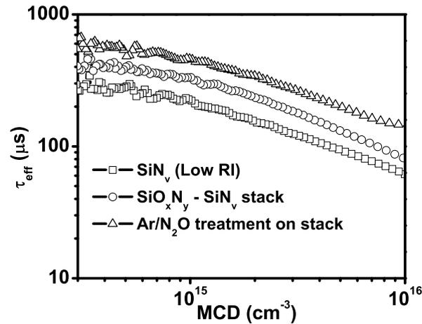
Fig. 7.13:  $\tau_{eff}$  improvement as a result of plasma pre and post treatment; measured on n-type FZ wafer.
