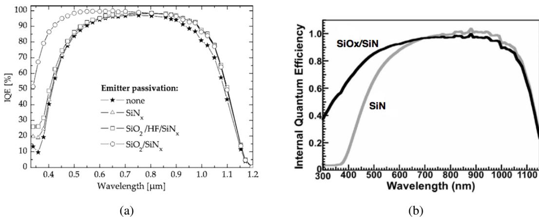
Fig. 2.5: (a), (b) IQE for n-type Si solar cells with wet chemical grown SiO<sub>2</sub>/PECVD SiN<sub>x</sub> films used for emitter surface passivation [73, 74]
