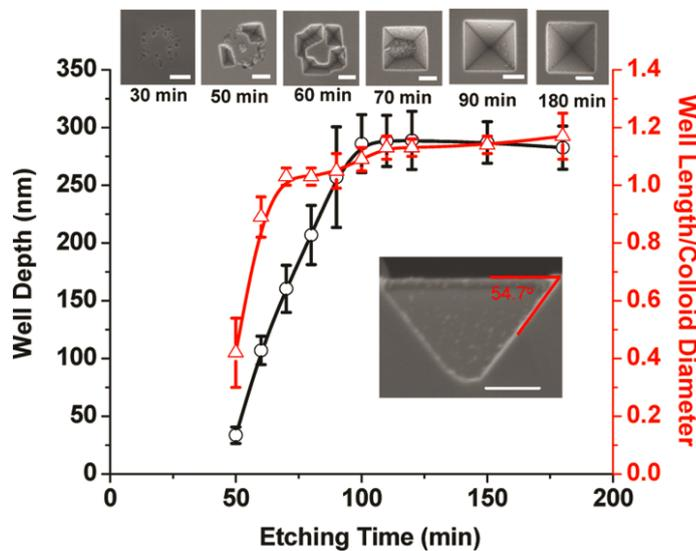
Fig. 3.6: Etched depth (well depth) versus etching time, indicating a large amount of etch for longer etch durations; inset shows the SEM images showing the evolution of the pyramids with time [105].
