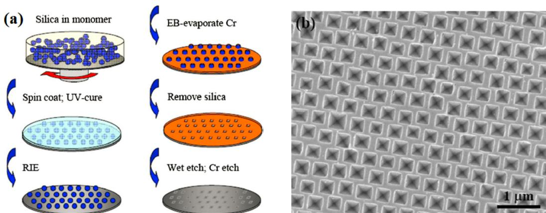
Fig. 3.5: (a) Process flow for fabricating inverted pyramids using colloidal lithography (b) Inverted pyramids fabricated using technique mentioned in (a) [103].
