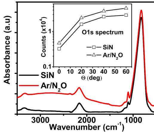
Fig. 7.3: FTIR spectrum showing no significant change in Si - H or N - H bond intensity following plasma treatment. Inset shows ARXPS O1s spectrum showing an increase in O-count after Ar + N<sub>2</sub>O plasma post treatment.
