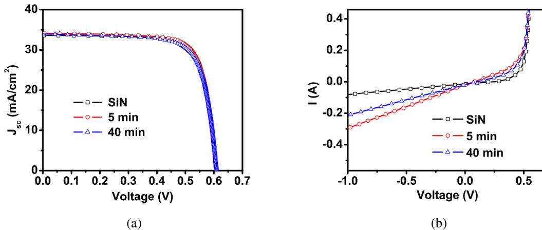
Fig. 6.9: (a) Illuminated and (b) dark IV curves for solar cell with and without plasma grown  $\text{SiO}_x\text{N}_y$  film.
