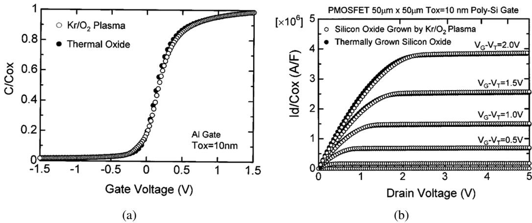
Fig. 2.11: (a) HFCV characteristics of MOS capacitor with Al gate (b) IV characteristics of p-MOS transistor [14].
