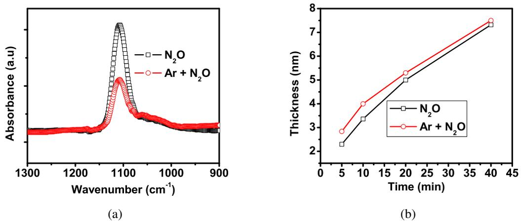
Fig. 6.13: (a) FTIR spectrum and (b) ellipsometry data comparing films grown in  $N_2O$  and  $Ar + N_2O$  ambient for 5 min.
