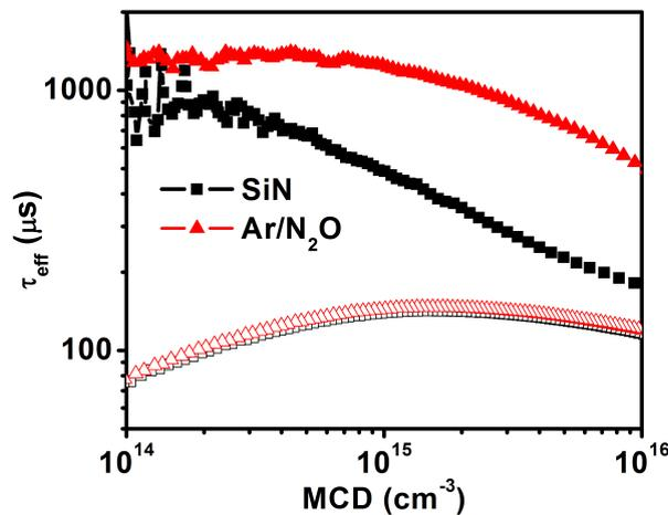
Fig. 7.5: Thermal stability of surface passivation quality for two different annealing conditions. Closed symbols represent 450°C anneal in furnace typically used for Ni - Cu contact sintering, while open symbols represent 850°C firing in RTA typically used for screen printed silver contacts.
