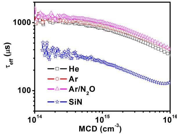
Fig. 7.10: Enhancement in  $\tau_{eff}$  for different plasma ambient. No significant difference in  $\tau_{eff}$  was seen for treatment in different plasma ambients.  $\tau_{eff}$  was measured on 300  $\mu\text{m}$  thick n-type FZ wafers with a resistivity of 3  $\Omega\text{ cm}$ .
