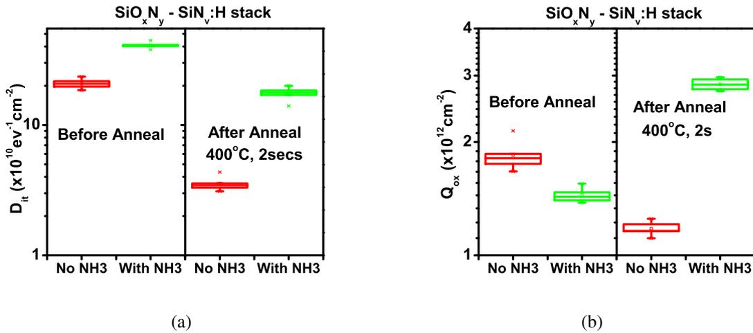
Fig. 5.15: Variation in (a)  $D_{it}$  and (b)  $Q_f$  for  $SiO_xN_y - SiN_v:H$  stacks before and after annealing at  $400^\circ C$ .
