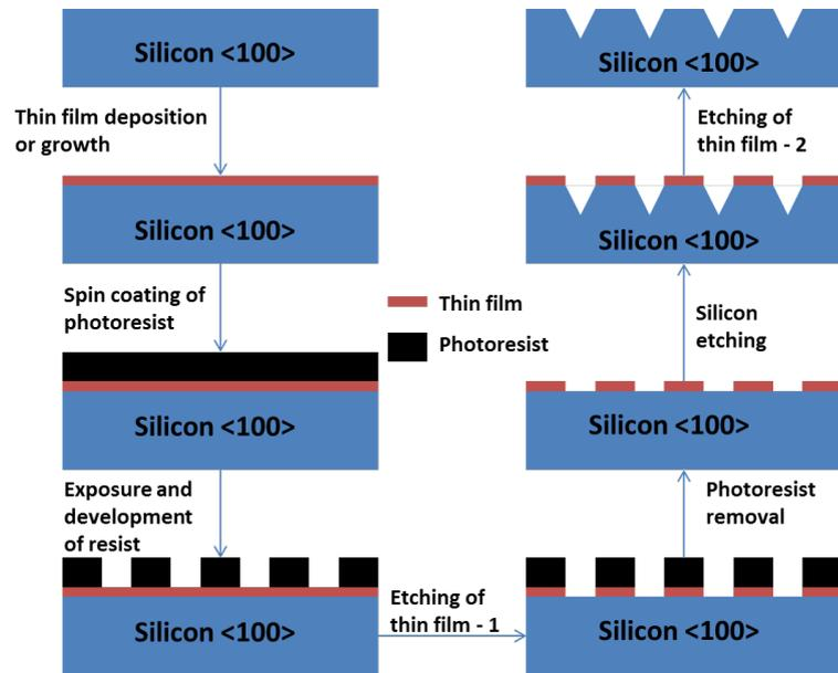
Fig. 3.2: Process flow for fabrication of inverted pyramids in crystalline silicon, adapted from [9].
