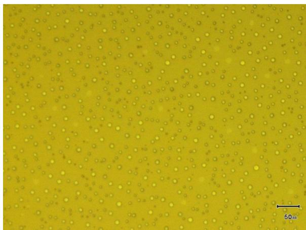
Fig. 8.15: Optical image showing small blisters in a thin silicon nitride film of thickness 18 nm.
