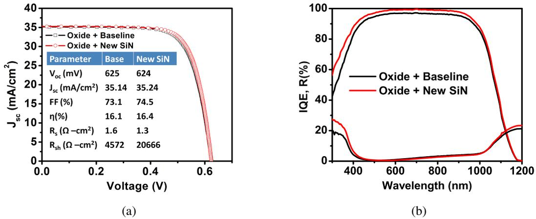
Fig. 6.27: (a) Illuminated IV characteristics for solar cells fabricated with two different silicon nitride films. A higher  $R_{sh}$  and  $J_{sc}$  was observed for the new SiN film (b) IQE curves indicating a better passivation quality for the newly developed SiN film as compared to the baseline silicon nitride film.
