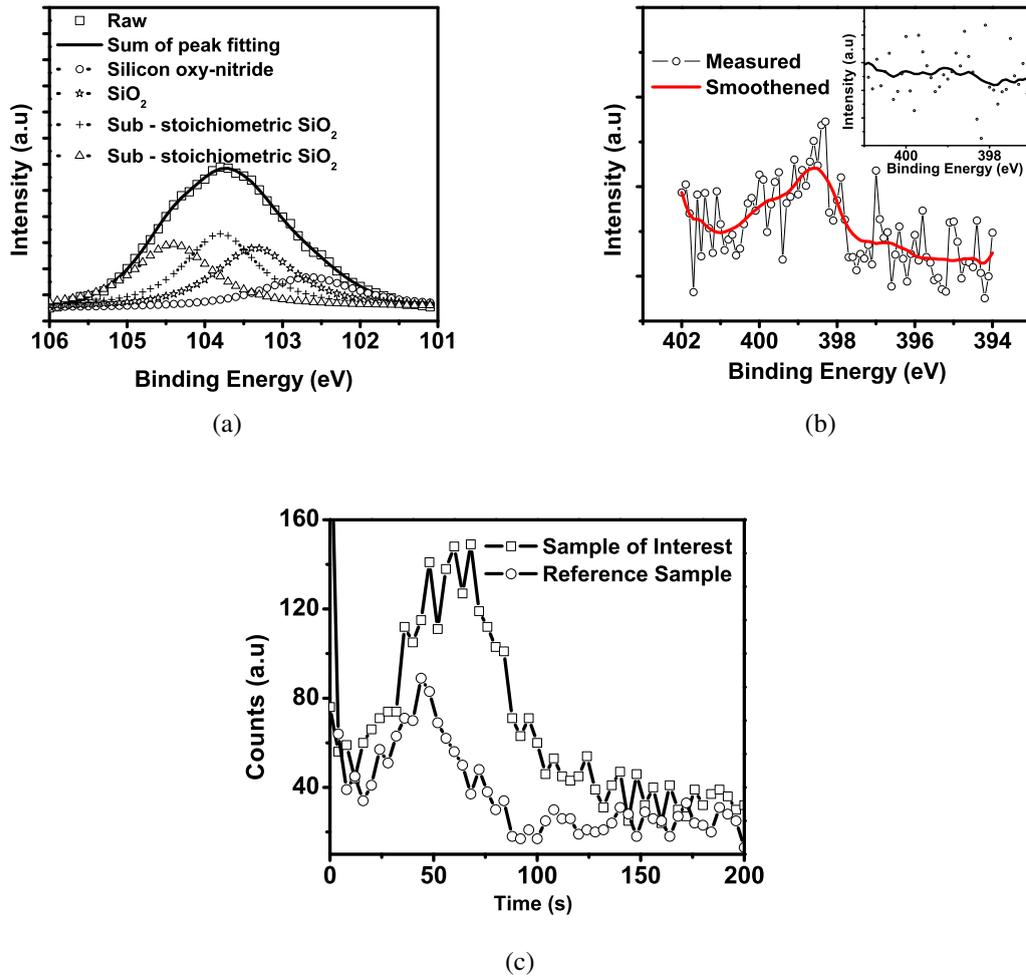
Fig. 5.9: Physical characterisation of the plasma grown film (a) Si<sub>2p</sub> XPS spectrum showing different oxide phases as well as oxy-nitride phase (b) N<sub>1s</sub> XPS spectrum showing raw and smoothed data, inset shows N<sub>1s</sub> spectrum for a film without nitrogen (c) SIMS profile showing nitrogen counts for plasma grown film.
