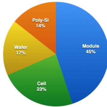
Fig. 1.1: Various components of module cost, data adapted from [3].
