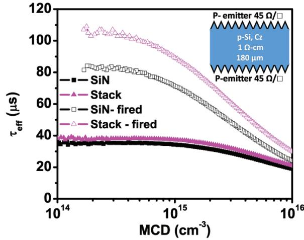
Fig. 6.16: Lifetime measurement on double side P-diffused p-type Cz wafers, before and after firing. Inset shows the test structure used for the measurement.
