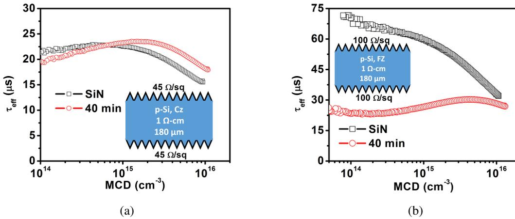
Fig. 6.11: Lifetime measurements on double side diffused emitters after firing at 850°C (a) 45 Ω/□ emitter on Cz wafer (b) 100 Ω/□ emitter on FZ wafer.
