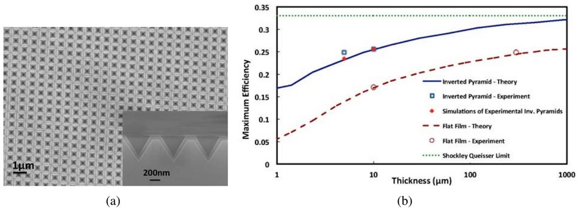
Fig. 3.3: Potential of nano texturing on ultra thin silicon wafers (a) Inverted nano pyramids fabricated on silicon using immersion lithography (b)  $5\ \mu\text{m}$  thick wafer shows an equivalent performance as compared to a  $300\ \mu\text{m}$  thick wafer [98].
