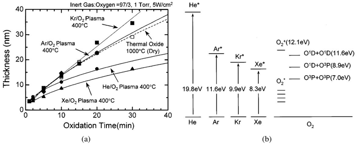
Fig. 2.7: (a) Growth rate in inert gas - oxygen mixture (b)Energy diagram of inert gas and oxygen [14].
