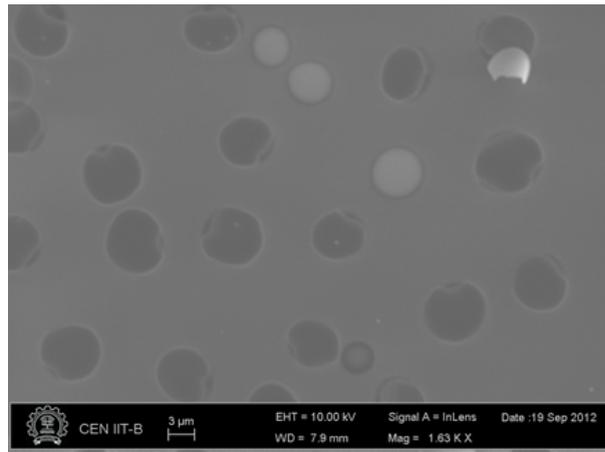
Fig. 8.5: Electron microscopy image showing the blister formed in silicon nitride film after annealing at 800°C for 2 s. Some of the blisters had fully cracked open, while some did not.
