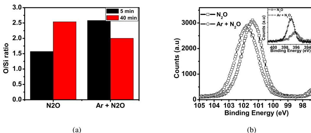
Fig. 6.14: (a) O/Si ratio for various oxidation times in  $N_2O$  and  $Ar + N_2O$  ambient (b) Si2p spectrum for  $N_2O$  and  $Ar + N_2O$  oxidation for 40 min, inset shows N1s spectrum.
