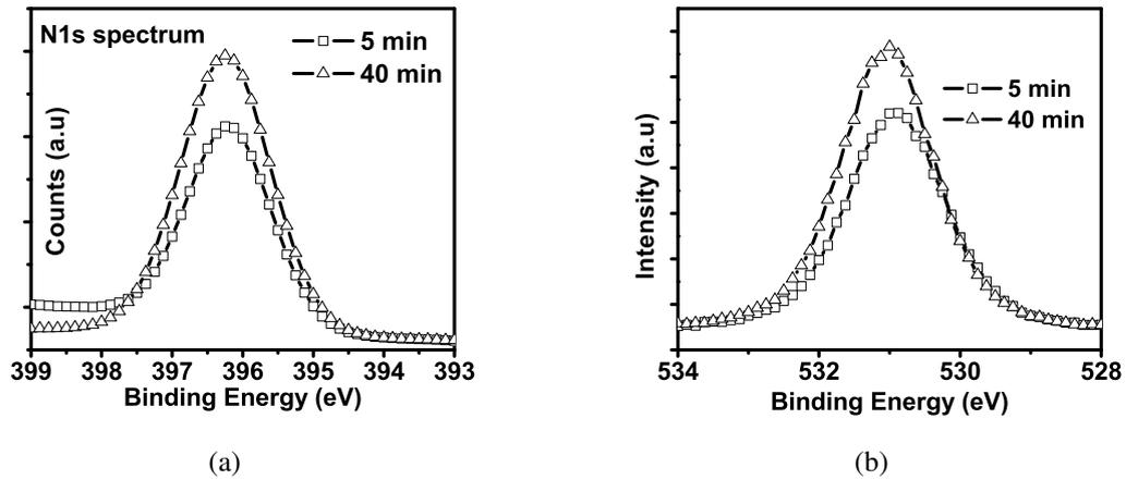
Fig. 6.3: Physical characterisation of  $\text{N}_2\text{O}$  plasma grown films on Si (a)  $\text{N}1s$  XPS spectrum for  $\text{SiO}_x\text{N}_y$  film grown in  $\text{N}_2\text{O}$  ambient for 5 min and 40 min confirming presence of nitrogen (b)  $\text{O}1s$  XPS spectrum showing larger oxygen content for films grown for 40 min.
