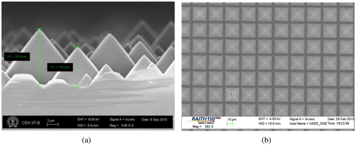
Fig. 3.1: Two different surface texturing schemes demonstrated on  $\langle 100 \rangle$  wafers (a) Random pyramidal texturing (b) Inverted pyramidal texturing.
