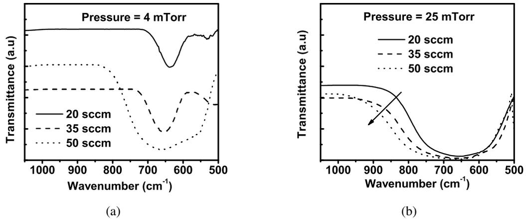
Fig. 5.8: FTIR spectrum at two different chamber pressures (a) 4 mTorr (b) 25 mTorr showing the variation in film composition with change in  $\text{N}_2\text{O}$  gas flow rates.
