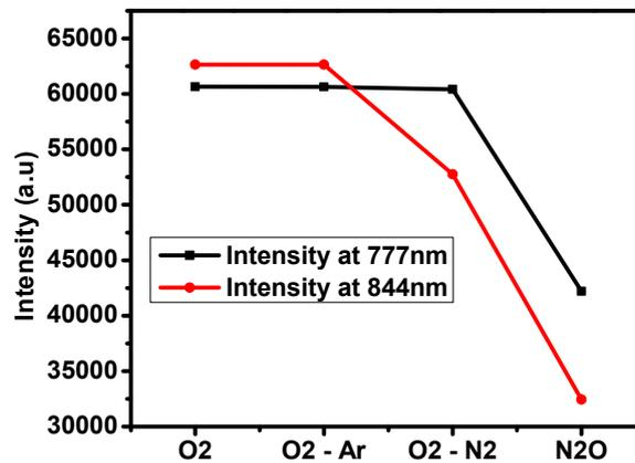
Fig. 5.3: Comparison of oxygen line intensities for different plasma ambient, showing a lower atomic oxygen content for  $\text{N}_2\text{O}$  plasma.
