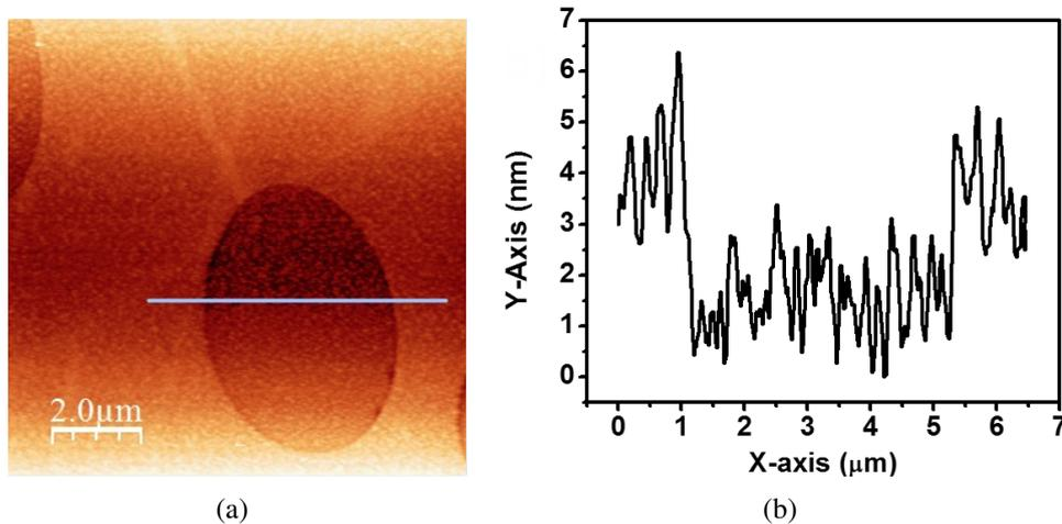
Fig. 8.6: (a) AFM image on silicon surface after removing silicon nitride film (b) Surface profile along the line shown in (a) indicates pit formation in silicon under the blisters.
