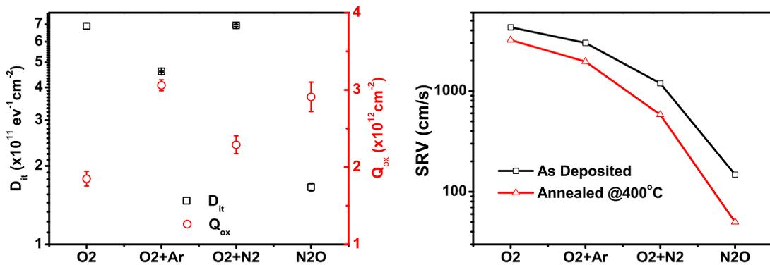
Fig. 5.6: Electrical Characteristics of film grown in different ambient.
