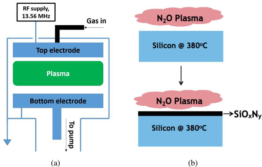
Fig. 6.1: (a) Schematic of PECVD system and (b) plasma oxidation process.
