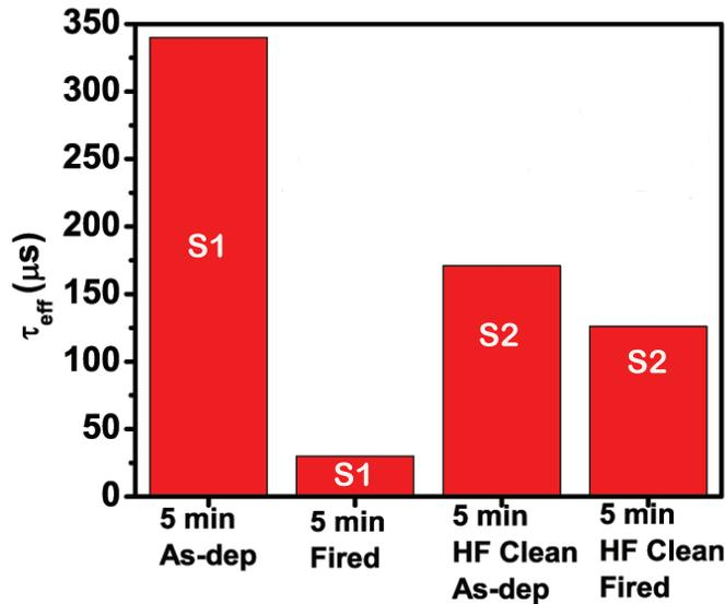
Fig. 6.8: Lifetime data on samples measured before and after firing. The samples differ in the fact that the plasma grown  $\text{SiO}_x\text{N}_y$  layer was etched out in 2% HF solution. After firing, a significant degradation in  $\tau_{eff}$  can be seen, when the  $\text{SiO}_x\text{N}_y$  layer is present during firing process.
