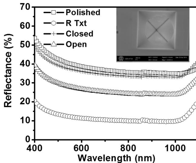
Fig. 8.4: Reflectance curves for textured samples showing a decrease in reflectance in comparison to polished silicon. No anti-reflective coating was used on the samples. Also shown is the reflectance curve for a commercial random texturization(R Txt) process for reference. Inset shows the undercut observed during etching through a blister.
