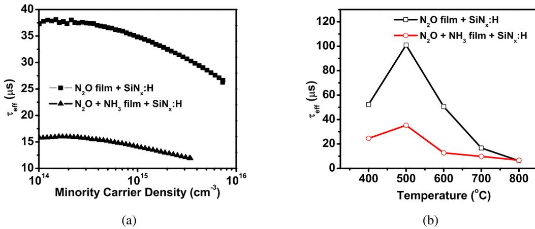
Fig. 5.16: (a)  $\tau_{eff}$  for the  $SiO_xN_y$  -  $SiN$  stack before annealing. Higher  $\tau_{eff}$  observed for films grown in  $N_2O$  plasma ambient (b) Variation in  $\tau_{eff}$  for  $SiO_xN_y$  -  $SiN$  stack for different annealing conditions.  $\tau_{eff}$  was measured on 300  $\mu m$  thick n-type FZ wafers with a resistivity of 3  $\Omega$  cm.
