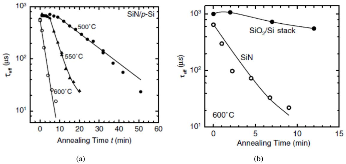
Fig. 5.1: (a) Thermal degradation of silicon nitride film on annealing (b) Improved thermal stability of  $\text{SiO}_2$  -  $\text{SiN}$  stack [51].
