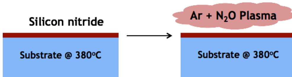
Fig. 7.2: Schematic of the plasma post treatment process of silicon nitride.
