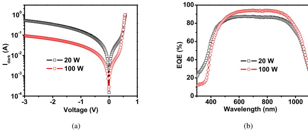
Fig. 6.25: (a) Dark IV and (b) external quantum efficiency for solar cells fabricated with two different silicon nitride films.
