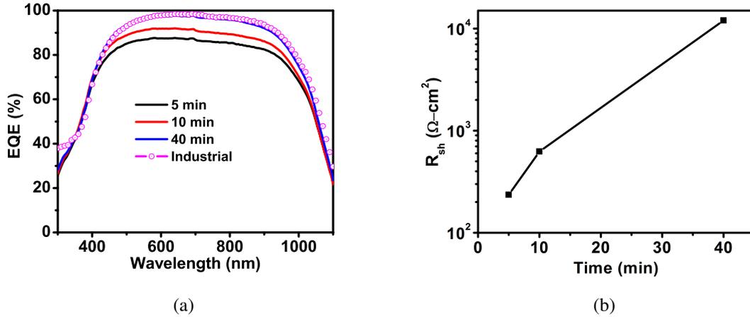
Fig. 6.24: (a) External quantum efficiency of solar cells fabricated with  $\text{SiO}_x\text{N}_y - \text{SiN}_v\text{:H}$  for varying oxidation durations (b) Improvement in  $R_{sh}$  for increasing oxidation time.
