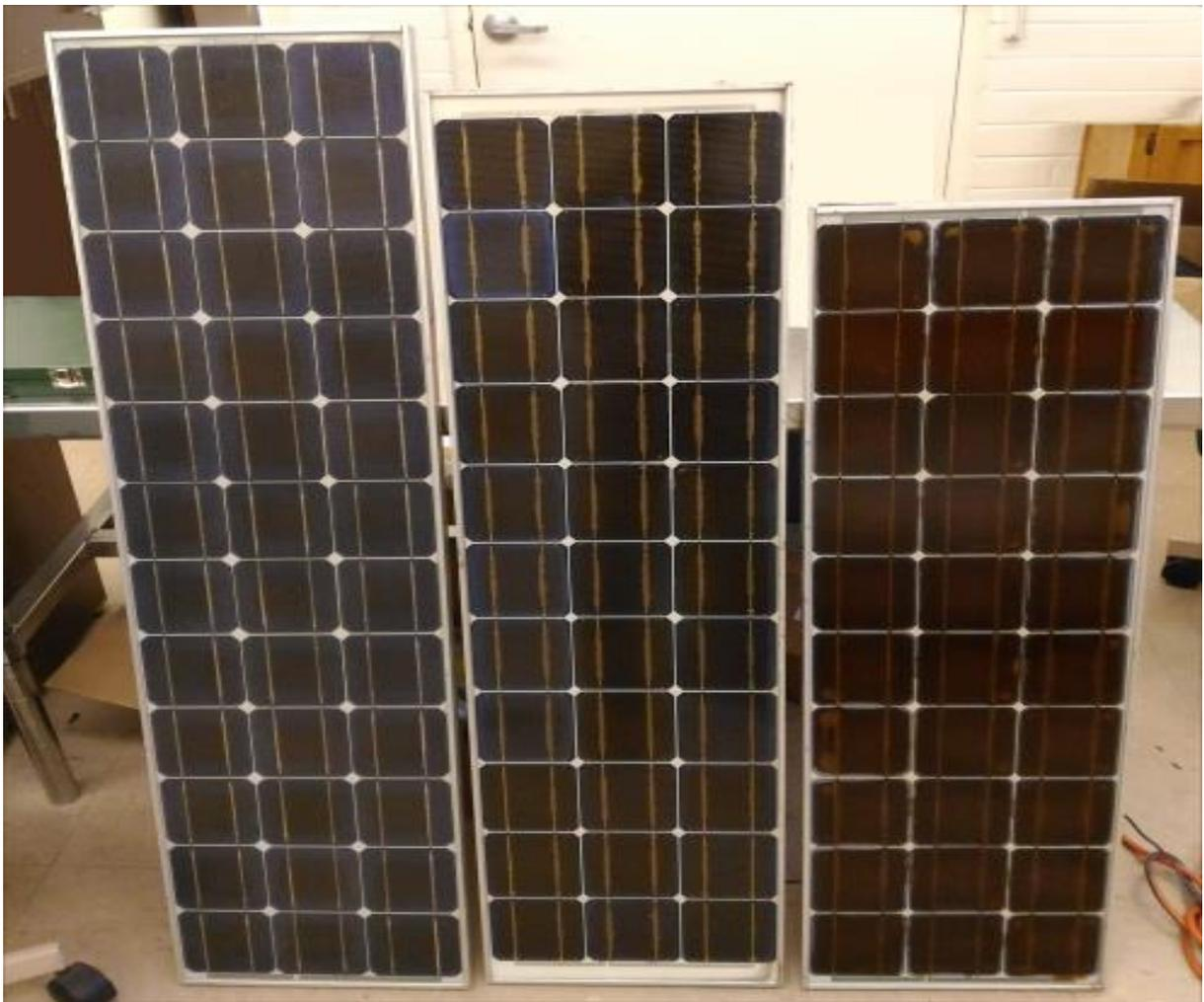
Fig. 5.1: Discolored PV modules used for discoloration study during internship at Arizona State University – Photovoltaic Reliability Laboratory.
