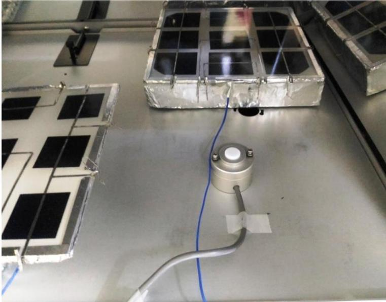
Fig. 7.4: Measurement of the irradiance at the position of the solar cells of sample UVC-3.
