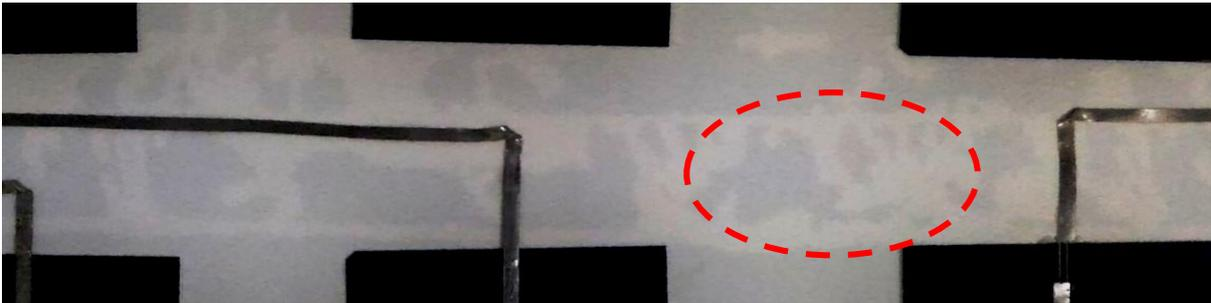
Fig 8.9: Section of the UV-pass sample showing the delamination (visible as white bubbles). The image has been taken under room light.
