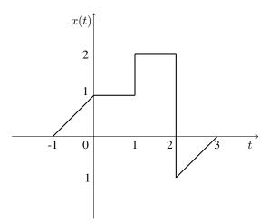
4. [†] Consider the signal y(t) = (1/5)x(-2t-3) shown below. Determine and carefully sketch the original signal x(t).
