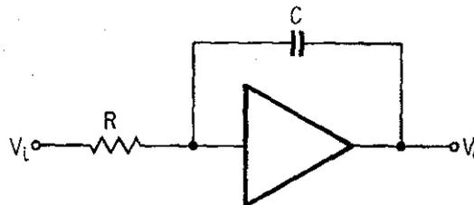
FIGURE 13.2.5. Inverting Integrator Circuit.
