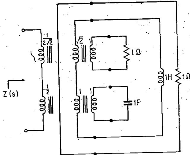
FIGURE 10.4.2. A Synthesis of  $Z(s)$  for Example 10.4.1.
