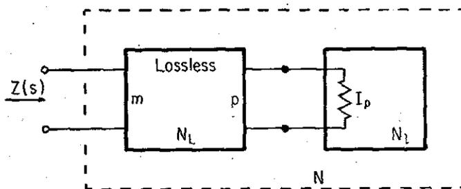
FIGURE 8.2.1. Resistance Extraction to Obtain a Lossless Coupling Network.
