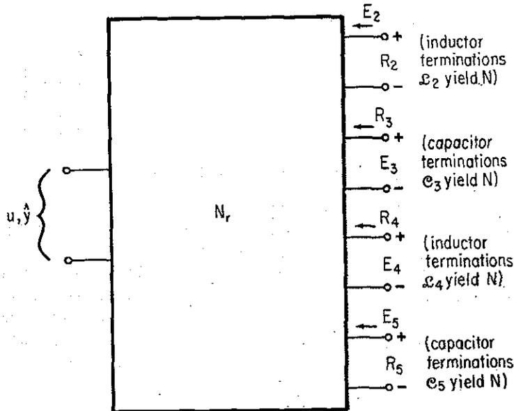
**FIGURE 4.4.4. Selection of Excitation Variables Prior to Generating State-Space Equations.**
