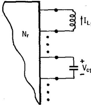
FIGURE 4.3.4. Definition of State Vector Components.
