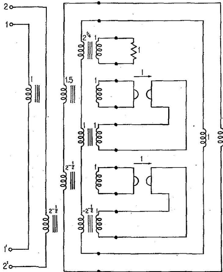
FIGURE 12.2.2. Synthesis of Transfer Function  $\frac{1}{2}(s^2 + \sqrt{2}s + 1)^{-1}$ .
