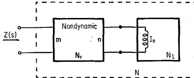
FIGURE 8.2.5. Inductor Extraction.
