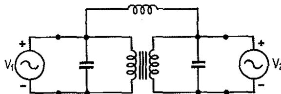
FIGURE 4.2-6. Network for Example 4.2.5. The Inputs  $V_1$  and  $V_2$  cannot be Chosen Independently.
