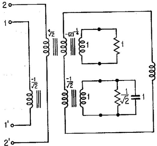
FIGURE 12.3.2. Reciprocal Synthesis of the Transfer Function  $\frac{1}{2}(s^2 + \sqrt{2}s + 1)^{-1}$ .
