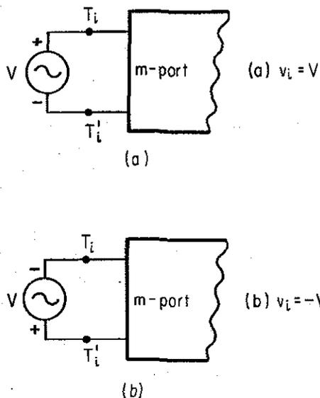
FIGURE 2.2.5. Connection of an Independent Voltage Source.
