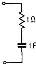
FIGURE 11.2.4. A Network Equivalent to that of Figure 11.2.2.
