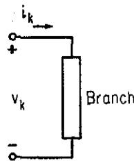
FIGURE 2.3.1. Reference Directions for Tellegen's Theorem.
