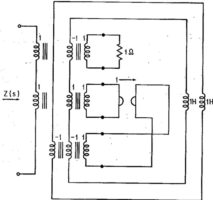
FIGURE 9.2.3. Complete Synthesis of  $Z(s)$  of Example 9.2.1.
