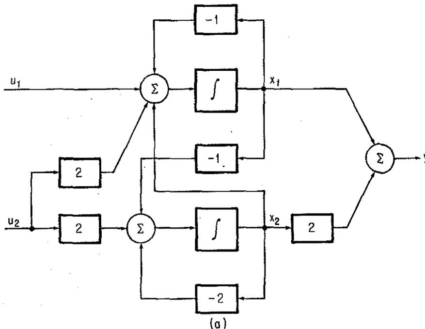
FIGURE 13.3.2. (a) Synthesis for Example 12.3.1, Showing Integrators, Gain Blocks and Summers.
