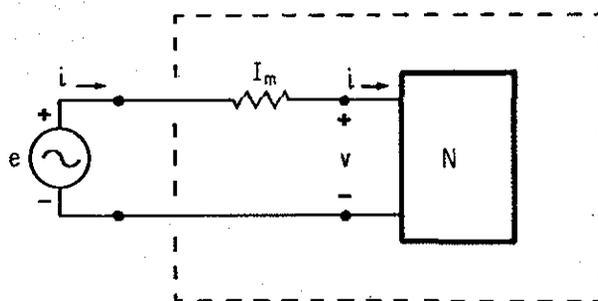
FIGURE 2.4.1. The Augmented  $m$ -Port Network.
