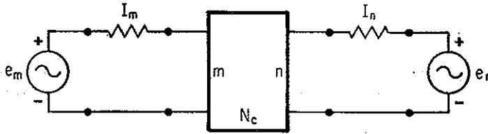
FIGURE 2.5.9. Augmented Network for  $N_c$  of Figure 2.5.8.
