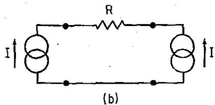
FIGURE 4.3.8. Network for Example 4.3.3.  $I$  and  $I_1$  cannot be taken as Independent Excitations.
