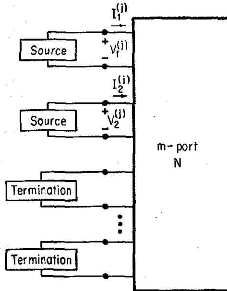
FIGURE 2.8.1. Arrangement to Illustrate Reciprocity;  $j = 1, 2$  Gives Two Operating Conditions for Network.
