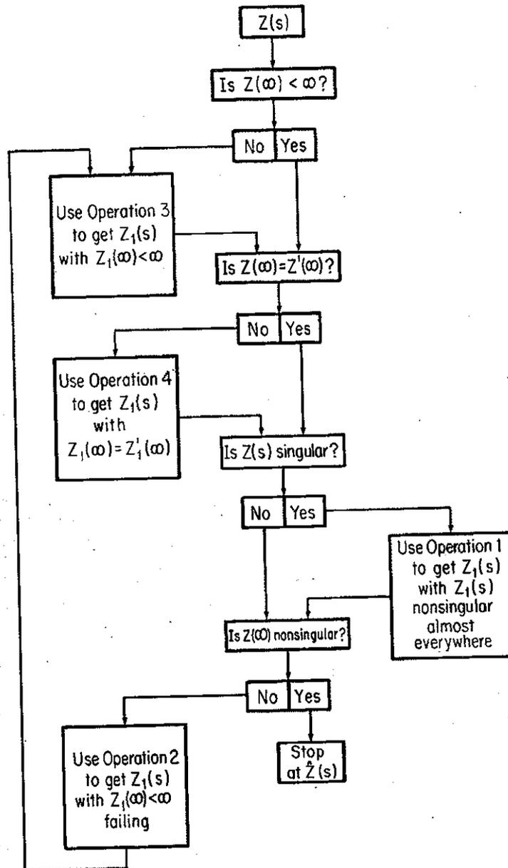
FIGURE 8.4.5. Flow Diagram Depicting Preliminary Lossless Extractions for Immittance Matrix Problem.
