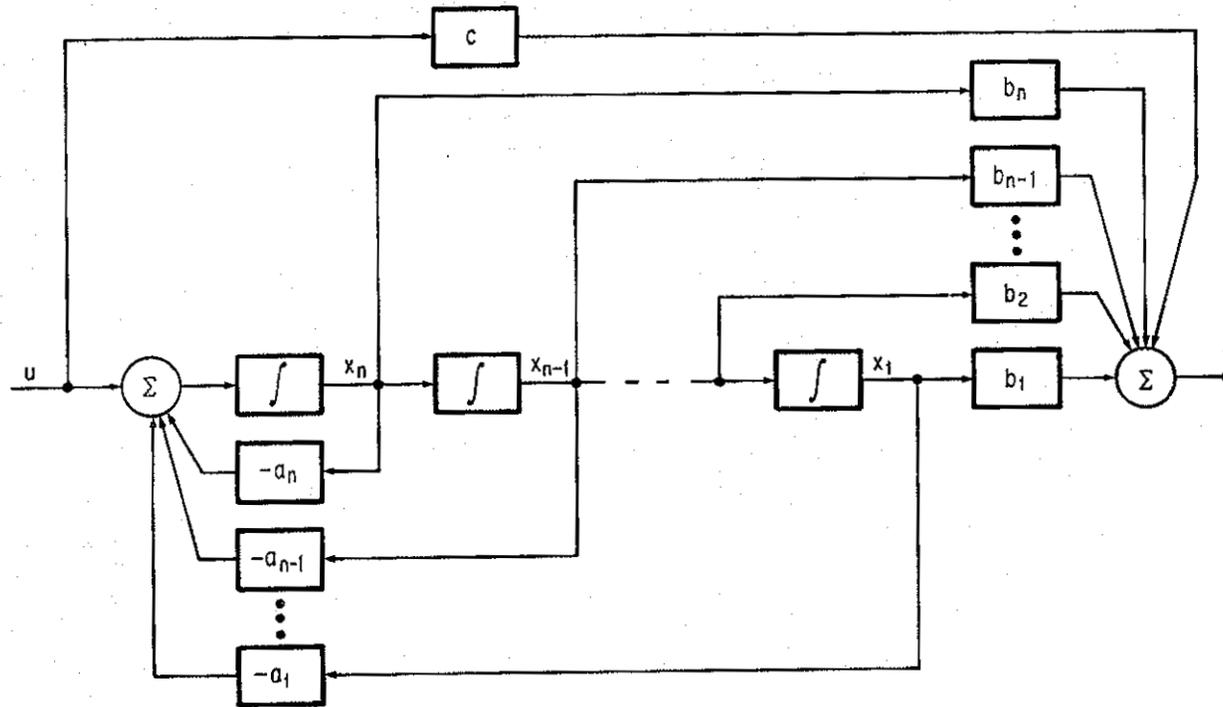
FIGURE 13.3.3. Block Diagram Representation of a State-Space Realization of a Scalar Transfer Function.
