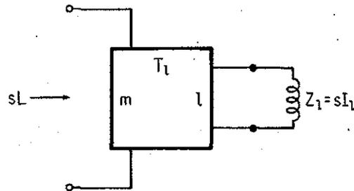
FIGURE 8.4.2. Synthesis of Impedance  $sL$ .
