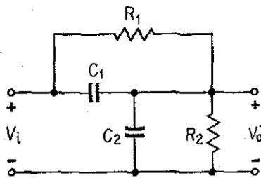
FIGURE 13.3.4. Realization of a First Order Transfer Function Using Passive Components Only.
