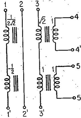
FIGURE 10.4.1. A Multiport Transformer Realizing  $T_e$  of Example 10.4.1.
