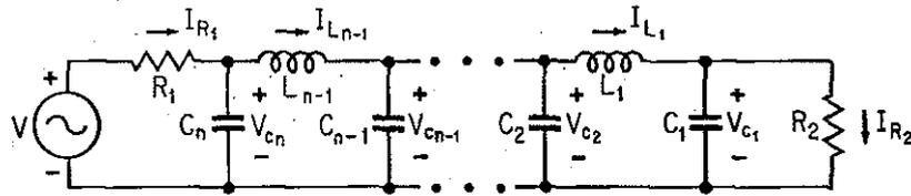
FIGURE 12.1.2. Ladder Network with State Equation (12.1.12).
