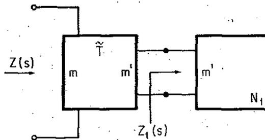
FIGURE 8.4.1. Conversion of a Singular  $Z(s)$  to a Nonsingular  $Z_1(s)$ .
