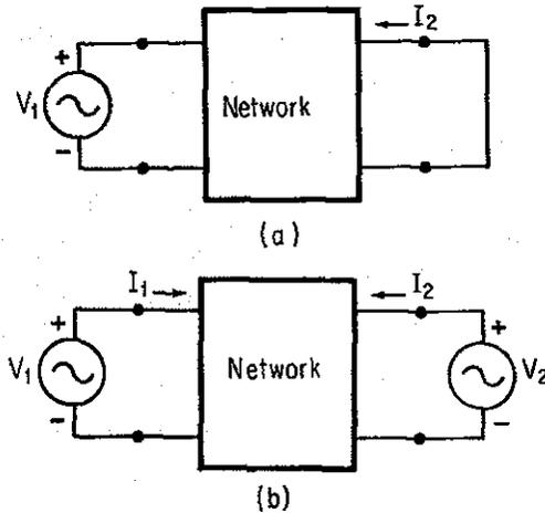
FIGURE 4.3.1. Introduction of Excitation at a Port where Response is Measured.
