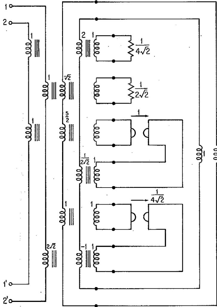
FIGURE 12.2.4. Synthesis of Transfer Function  $\frac{1}{2}(s^2 + \sqrt{2}s + 1)^{-1}$ .
