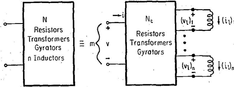
FIGURE 5.3.2. Redrawing of Network as Nondynamic Network Terminated in Inductors.
