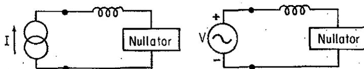
FIGURE 4.5.2. Circuits for which no State-Space Equations Exist
