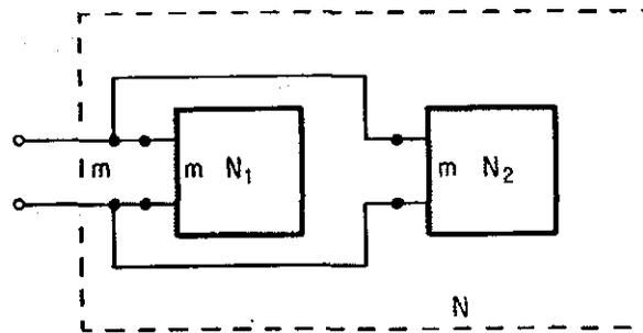
FIGURE 2.5.3. Parallel Connection.
