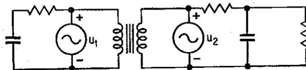
FIGURE 4.4.2. State-Space Equations Cannot Be Found with  $u_1$  and  $u_2$  as Excitations.
