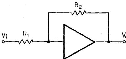
FIGURE 13.2.2. Single-Ended Operational Amplifier Generating Gain Element of Gain  $-(R_2/R_1)$ .
