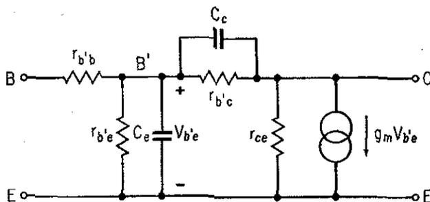
FIGURE 2.2.6. The Common Emitter Hybrid- $\pi$  Model of a Transistor.
