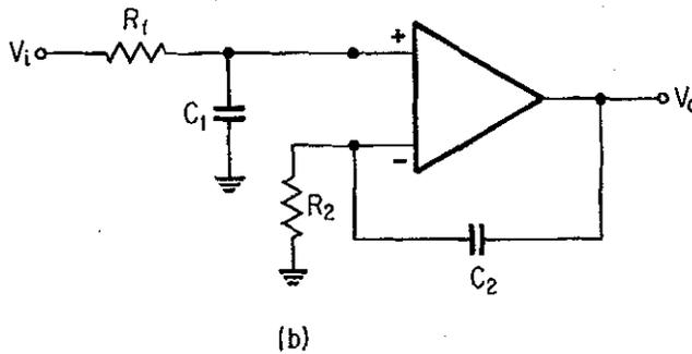
FIGURE 13.2.6. (a) Resistance Bridge Non-Inverting Integrator; (b) Balanced Time Constant Integrator.
