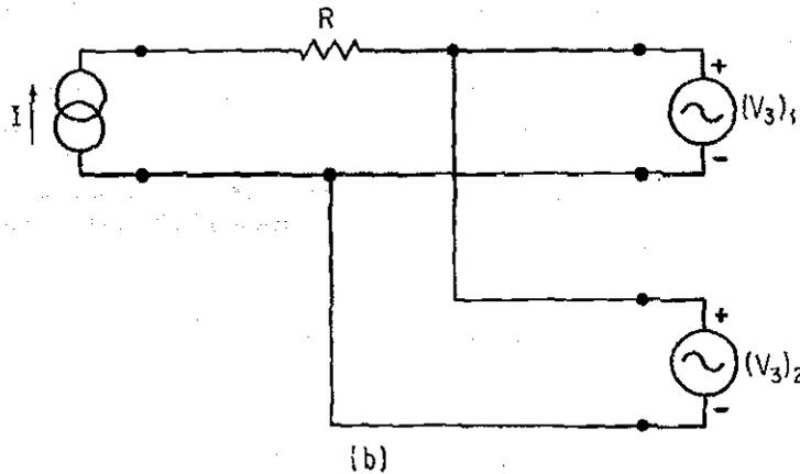
FIGURE 4.3.9. Network for Example 4.3.4.  $(V_3)_1$  and  $(V_3)_2$  are not independent.
