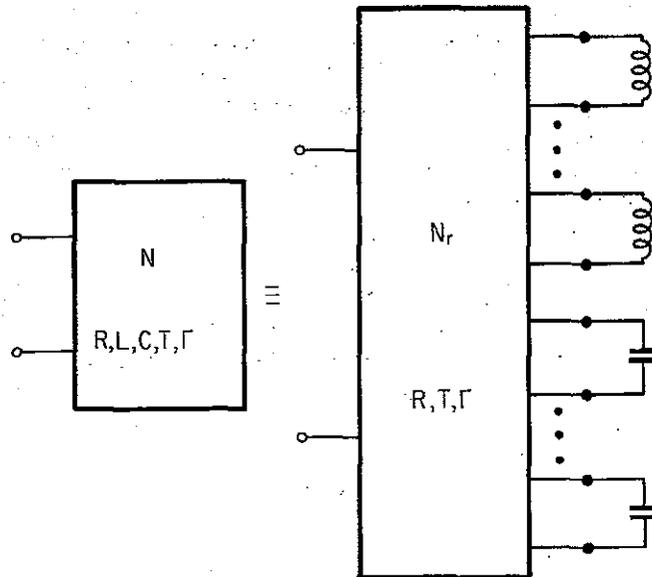
FIGURE 4.3.3. Illustration of Reactance Extraction.
