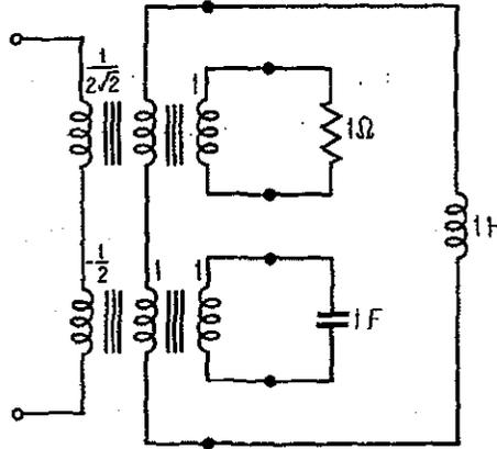
FIGURE 10.4.3. A Simplified Version of the Network of Fig. 10.4.2.
