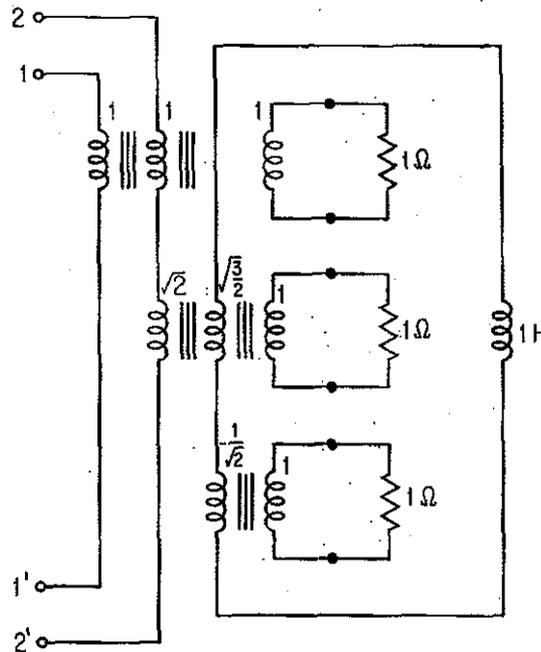
FIGURE 9.2.6. A Final Synthesis of  $Z(s)$  for Example 9.2.3.
