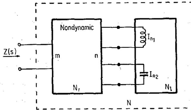
FIGURE 8.2.3. Reactance Extraction to Obtain a Nondynamic Coupling Network.
