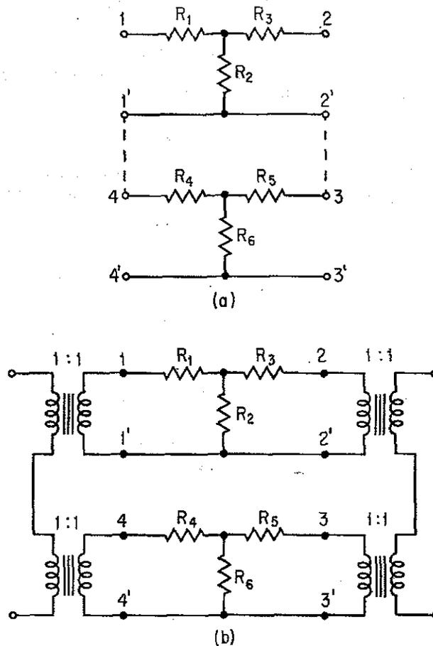
FIGURE 2.5.2. Series Connections Illustrating Nonadditivity and Additivity of Impedance Matrices.
