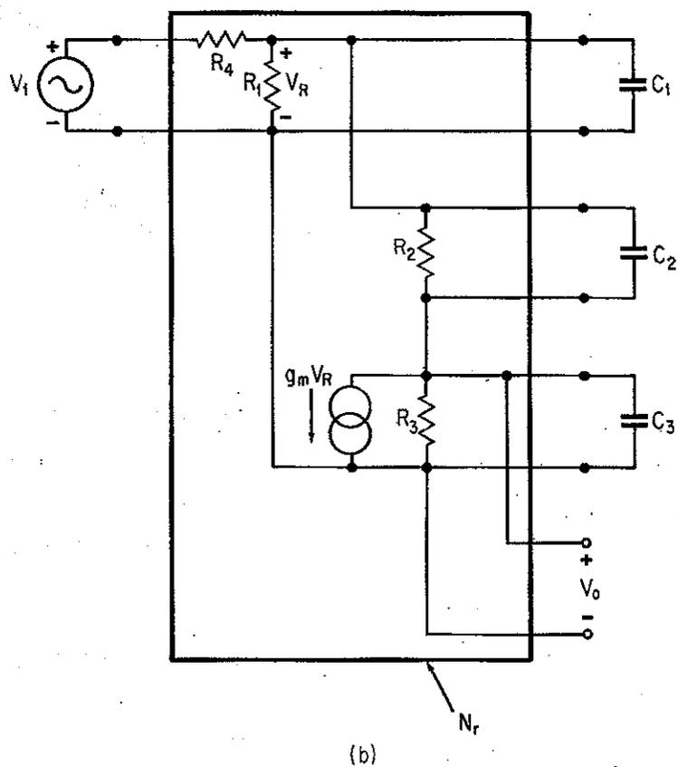
FIGURE 4.5.4. Network for Examples 4.5.2 and 4.5.3. The Network Models a Transistor.
