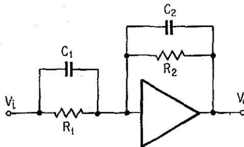
FIGURE 13.3.5. Realization of a First Order Transfer Function, Using Resistors, Capacitors and an Operational Amplifier.
