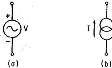
FIGURE 2.2.4. Independent Voltage and Current Sources.
