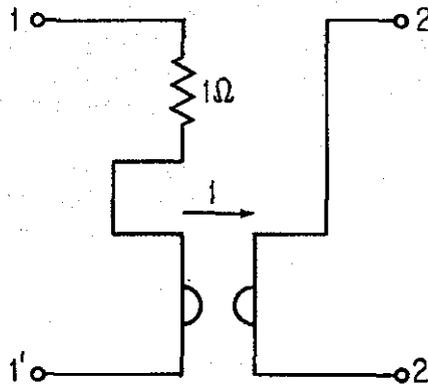
FIGURE 11.2.1. Synthesis of  $Z_a$  in Example 11.2.1.
