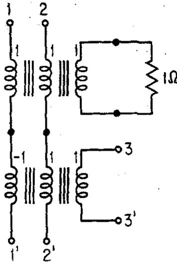
FIGURE 10.3.1. A Synthesis of the Hybrid Matrix  $M_1$ .
