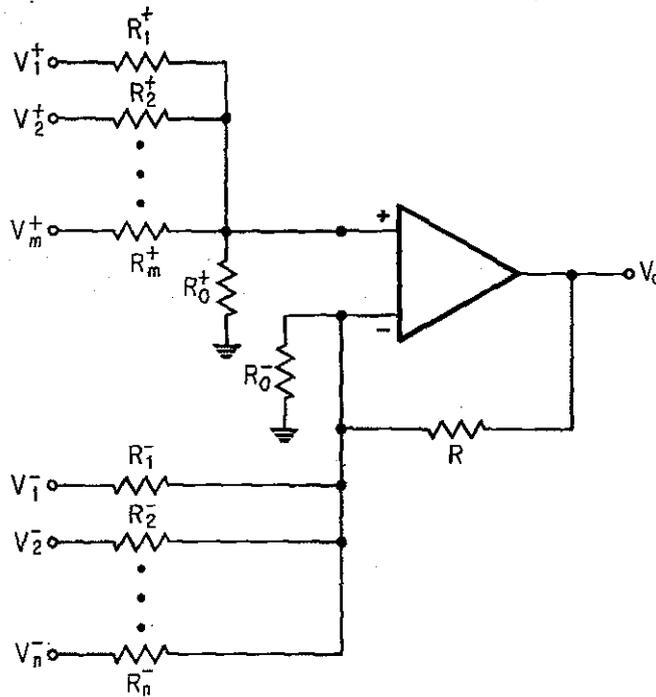
FIGURE 13.2.4. Differential-Input Operational Amplifier Generating a Summer.
