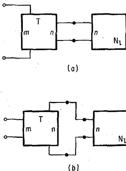
FIGURE 2.5.5. Cascade-Loaded Transformer Arrangements.
