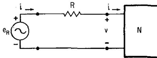
FIGURE 2.4.2. An  $m$ -port Network with Resistive Network Termination of Symmetric Impedance Matrix  $R$ .
