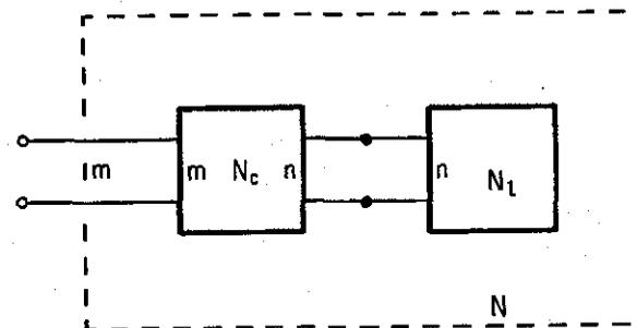
FIGURE 2.5.4. Cascade-Load Connection.
