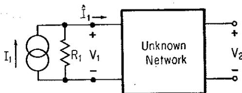
FIGURE 12.4.4. Arrangement for Input Loading Only.
