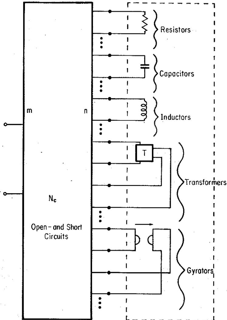
FIGURE 2.5.8. Cascade-Loading Representation for  $N_c$ .
