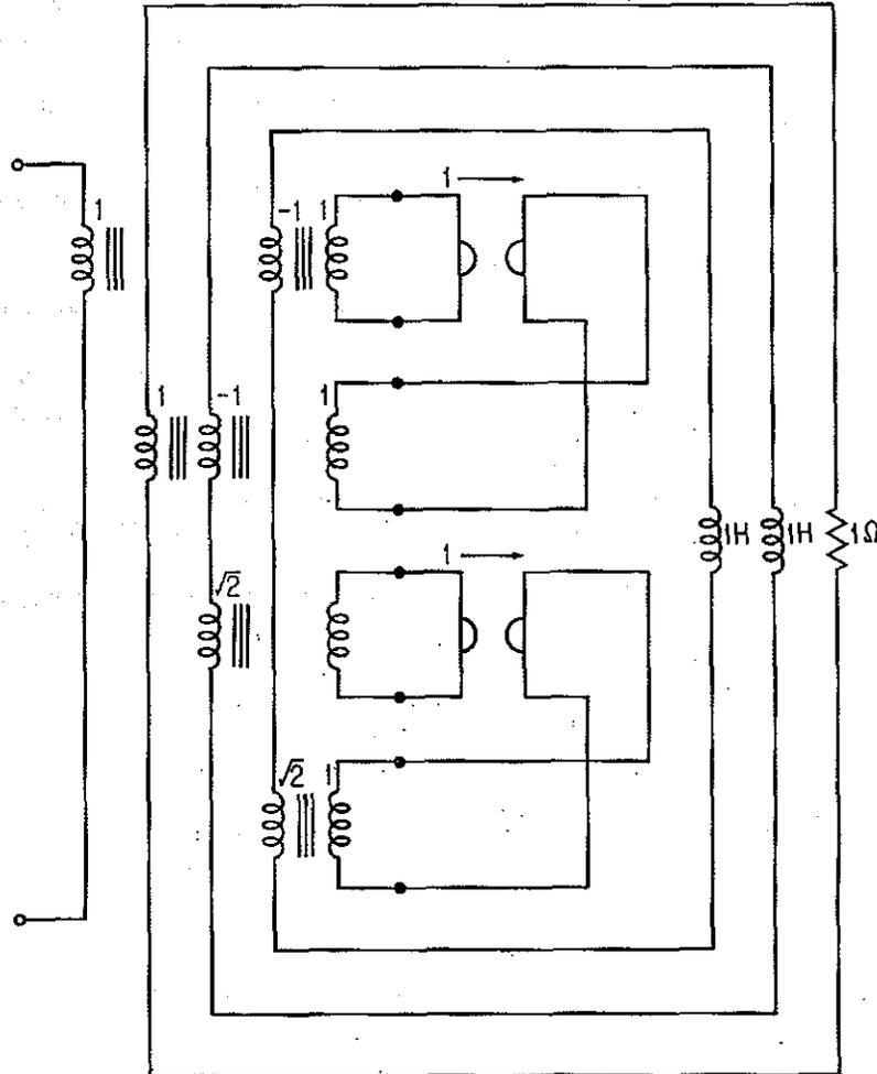
FIGURE 9.3.2. A Synthesis of  $Z(s)$  of Example 9.3.1.
