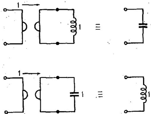
FIGURE 8.2.4. Element Replacements.
