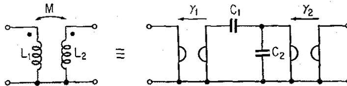
FIGURE 13.5.4. Replacement of Coupled Coils by Capacitors and Gyrators.
