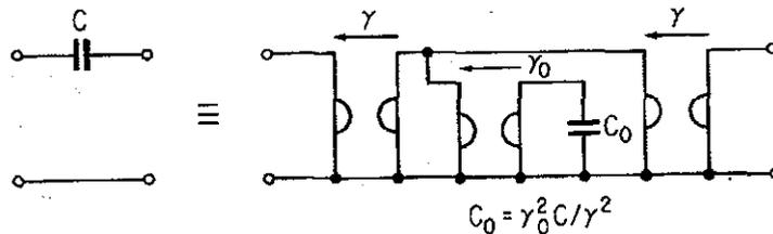
FIGURE 13.5.3. Replacement of Ungrounded Capacitor by Grounded Elements.
