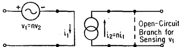
FIGURE 2.3.2. Redrawing of a Transformer.
