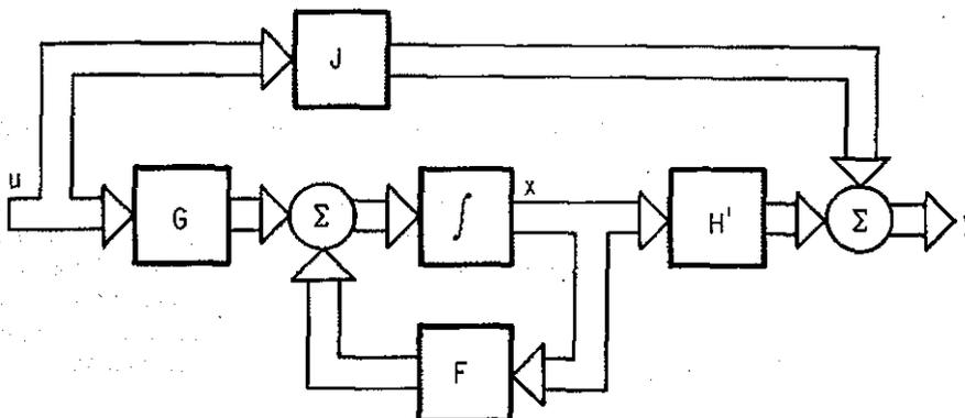
FIGURE 13.3.1. Block Diagram Representation of State-Space Equations.
