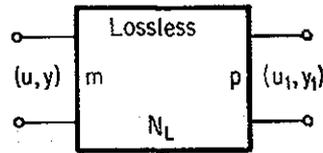
FIGURE 8.2.2. An  $(m + p)$ -port Lossless Network.
