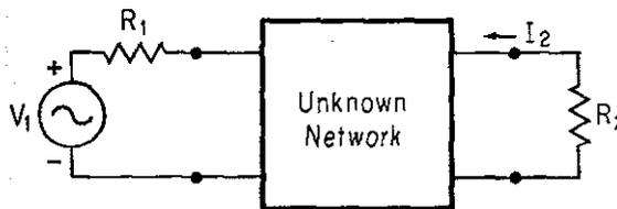
FIGURE 12.4.2. Synthesis Arrangement for Voltage-to-Current Transfer Function.
