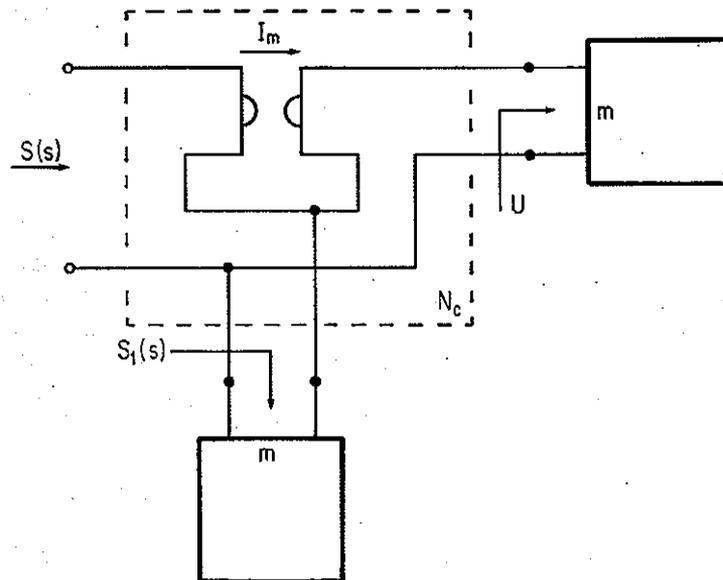
FIGURE 8.4.6. Connection for Scattering-Matrix Multiplication.
