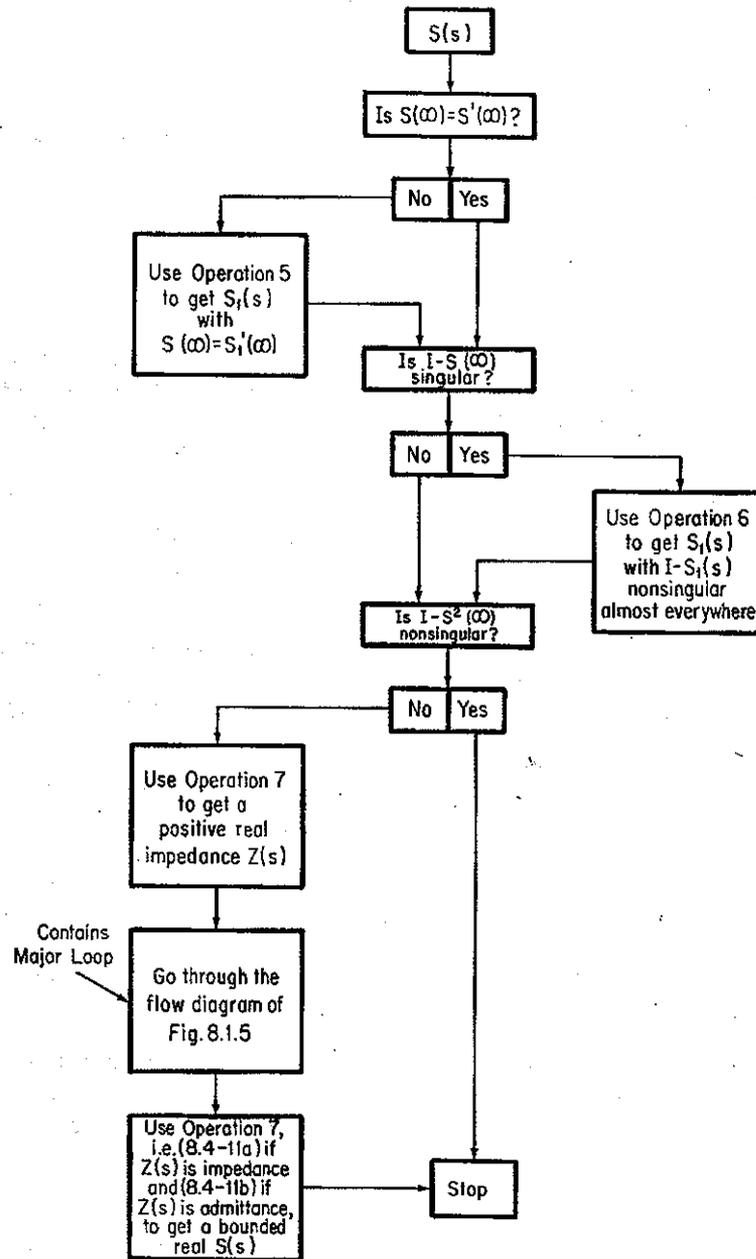
FIGURE 8.4.8. Flow Diagram Depicting Preliminary Lossless Extractions for Scattering Matrix Problem.
