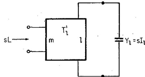
FIGURE 8.4.3. Synthesis of Admittance  $sL$ .
