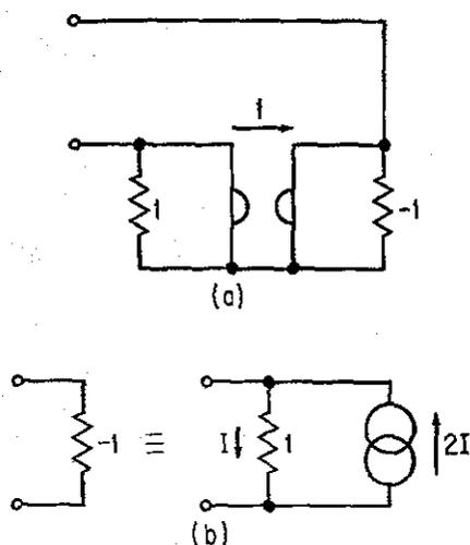
FIGURE 4.5.1. (a) The Nullator and (b) the Simulation of a Negative Resistor.
