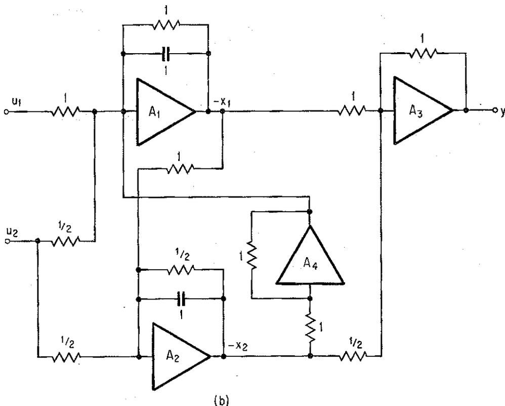
FIGURE 13.3.2. (b) Synthesis of Example 12.3.1, Showing Operational Amplifiers, Resistors and Capacitors.
