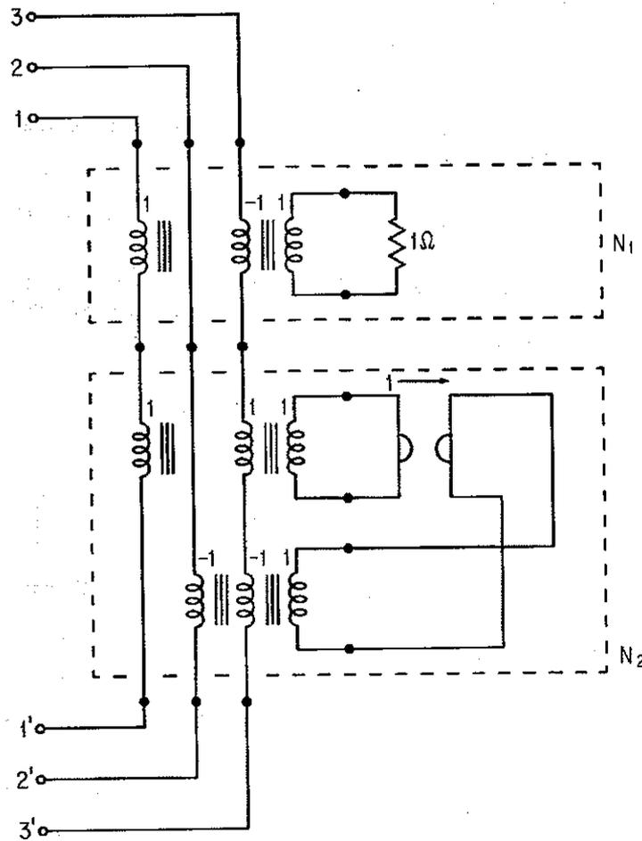
FIGURE 9.2.2. Synthesis of Nondynamic Coupling Network  $N_c$  for Example 9.2.1.
