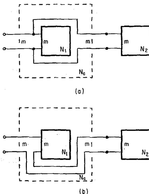
FIGURE 2.5.7. Cascade-Load Equivalents for: (a) Parallel; (b) Series Connection.
