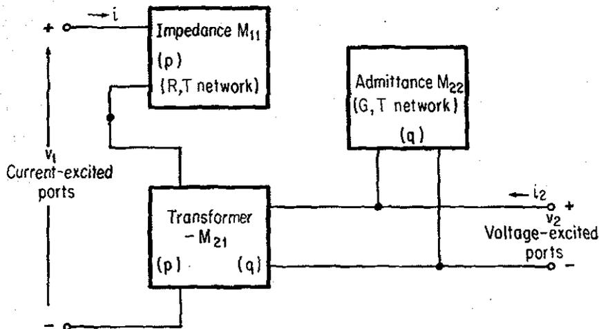
FIGURE 9.4.1. Synthesis of the Hybrid Matrix  $M$  of Equation (9.4.14).
