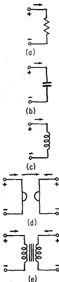
FIGURE 2.2.2. Representations and Definitions of Basic Circuit Elements.
