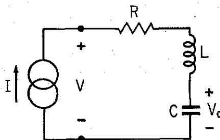
FIGURE 4.2.4. Second Network for Example 4.2.3.
