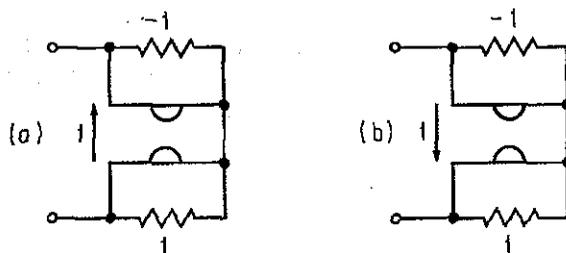
FIGURE 2.2.8. (a) The Nullator; and (b) the Norator.
