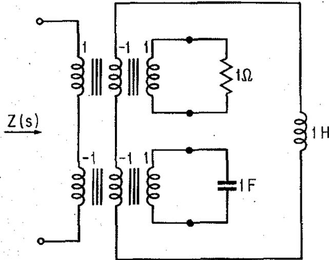
FIGURE 9.4.3. A Simplified Circuit Arrangement for Fig. 9.4.2.
