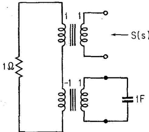
FIGURE 11.2.6. Synthesis of  $S(s)$  in Example 11.2.2.
