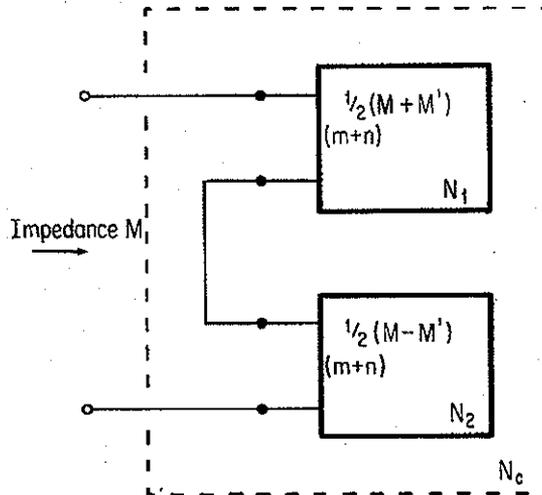
FIGURE 9.2.1. Series Connection of Impedances  $\frac{1}{2}(M + M')$  and  $\frac{1}{2}(M - M')$ .
