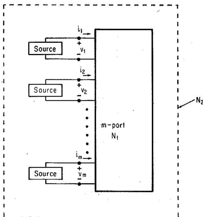
FIGURE 2.3.4. Passivity of  $N_1$  is Related to Passivity of Elements of  $N_1$ .
