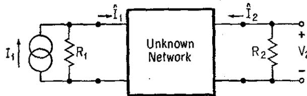
FIGURE 12.4.1. Synthesis Arrangement with  $R_1$  and  $R_2$  Known.
