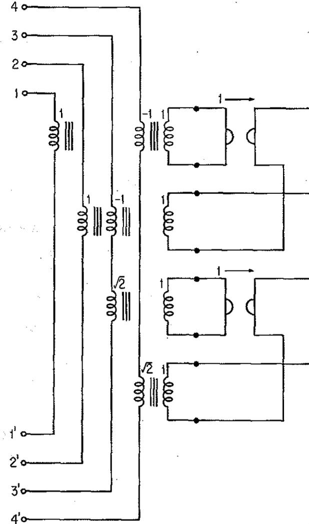
FIGURE 9.3.1. Synthesis of  $M$  in Example 9.3.1.
