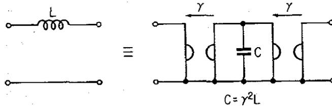
FIGURE 13.5.2. Inductor Equivalence Involving Grounded Capacitor and Gyrators.
