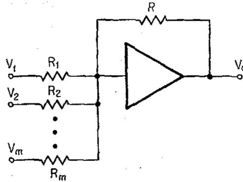
FIGURE 13.2.3. Single-Ended Operational Amplifier Generating a Summer.
