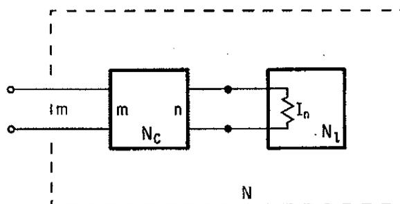
FIGURE 2.5.6. Special Cascade Load Connection.
