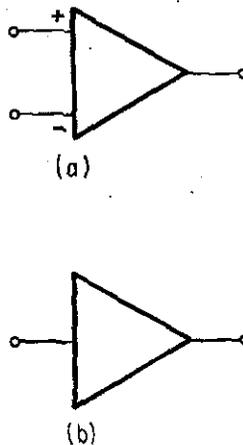
FIGURE 13.2.1. (a) Differential-Input Operational Amplifier; (b) Single-Ended Operational Amplifier.
