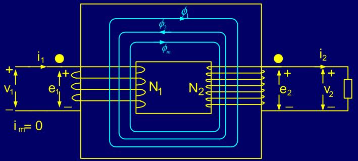
Steady state will reach when,  $\phi_1 = \phi_2$  Therefore at steady state  $\phi_1 = \frac{N_1 i_1}{\text{reluctance}}$   $\phi_2 = \frac{N_2 i_2}{\text{reluctance}}$   $N_1 i_1 = N_2 i_2$  $\frac{i_1 = N_2}{N_2}$
