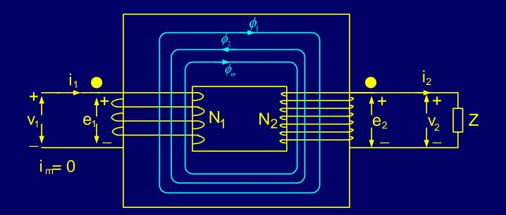
$\frac{v_1}{v_2} = \frac{e_1}{e_2} = \frac{V_1}{V_2} = \frac{N_1}{N_2}$  $\frac{i_1}{i_2} = \frac{N_2}{N_1} = \frac{e_2}{e_1} = \frac{v_2}{v_1}$
