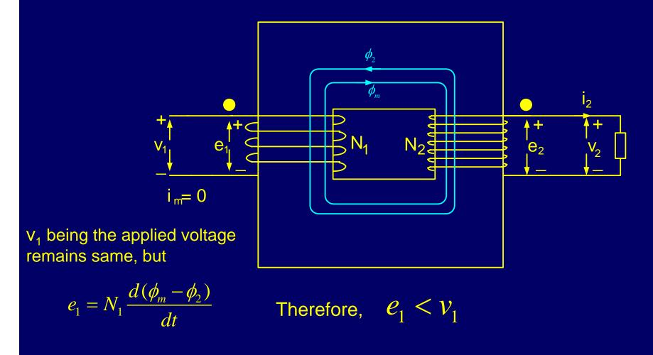
Hence a current  $i_1$  flows from v1 to "dot" terminal of winding 1. Flow of current  $i_1$  in N<sub>1</sub> sets a flux  $\phi_1$  in the core
