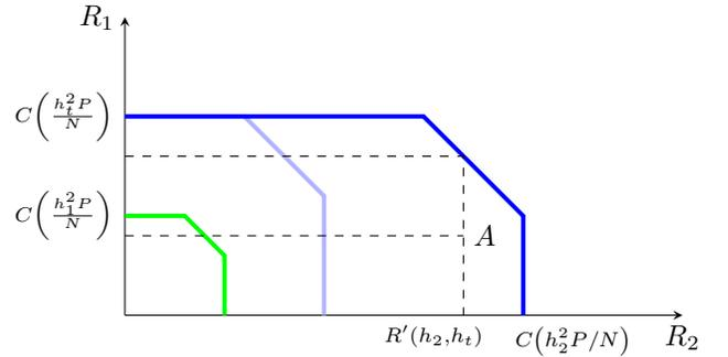
Fig. 3. Here,  $C(x) \triangleq \frac{1}{2} \log(1 + x)$ . User 2, who is beyond the threshold, constructs the outer two pentagons assuming 1 to be at most as good as the intermediate region. User 1, who is within threshold constructs the innermost region, choosing its midpoint rate.  $A$  denotes the final operating point.
