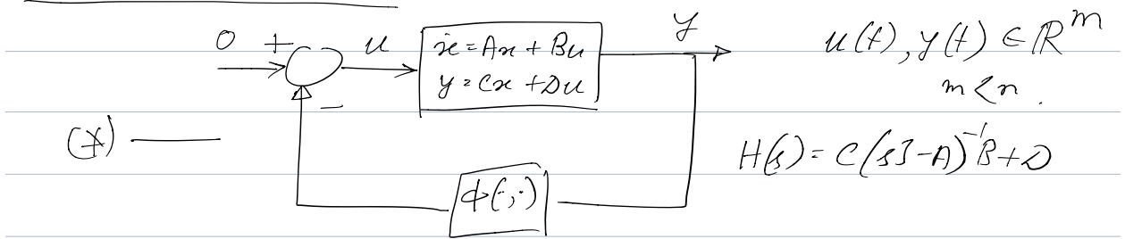
$$\Rightarrow u(t) = -\phi(t, y(t)) \quad \{ \dot{x} = Ax + Bu, y = Cx + Du \} \quad (1)$$
