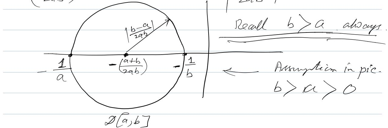
Thm (Circle Criterion): Consider the Luré system with  $m = 1$ . Let (i)  $(A, b, c, d)$  be minimal realization of  $h(s)$ , (ii)  $\phi$  belong to set  $[a, b]$ . Then the feedback system is globally exponentially stable if one of the following conditions, as appropriate holds:
