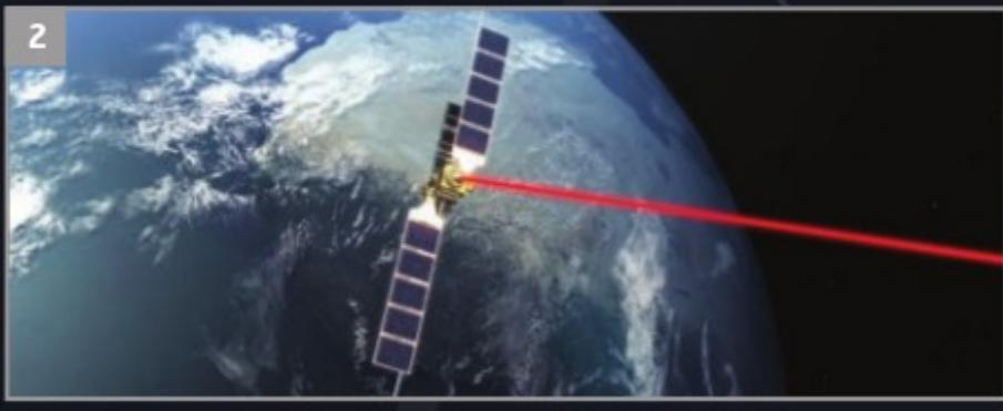
An EDRS laser terminal locates the lower orbiting satellite
