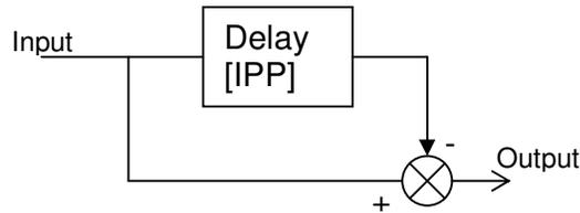
A two-pulse cancellor is used if the clutter component [assuming DC only] remains constant in a given range bin and can be eliminated by subtracting the output from two successive pulses. The transfer function of two-pulse cancellor is equal to  $1 - z^{-1}$ . And is equivalent to FIR digital filter with magnitude response  $\sin(\omega/2)$ .
