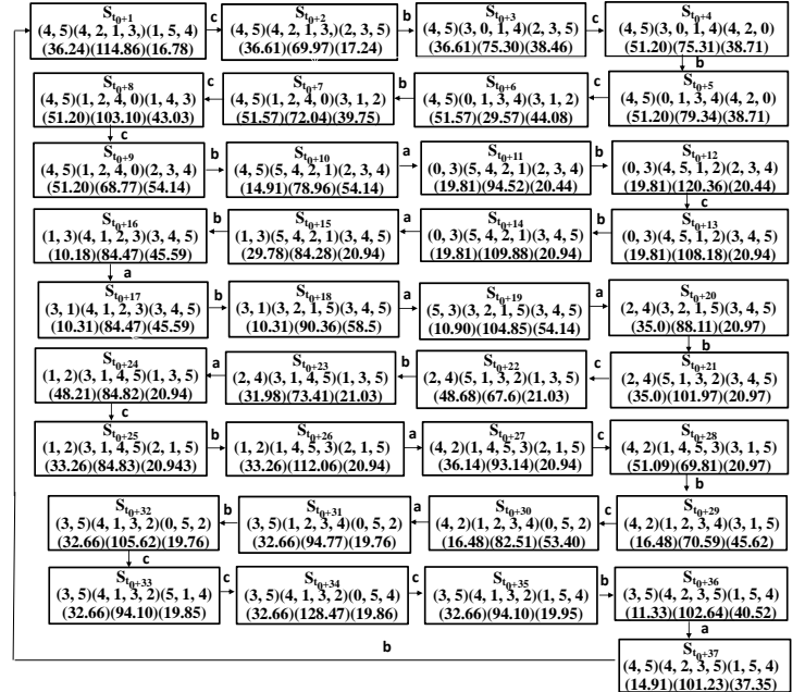
Fig. 2: The figure shows the existence of a cycle formed by the strategy profiles \mathbf{S}_{t_0+1}, \dots, \mathbf{S}_{t_0+37} . Each box represents the strategy profile along with the subchannels allocated to MSs in the second row and corresponding utilities of the BSs in the third row. In each strategy profile update, the BS indicated on the arrow changes its allocation such that its utility increases.
