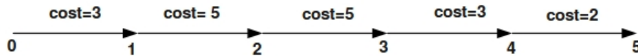
Figure 6.3: A subgraph G_{sub} , which includes only the critical path, with calculated cost on the edges
