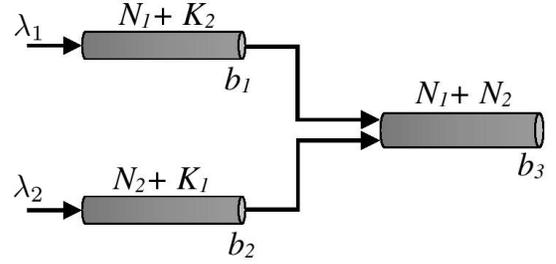
Fig. 4. A circuit multiplexed network whose analysis is the same as the analysis of the deterministic sharing scheme.
