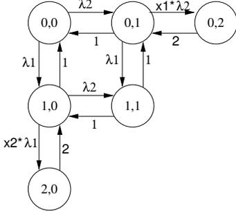
Fig. 1. Markov chain representation of the probabilistic sharing model with each service provider having one channel
