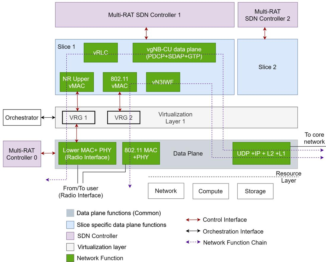
Figure 5.3: Example of virtualization of the proposed architecture for 5G NR and WLAN
