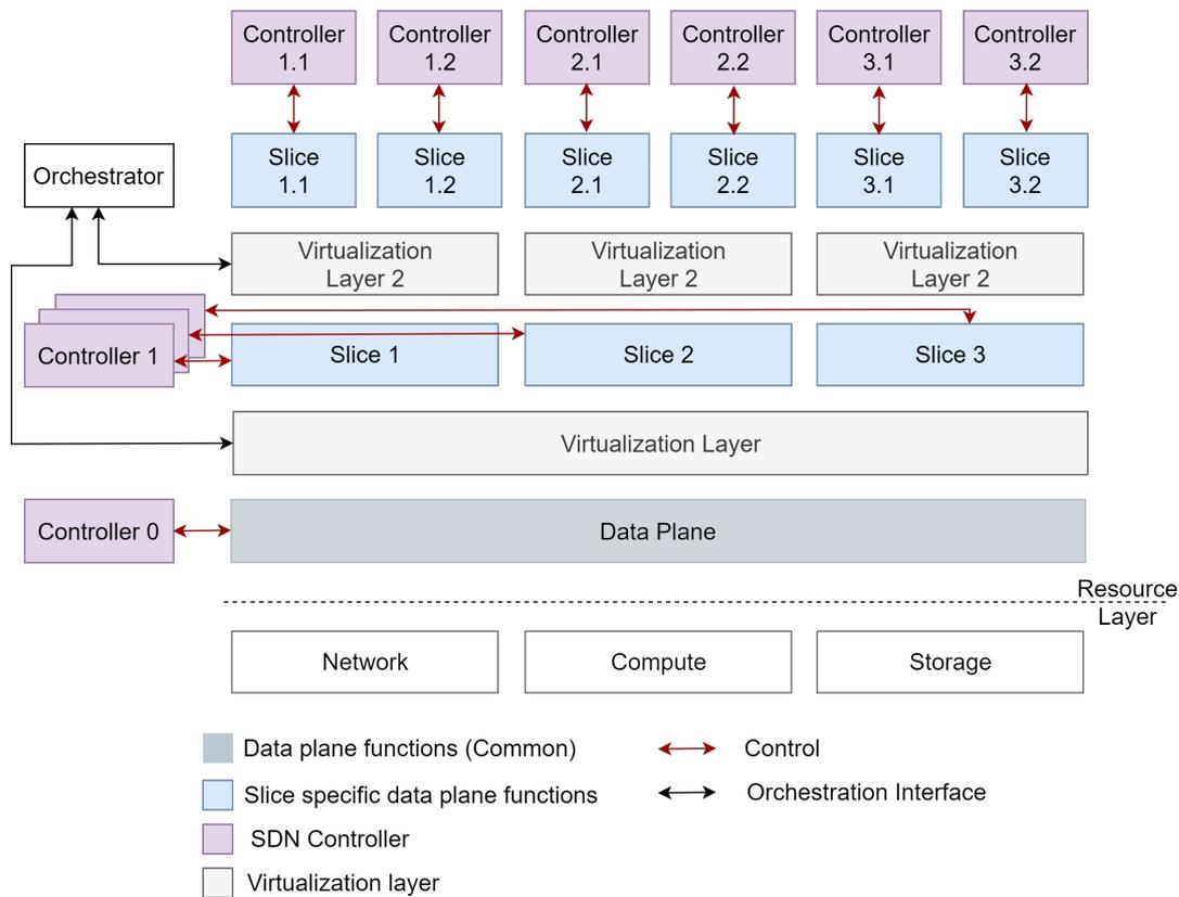
Figure 5.1: Proposed recursive architecture for slicing
