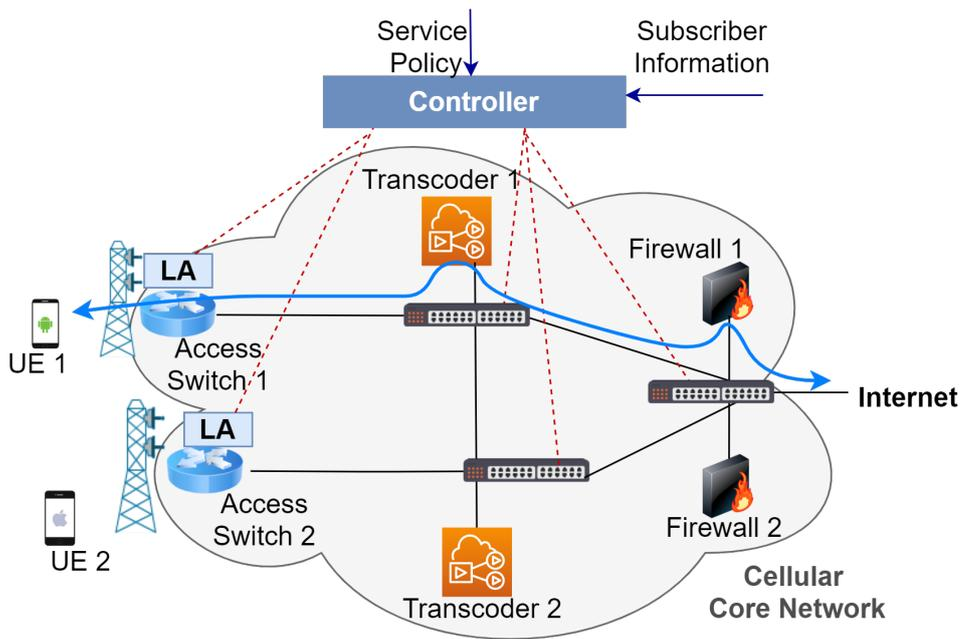
Figure 2.2: SoftCell architecture (courtesy [32])
