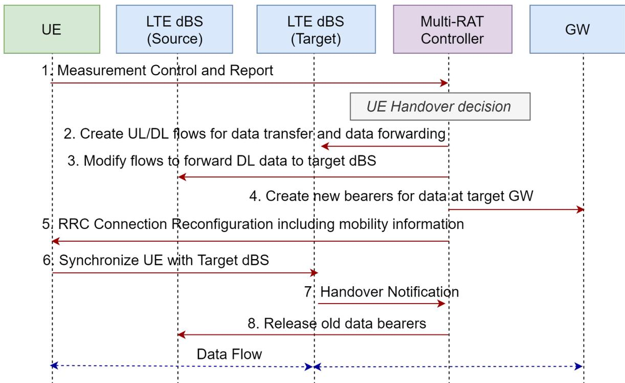
Figure 4.5: Call flow for UE handover within LTE RAT in the proposed architecture
