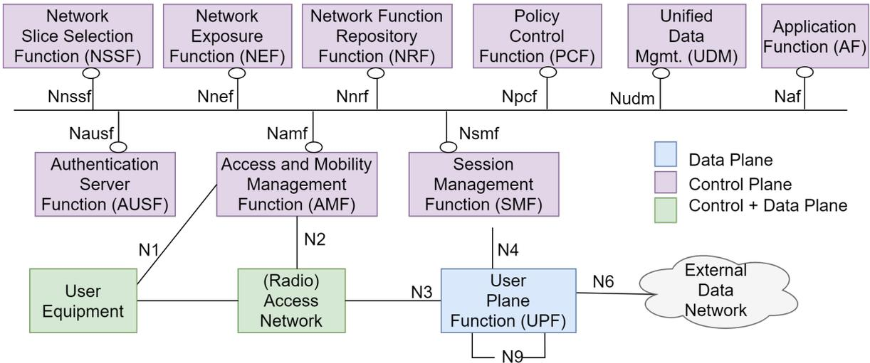
Figure 3.1: 3GPP 5G network architecture (courtesy [21])
