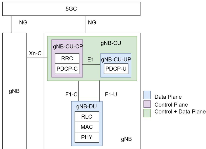
Figure 3.2: 3GPP 5G NR dis-aggregated architecture (courtesy [21])
