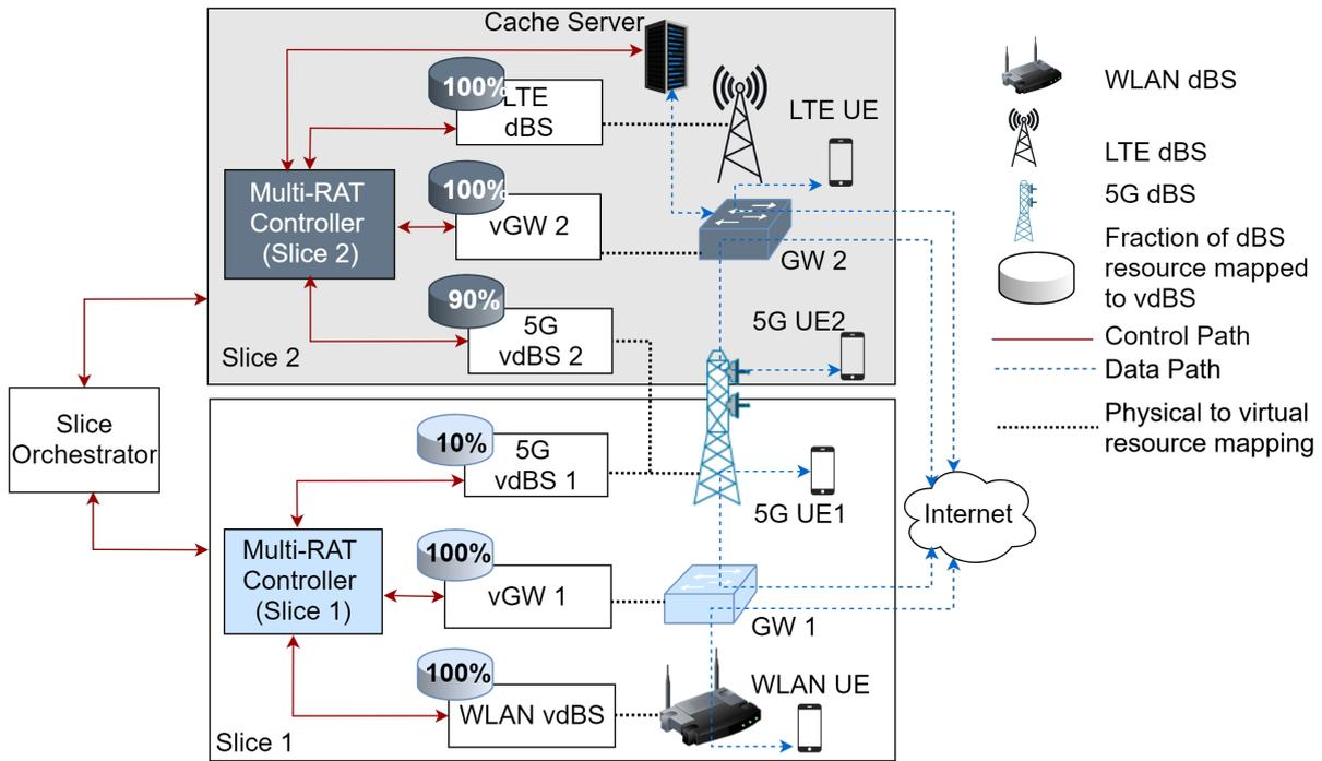
Figure 4.3: An example deployment within the proposed architecture
