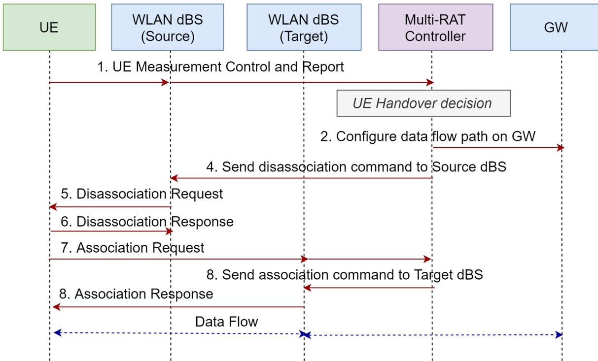
Figure 4.6: Call flow for UE handover within WLAN RAT in the proposed architecture
