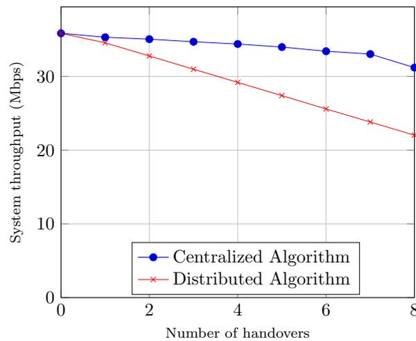
Figure 3.11: System throughput comparison for load balancing in centralized SDN versus traditional distributed LTE architectures
