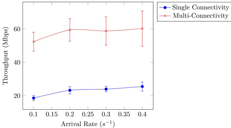
Figure 6.8: Median system throughput v/s user arrival rates for different connectivity types.
