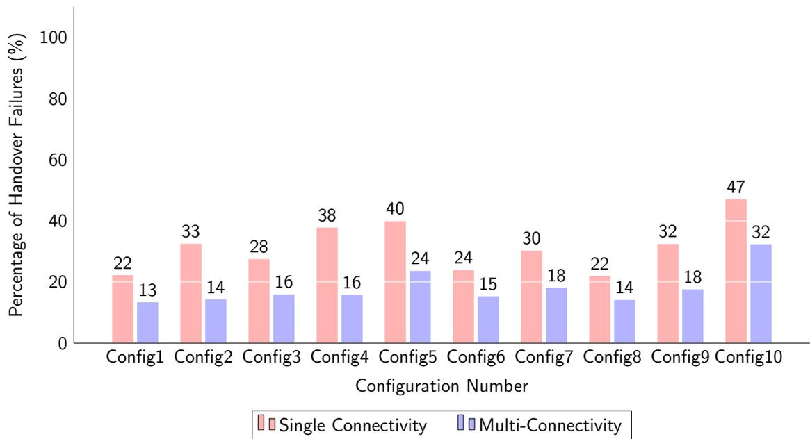
Figure 6.9: Percentage of handover failures for various slice configurations in LTE
