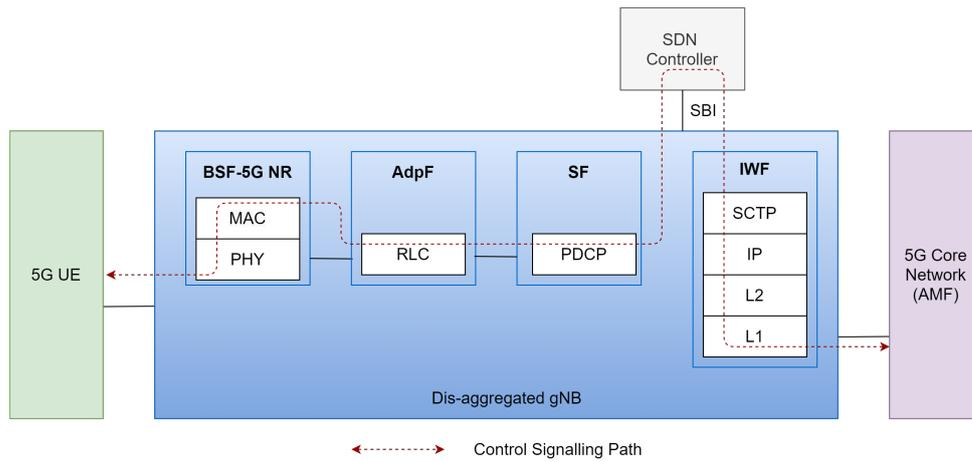
Figure 7.3: RAN dis-aggregation of the gNB control plane protocol stack
