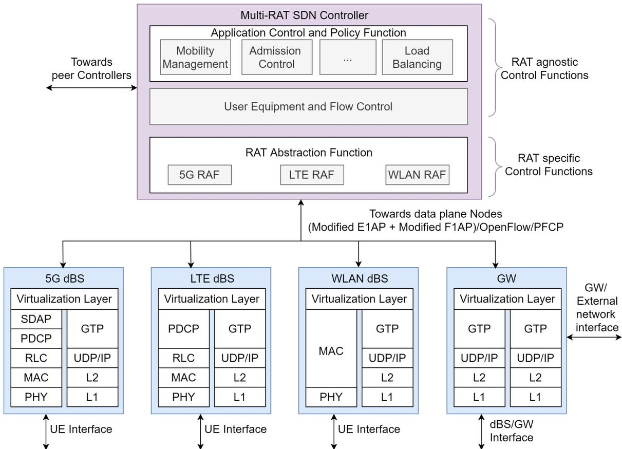
Figure 4.2: Proposed multi-RAT controller architecture and interfaces
