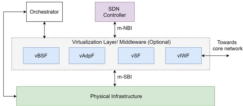
Figure 7.4: Architecture for dis-aggregating RAN nodes in existing networks
