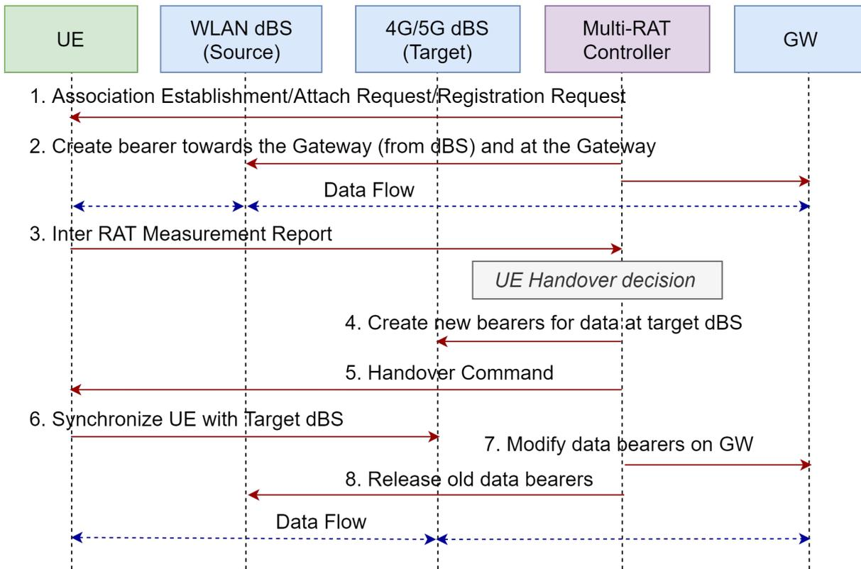
Figure 4.4: UE handover (WLAN to 3GPP 4G/5G) call flow within the proposed architecture
