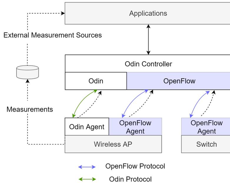
Figure 2.1: System architecture of Odin (courtesy [29])
