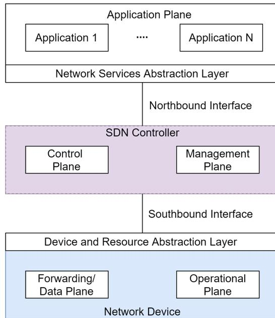
Figure 1.4: SDN architecture (adapted from [14])
