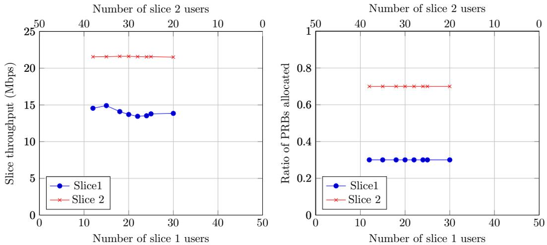
(a) Throughput for slices when slicing is performed at PDCP and MAC layers
