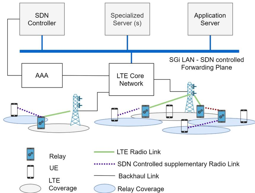
Figure 7.1: Proposed SDN based overlay network architecture
