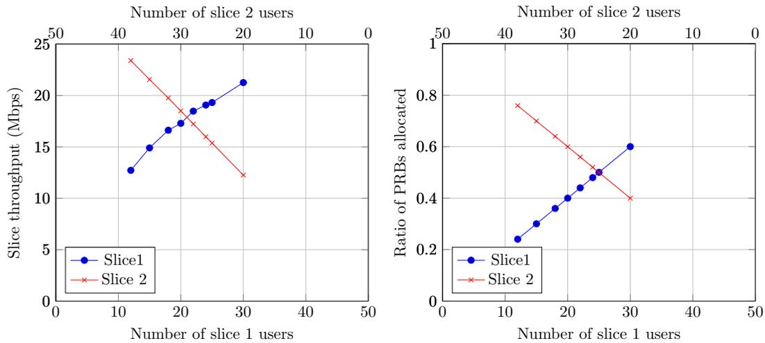
(a) Throughput for slices when slicing is performed at PDCP layer (b) Ratios of PRBs allocated when slicing is performed at PDCP layer
