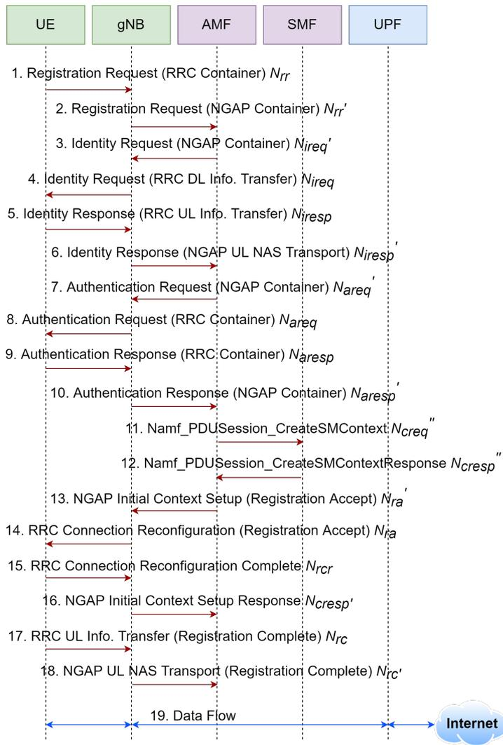
Figure 3.6: Registration procedure for the 3GPP defined 5G architecture (courtesy [21])
