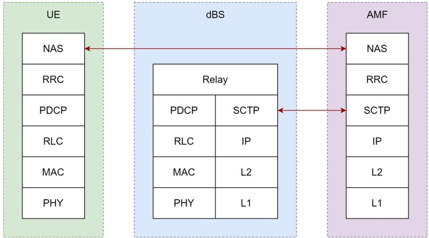
Figure 3.5: Control plane stack for the proposed architecture
