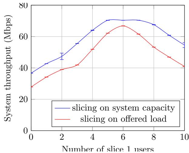
Figure 5.6: Comparison of system throughput for resource division based on system capacity and offered load
