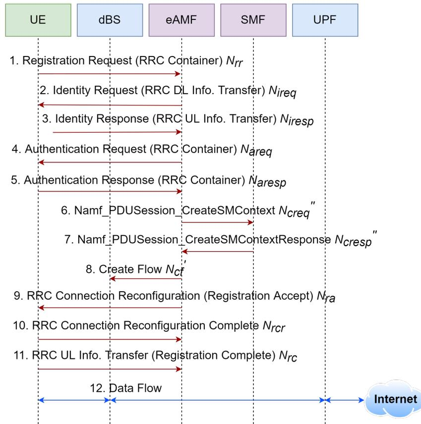
Figure 3.7: Registration procedure for the proposed architecture
