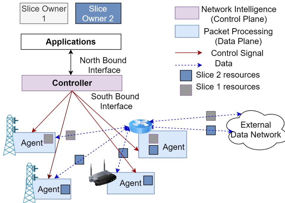
Figure 1.6: Illustration of SDN and network slicing in a wireless network
