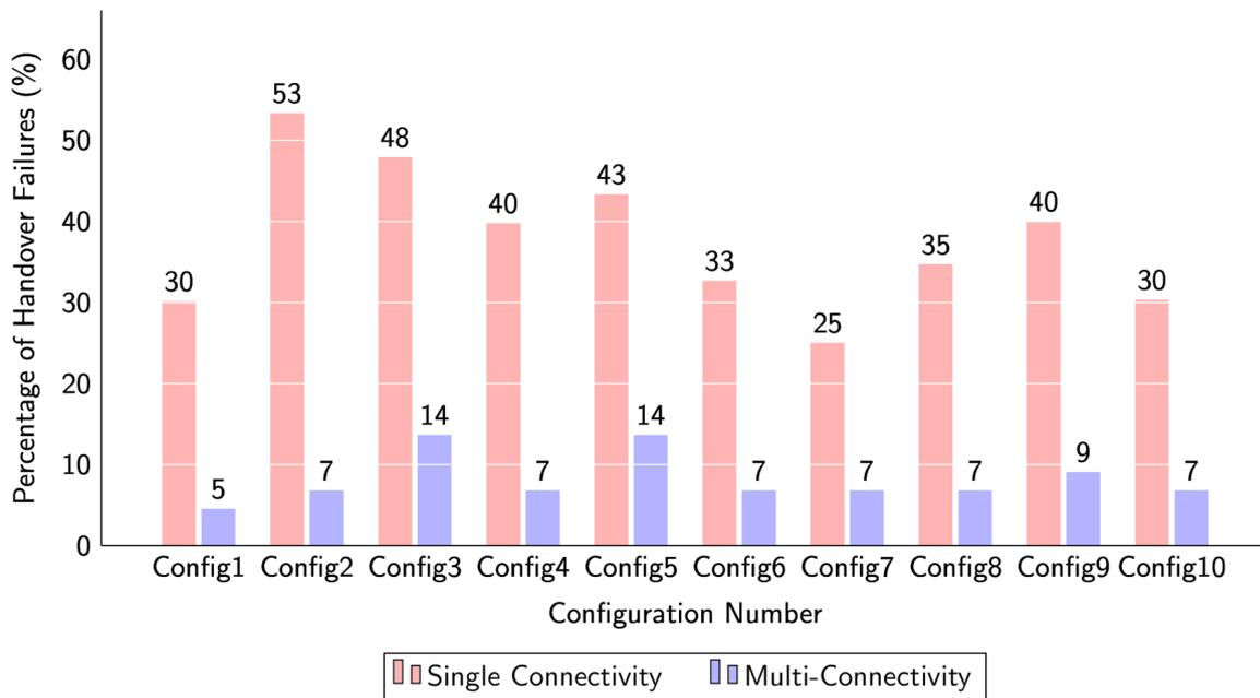
Figure 6.10: Percentage of handover failures for various slice configurations for multi-RAT network
