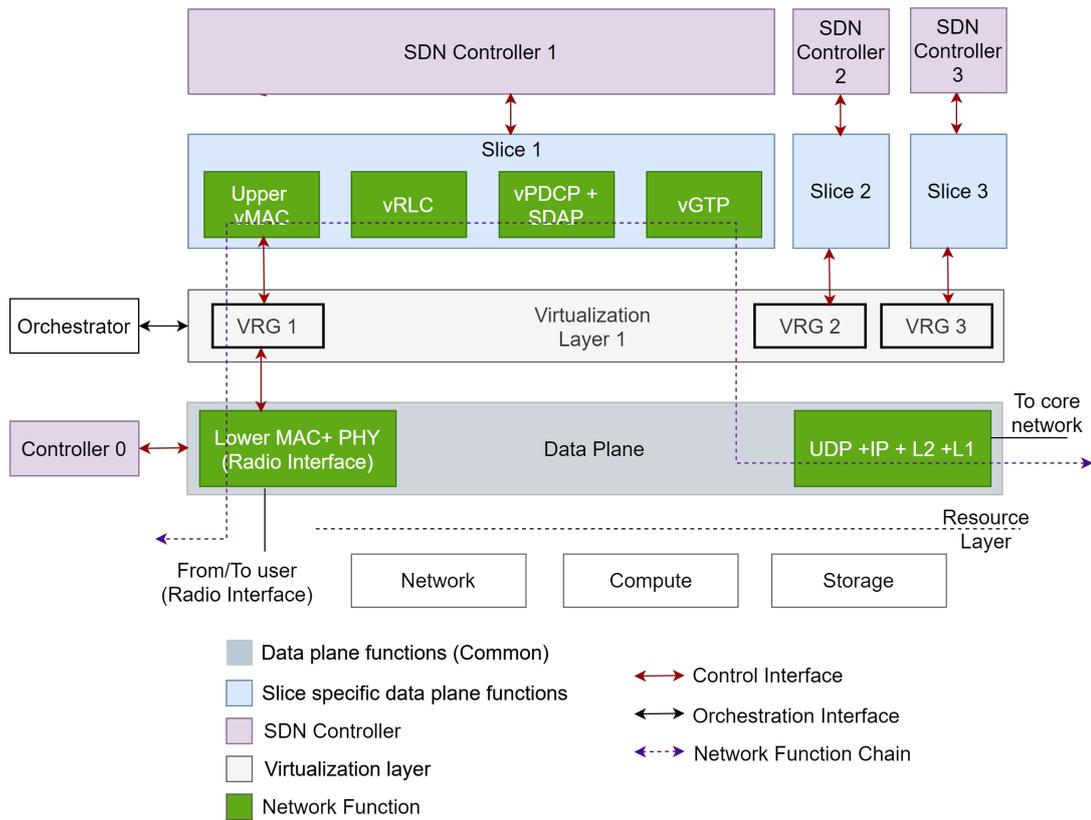
Figure 5.2: Data Path illustration for 5G NR in the proposed recursive architecture
