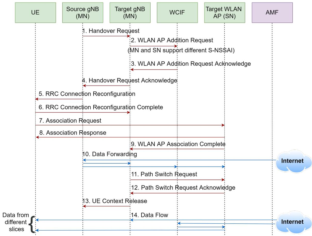
Figure 6.4: Proposed slice handover to both 5G NR and WLAN using multi-connectivity
