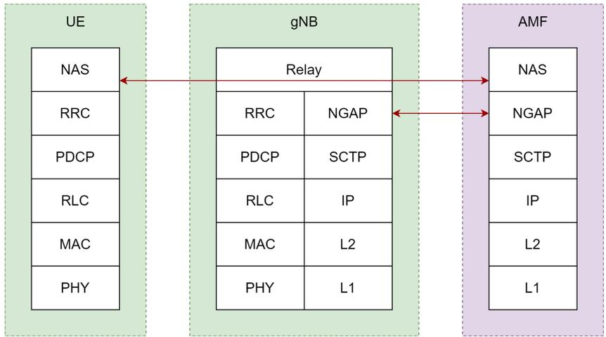
Figure 3.4: 3GPP defined 5G control plane stack (courtesy [21])
