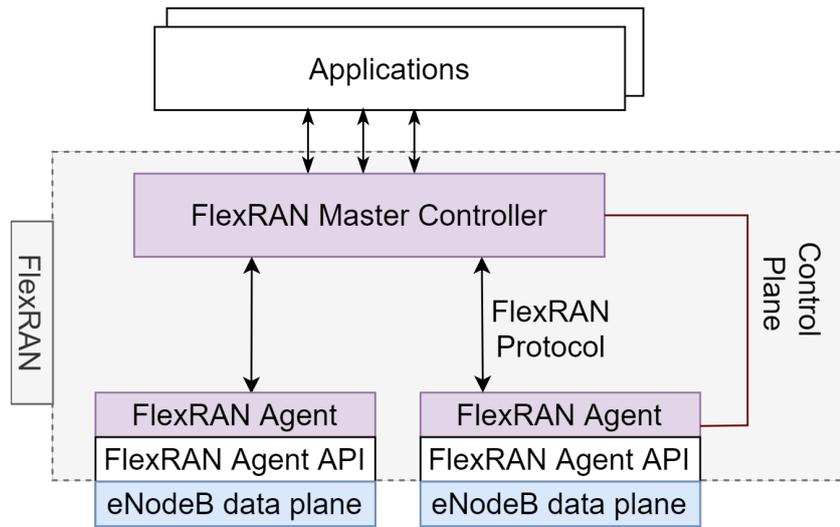
Figure 2.3: System architecture for FlexRAN (courtesy [37])
