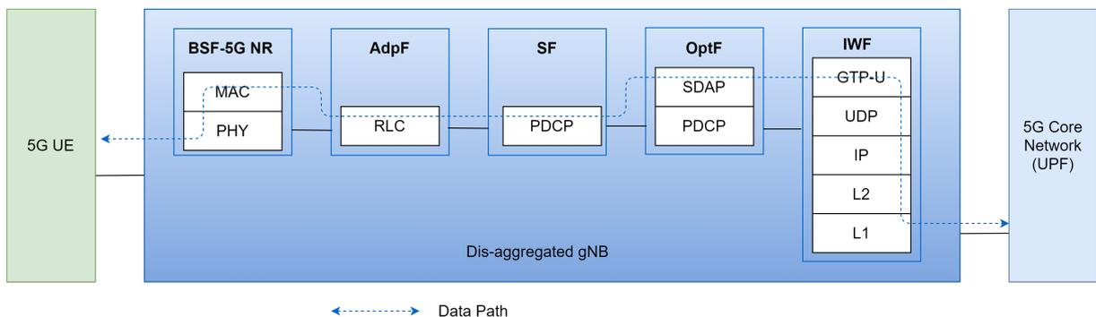
Figure 7.2: RAN dis-aggregation of the gNB user plane protocol stack
