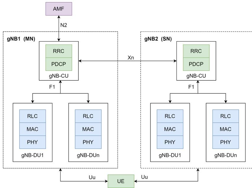
Figure 6.1: Block diagram of 3GPP NR multi-connectivity architecture
