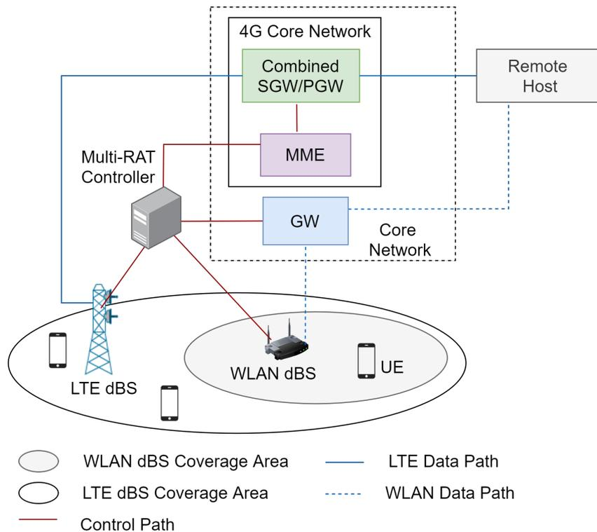
Figure 4.7: SDN based multi-RAT controller simulation setup
