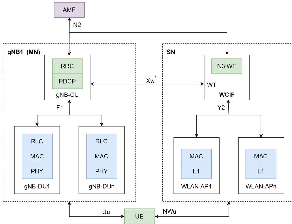
Figure 6.2: Block diagram of proposed NR-WLAN multi-connectivity architecture
