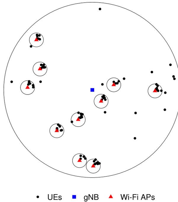
Figure 4.3: A single cell simulation scenario with 1000 m cell radius and multiple Wi-Fi basic service areas
