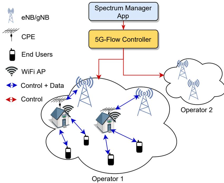
Figure 6.1: Overview of a multi-operator middle mile network
