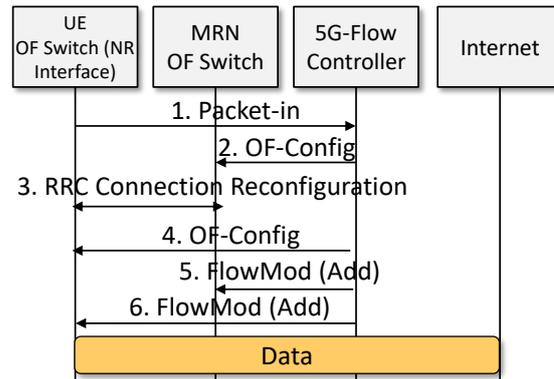
Figure 3.8: Call Flow to illustrate the communication of UE with the Internet
