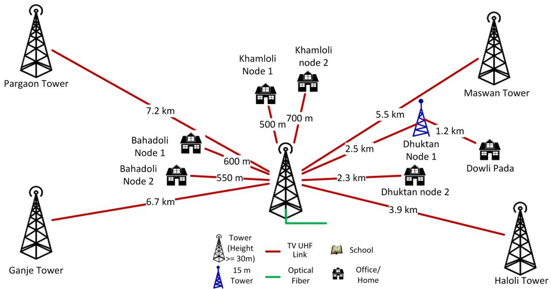
(a) Network topology of Palghar testbed
