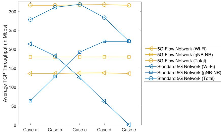
Figure 4.5: Load balancing across RATs
