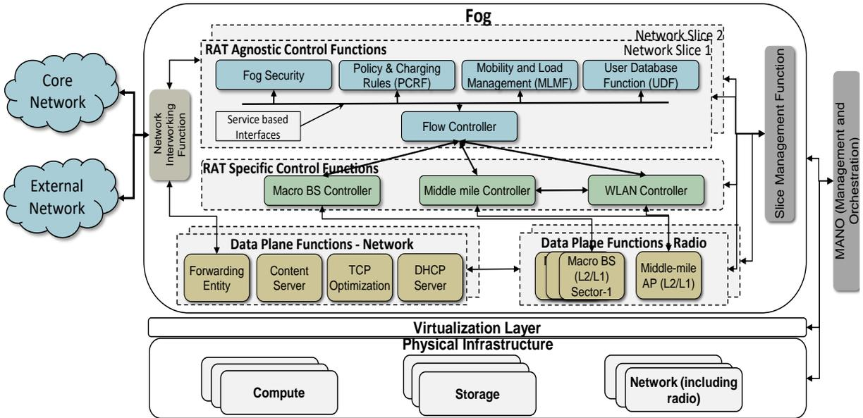
Figure 2.5: Detailed architecture of access network (fog)
