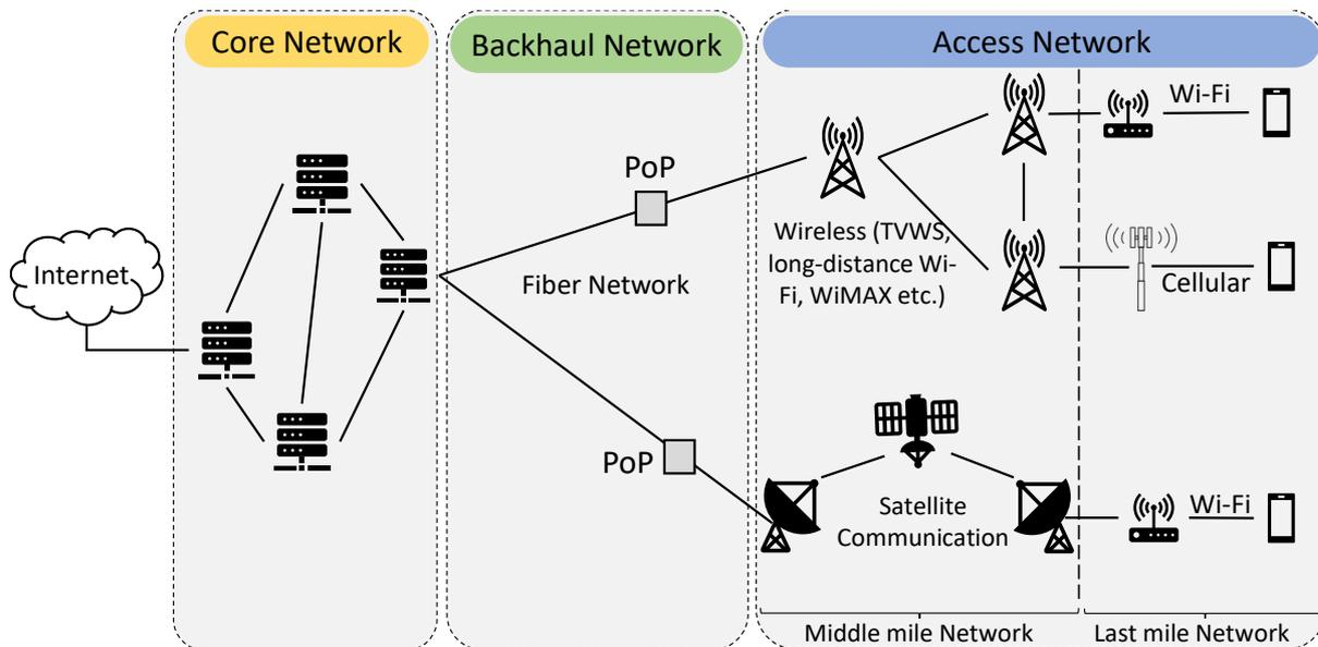
Figure 1.3: A communication network and its components
