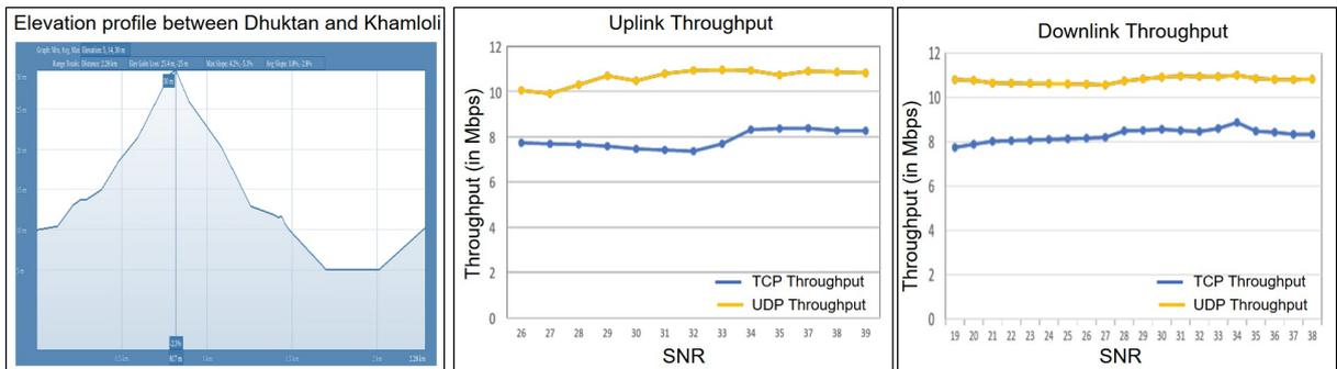
(c) Elevation profile of Dhuktan-Khamloli link along with obtained TCP/User Datagram Protocol (UDP) throughput results are shown. The channel bandwidth was 10 MHz and transmit power was 27 dBm.
