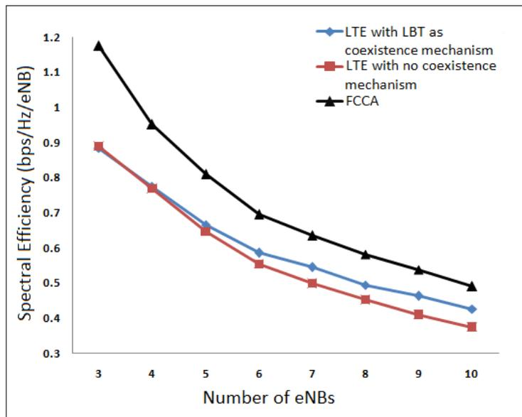
(a) Spectral efficiency of eNB vs. number of eNBs deployed in 100 sq. km area
