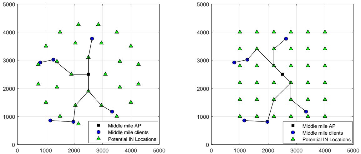
(a) Circular Grid ( $\sum_{i=1}^M U_i = 827$  Mbps and  $\min(U_i) = 95$  Mbps) (b) Square Grid ( $\sum_{i=1}^M U_i = 654$  Mbps and  $\min(U_i) = 109$  Mbps)
