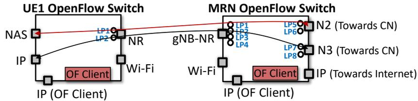
Figure 3.5: Example of flow entries at UE and MRN OpenFlow switch for NAS signaling and data transfer. Figure shows how Logical Ports (LPs) are used to set up a flow in the proposed network.
