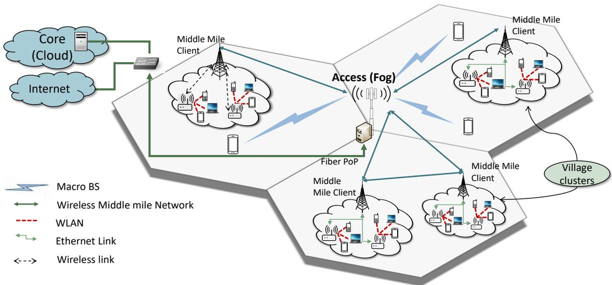
Figure 2.3: A deployment example of Frugal 5G network.
