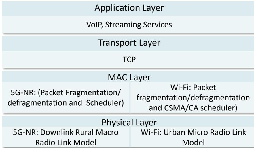
Figure 4.2: Network stack implementation in 5G Multi-RAT simulator
