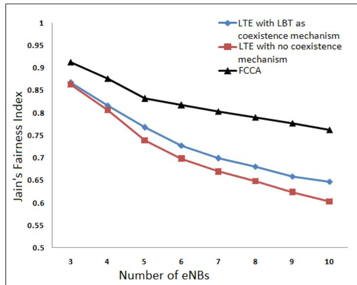
Figure 6.6: Comparative analysis of Jain's fairness index for i) LTE with no coexistence mechanism ii) LTE with LBT as coexistence mechanism and iii) FCCA
