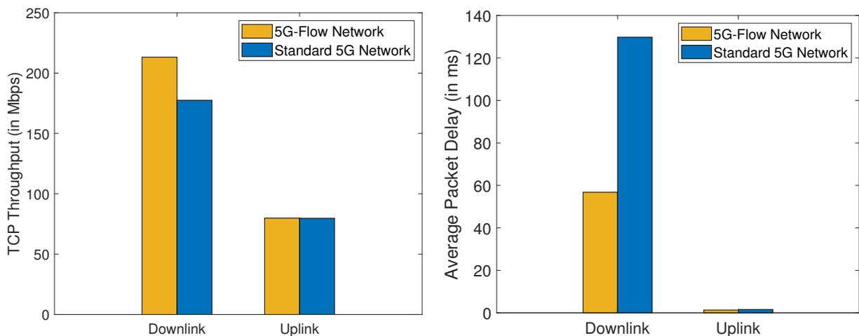
Figure 4.6: Performance comparison between 5G-Flow network and standard 5G network when uplink and downlink data flows are decoupled
