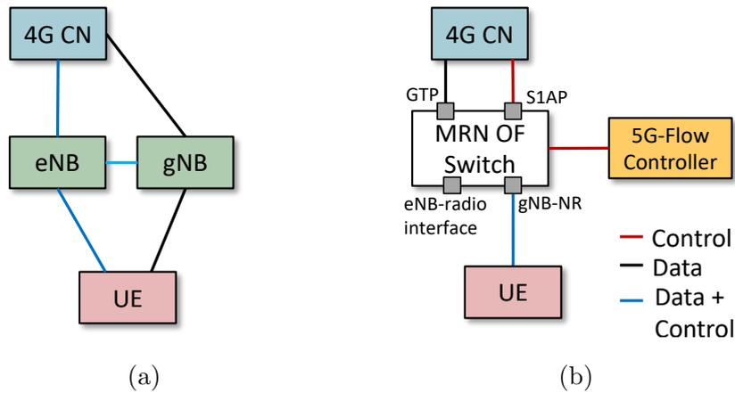
Figure 3.11: Implementation of non-standalone 5G architecture proposed by (a) 3GPP, viz-a-viz (b) 5G-Flow Network
