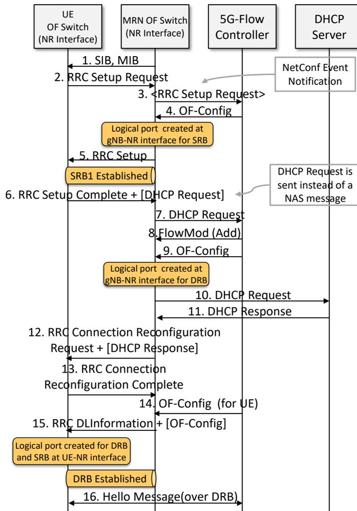
Figure 3.6: Initial connection setup
