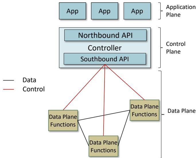
Figure 2.1: Overview of a software defined network
