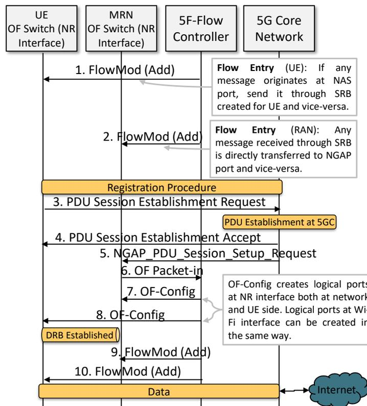
Figure 3.7: Call Flow to illustrate the communication of UE with 5G Core Network
