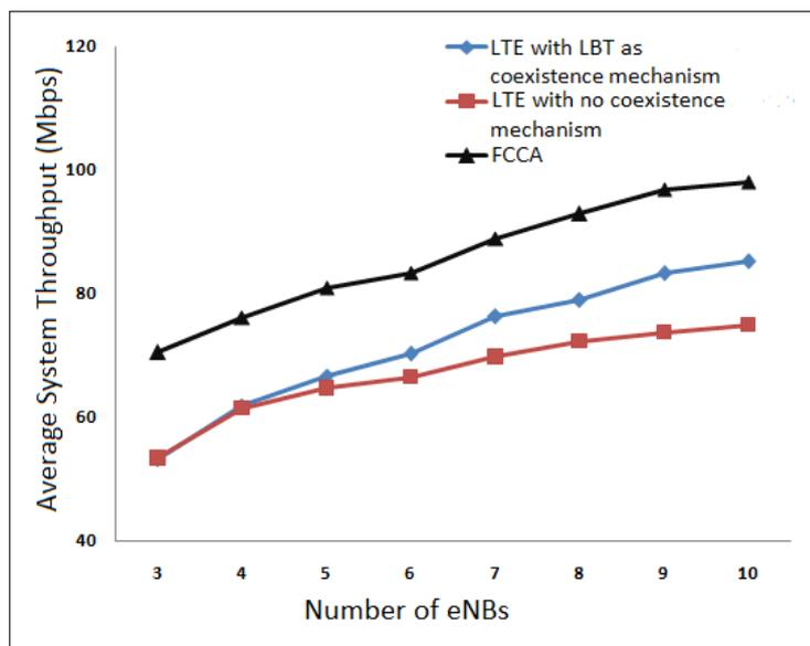
(b) Average throughput per eNB vs. number of eNBs deployed in 100 sq. km area
