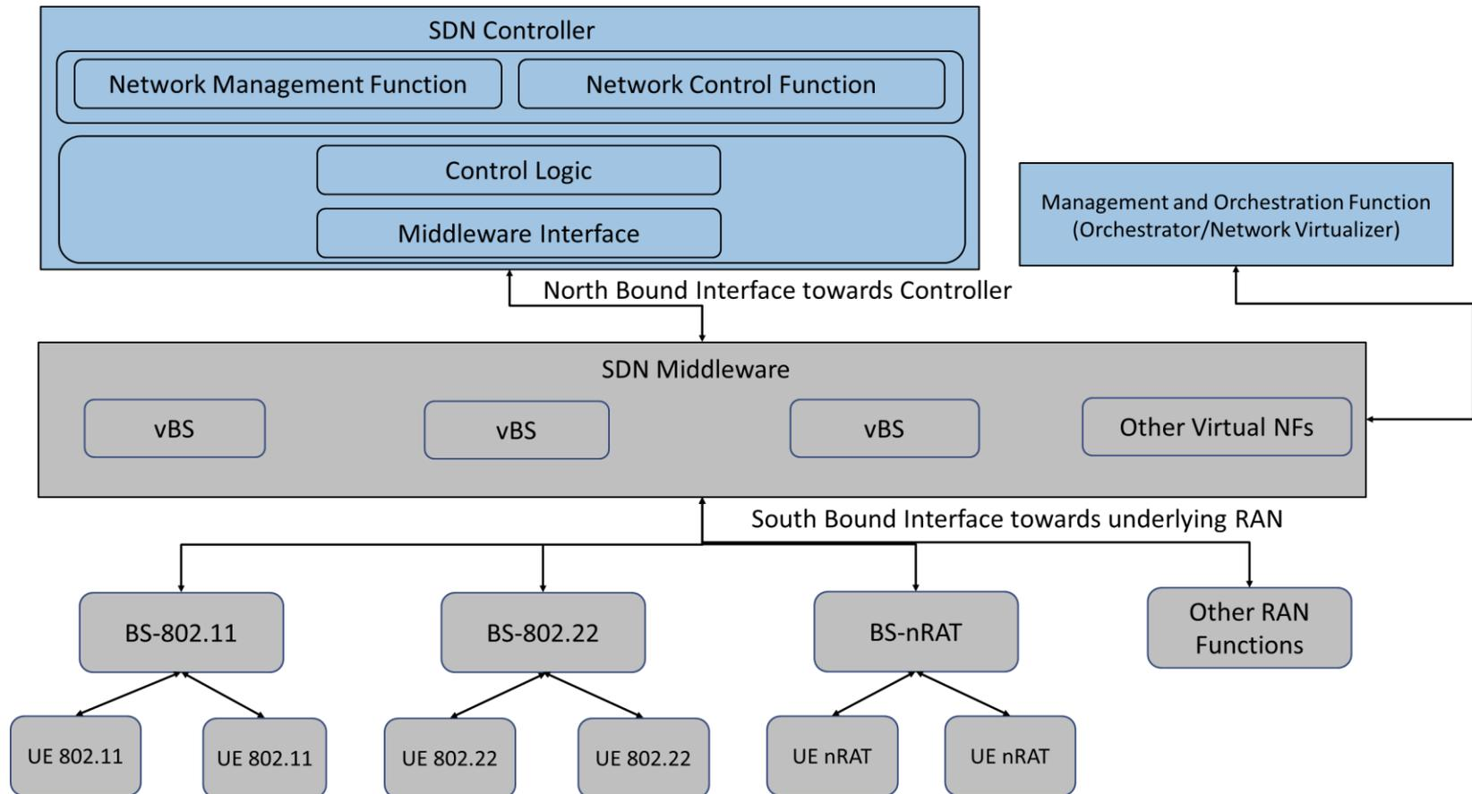
The SDN based RAN architecture proposed in P1930.1 can be used to develop the architecture for Frugal 5G Network
