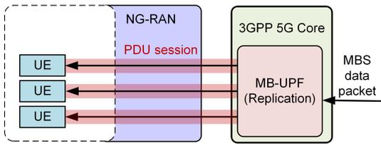
Fig. 3. Individual MBS traffic delivery method. 3GPP: Third Generation Partnership Project, 5G: Fifth Generation, MB-UPF: Multicast/Broadcast User Plane Function, MBS: Multicast Broadcast Services, NG-RAN: Next Generation Radio Access Network, PDU: Protocol Data Unit, UE: User Equipment
