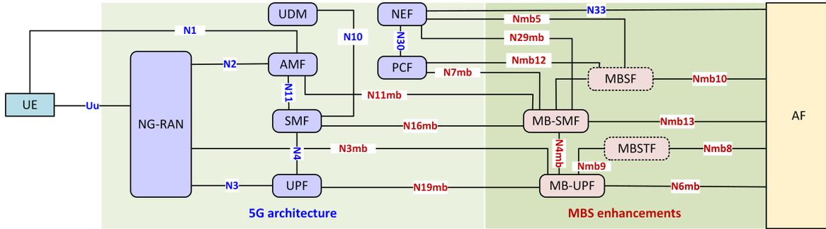
Fig. 1. 5G architecture with MBS enhancements [4]. AMF: Access and Mobility Management Function, AF: Application Function, MB-SMF: Multicast/Broadcast Session Management Function, MBSF: Multicast/Broadcast Service Function, MBSTF: Multicast/Broadcast Session Transport Function, MB-UPF: Multicast/Broadcast User Plane Function., NEF: Network Exposure Function, NG-RAN: Next generation Radio Access Network, PCF: Policy Control Function, UDM: User Data Management, and UE: User Equipment.
