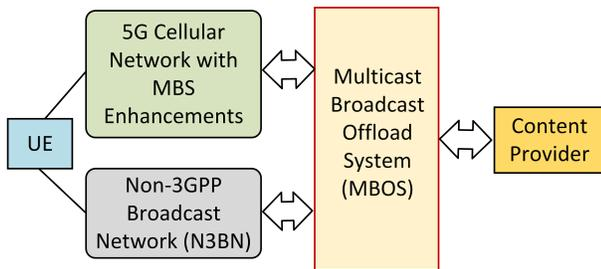
Fig. 8. MBOS for load sharing between 5G and non-3GPP broadcast networks. UE: User Equipment.
