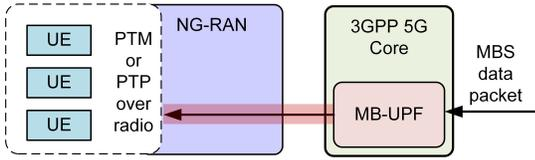
Fig. 2. 5G Shared MBS traffic delivery method. 3GPP: Third Generation Partnership Project, 5G: Fifth Generation, MB-UPF: Multicast/Broadcast User Plane Function, MBS: Multicast Broadcast Services, NG-RAN: Next Generation Radio Access Network, PTM: Point-to-multipoint, PTP: Point-to-point, UE: User Equipment
