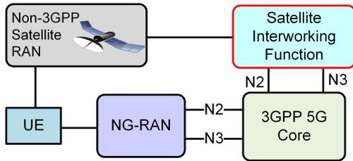
Fig. 6. Integration of non-3GPP satellite access using a new interworking function. NG-RAN: Next Generation Radio Access Network, and UE: User Equipment
