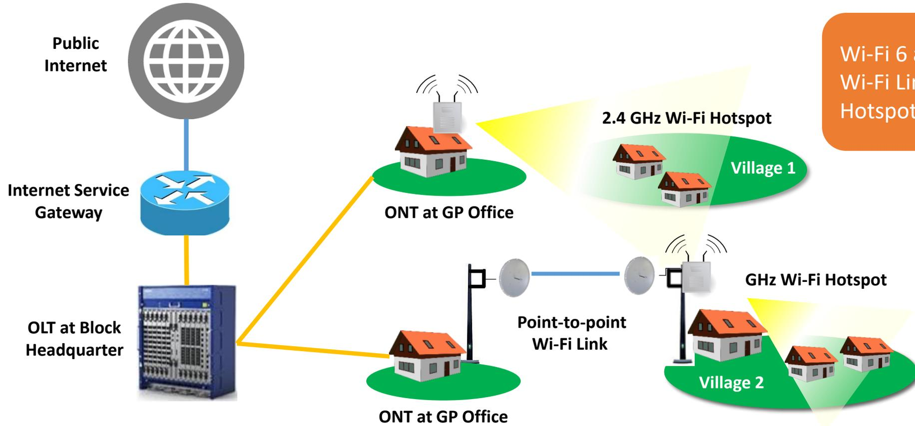
Wi-Fi 6 as Point-to-Point Wi-Fi Links as well as Hotspots
