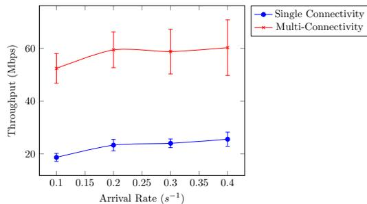
Fig. 8: Median system throughput v/s user arrival rates for different connectivity types.
