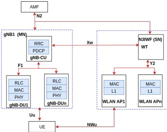
Fig. 3: Block diagram of proposed NR-WLAN Multi-Connectivity architecture.
