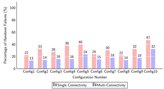
Fig. 7: Percentage of handover failures for various slice configurations.
