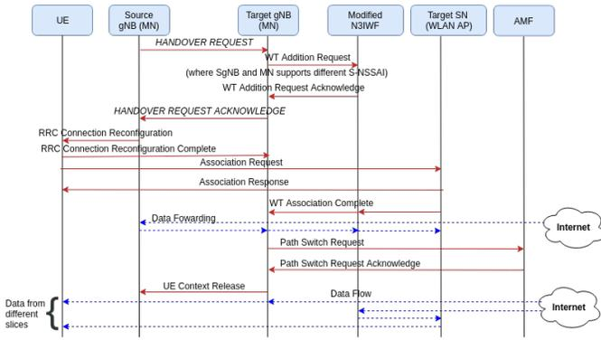
Fig. 5: Slice Handover to both 5G NR and non-3GPP networks using Multi-connectivity.
