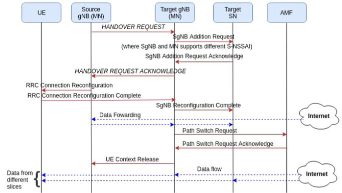
Fig. 4: Slice Handover within 5G NR using Multi-connectivity.
