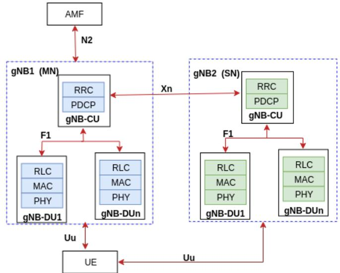
Fig. 2: Block diagram of 3GPP NR Multi-Connectivity architecture.
