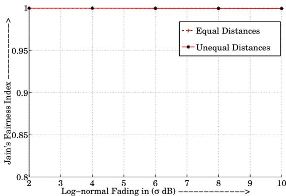
Fig. 5. JFI with Different log-normal Fading using TWUS
