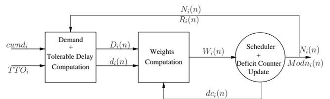
Fig. 3. Block Diagram of the Proposed Uplink Scheduler
