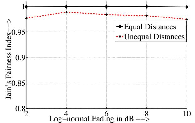
Fig. 5. JFI with Different Log-normal Fading using DTWUS-A
