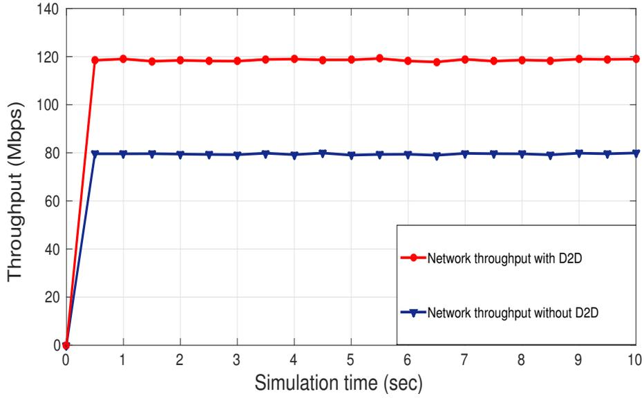
Figure 2.8: Comparison of network throughput for the downlink scenario with and without D2D communication ( $N_C = 100$ ,  $N_D = 20$ ,  $R_{D2D} = 50$  m).
