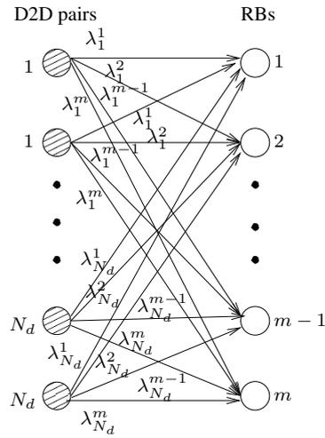
Figure 3.3: Bipartite graph for allocating maximum two resource blocks ( $T = 2$ ) to a D2D pair.
