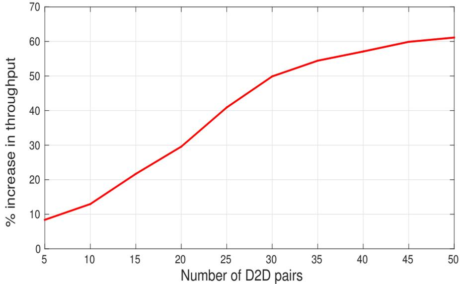
Figure 2.10: Percentage increase in network throughput as the number of D2D pairs increases ( $N_C = 100$ ,  $R_{D2D} = 50$  m).
