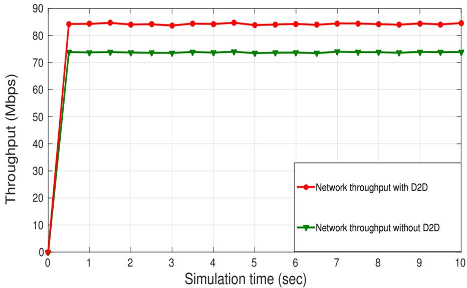
Figure 2.9: Comparison of network throughput for the uplink scenario with and without D2D communication ( $N_C = 100$ ,  $N_D = 20$ ,  $R_{D2D} = 50$  m).
