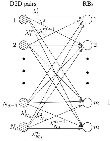
Figure 3.2: Bipartite graph for allocating maximum one resource block ( $T = 1$ ) to a D2D pair.
