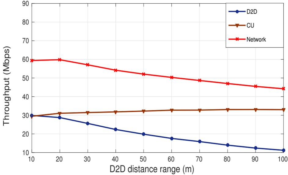
Figure 3.4: Throughput of CUs, D2D pairs and network with increasing D2D range for single resource block allocation ( $N_c = 30$ ,  $N_D = 20$ ,  $T = 1$ ).
