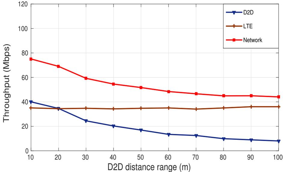
Figure 3.5: Throughput of CUs, D2D pairs and network with increasing D2D range for multiple resource block allocation ( $N_c = 20$ ,  $N_D = 20$ ,  $T = 2$ ).
