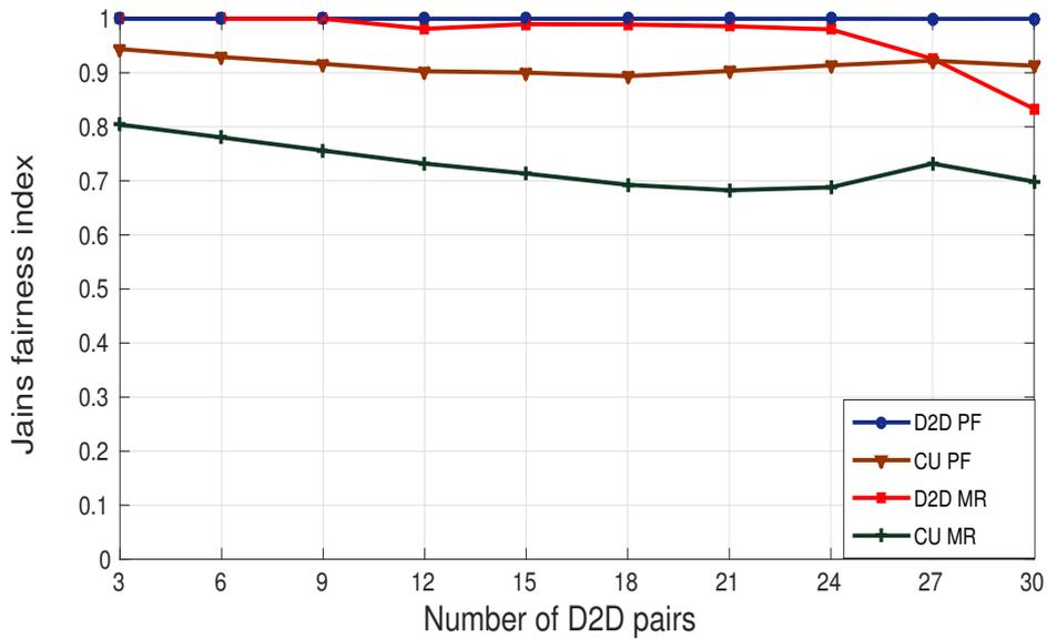
Figure 3.8: Comparison of Jain's fairness index between PF and MR scheduling with increasing number of D2D pairs for single resource block allocation ( $N_C = 30$ ,  $R_{D2D} = 20$  m,  $T = 1$ ).
