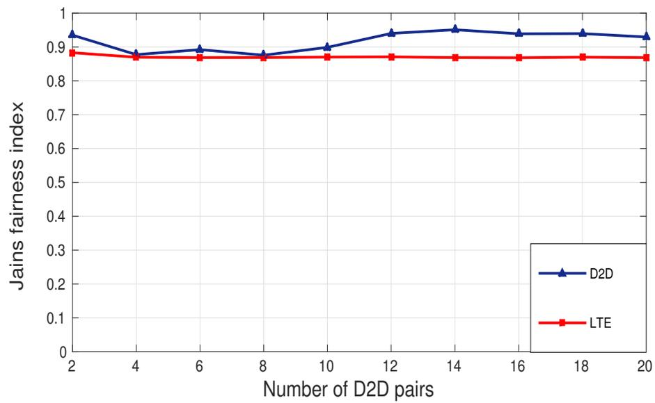
Figure 3.9: Jain's fairness index with increasing number of D2D pairs for multiple resource block allocation ( $N_C = 20$ ,  $R_{D2D} = 20$  m,  $T = 2$ ).
