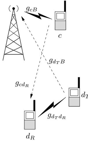
Figure 3.1: Interference scenario for a CU and a D2D pair communicating over common uplink resource blocks.
