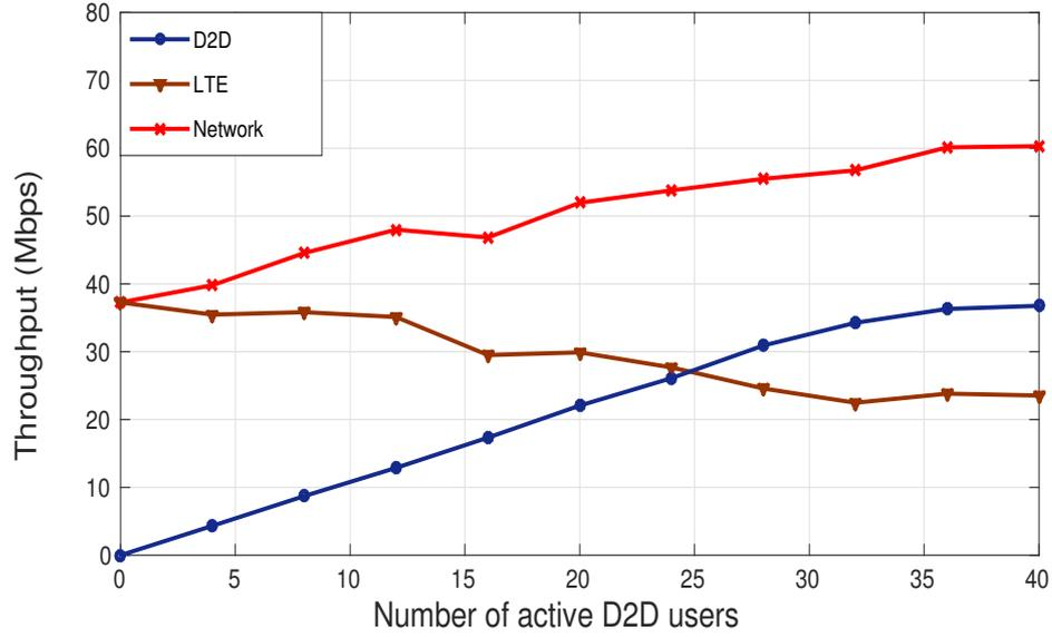
Figure 3.6: Throughput of CUs, D2D pairs and network with increasing number of D2D pairs for single resource block allocation ( $N_C = 40$ ,  $R_{D2D} = 20$  m,  $T = 1$ ).
