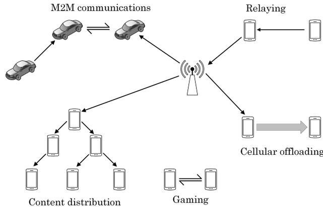
Figure 1.1: Applications of D2D communication.
