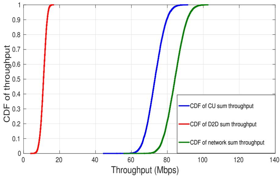
Figure 2.7: CDFs of CU, D2D and network throughput for the uplink scenario ( $N_C = 100$ ,  $N_D = 20$ ,  $R_{D2D} = 50$  m).
