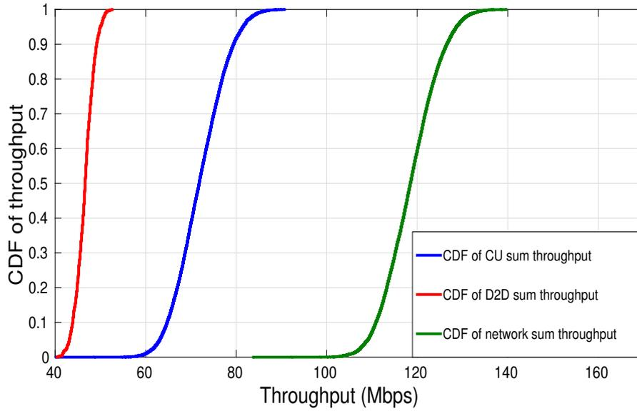
Figure 2.6: CDFs of CU, D2D and network throughput for the downlink scenario ( $N_C = 100$ ,  $N_D = 20$ ,  $R_{D2D} = 50$  m).
