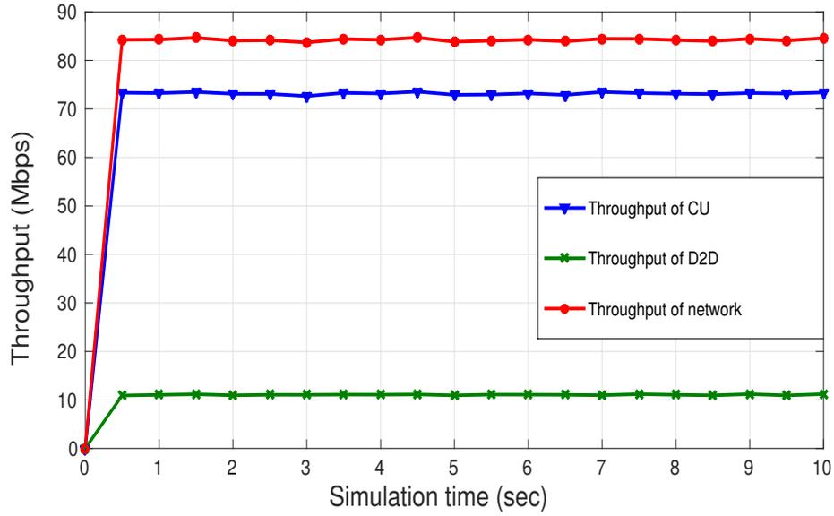
Figure 2.5: Comparison of CU, D2D and network throughput for the uplink scenario ( $N_C = 100$ ,  $N_D = 20$ ,  $R_{D2D} = 50$  m).
