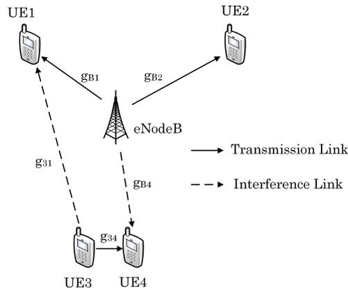
Figure 2.1: Interference scenario for a CU and a D2D pair communicating over common downlink resource blocks.
