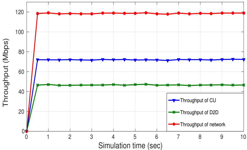
Figure 2.4: Comparison of CU, D2D and network throughput for the downlink scenario ( $N_C = 100$ ,  $N_D = 20$ ,  $R_{D2D} = 50$  m).
