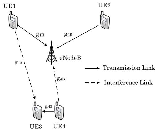
Figure 2.2: Interference scenario for a CU and a D2D pair communicating over common uplink resource blocks.
