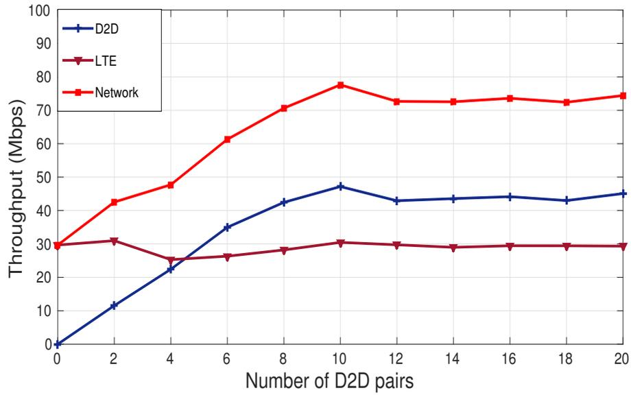
Figure 3.7: Throughput of CUs, D2D pairs and network with increasing number of D2D pairs for multiple resource block allocation ( $N_C = 20$ ,  $R_{D2D} = 20$  m,  $T = 2$ ).
