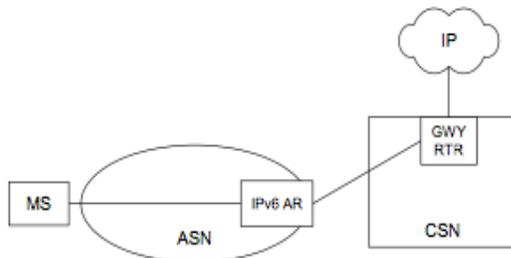
Figure 3: IPv6 in WiMAX Network Architecture
