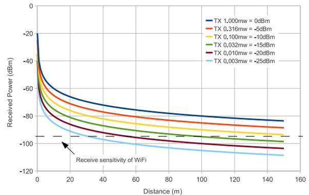
Fig. 10. Free Space Path-loss with Varying transmit power
