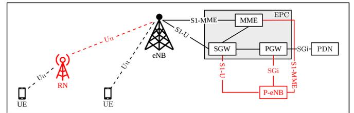
Fig. 2: An illustration of proposed architecture with network elements and their interfaces. The newly defined nodes (RN and P-eNB) and their interfaces are in red color. Note that the architecture reuses the existing standard interfaces: RN uses only Uu interface while P-eNB uses S1-U, S1-MME and SGi interfaces.
