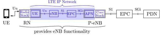
(c) Abstract view of the proposed architecture. The two protocol stacks of an eNB are distributed between RN and P-eNB and connected via LTE IP network. The eNB radio stack of the RN and the CN stack of the P-eNB in conjunction provide eNB functionality to the UE connected to the RN.
