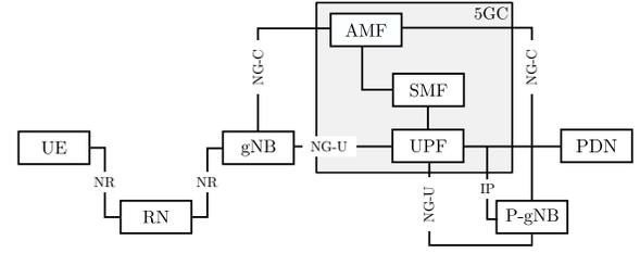
(a) An illustration of proposed architecture with interfaces.
