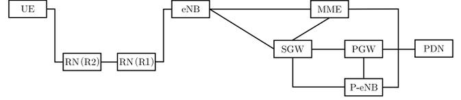
Fig. 5: An illustration of multihop relay communications in LTE network. R2 uses R1 data bearer, and UE uses R2 data bearer to communicate to CN.
