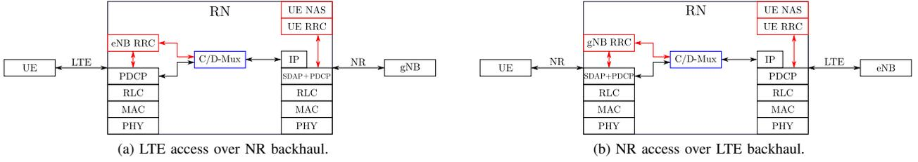
Fig. 7: Protocol stacks at RN, for Alternative 1, to support different combinations of access and backhaul for LTE and 5G.
