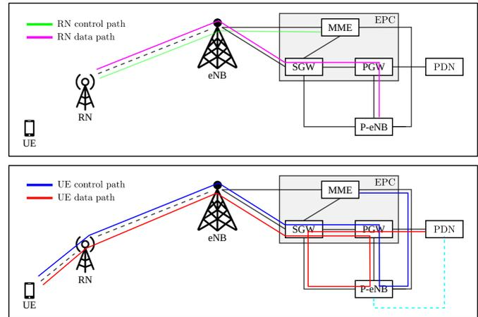
Fig. 4: An illustration of control and data paths for both UE and RN. As RN behaves as an UE, the control and data paths for RN follows the corresponding standard 3GPP UE paths with P-eNB as APN. The UE uses data path of the RN for both its control and data paths. The control path for the UE follows UE→RN→(RN data path)→P-eNB→MME, and the data path for the UE follows UE→RN→(RN data path)→P-eNB→SGW→PGW→PDN.
