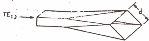
FIG. 14. Transformation from rectangular waveguide to diagonal horn.
