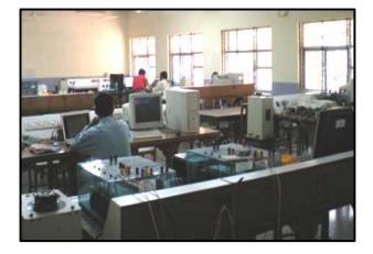
**Power Electronics Lab** – I: In this laboratory, research on the application of inverters for active power filters, switched reluctance motors and parallel operation of inverters in a microgrid are carried out. The inverters under use are three phase three wire and three phase four wire inverters fabricated by SEMIKRON.
