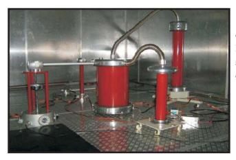
**Insulation Diagnostics Lab:** This recently developed laboratory has a 100 kV AC / 140 kV DC setup. It is also equipped with a partial discharge measurement setup. Research in this lab is in the fields of Partial discharge, Insulation life evaluation, Dielectric breakdown.
