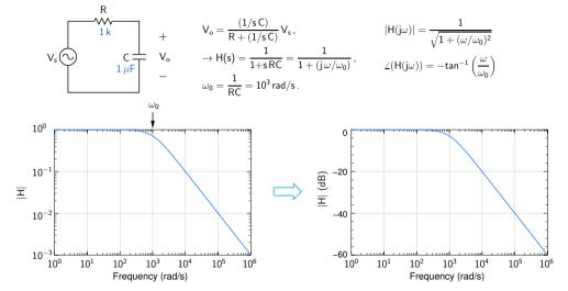
Note that the *shape* of the plot does not change. |H| (dB) = 20 log |H| is simply a scaled version of log |H|.
