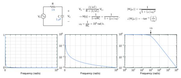
Since  $\omega$  and  $|H(j\omega)|$  vary by several orders of magnitude, a linear  $\omega$ - or |H|-axis is not appropriate  $\rightarrow \log |H|$  is plotted against  $\log \omega$ .
