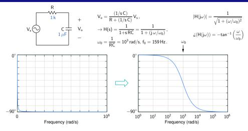
\* Since  $\angle H = -\tan^{-1}(\omega/\omega_0)$  varies in a limited range (0° to -90° in this example), a linear axis is appropriate for  $\angle H$ .
