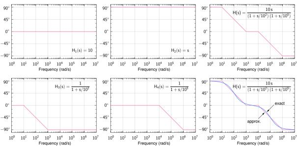
\* As we have seen, the contribution of a pole to the magnitude and phase plots is well represented by the asymptotes when  $\omega \ll p$  or  $\omega \gg p$  (similarly for a zero).
