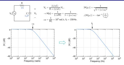
Since  $\omega = 2\pi f$ ,  $\log \omega = \log(2\pi) + \log f$  which causes a shift in the x direction, but the shape of the plot does not change.
