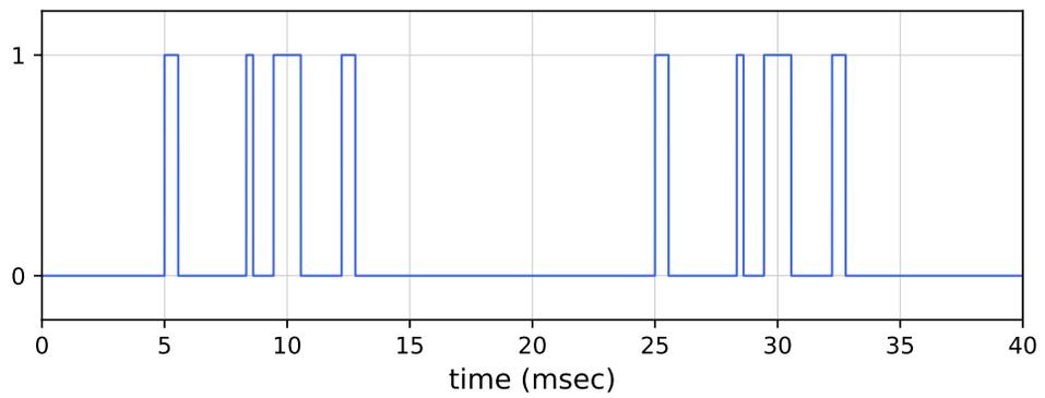
Figure 1:  $y(t)$  obtained with  $n_{data}=8$ ,  $frequency=50$ ,  $theta_1=90$ ,  $theta_2=100$ ,  $theta_3=150$ ,  $theta_4=155$ ,  $theta_5=170$ ,  $theta_6=190$ ,  $theta_7=220$ ,  $theta_8=230$ ,  $theta_{delay}=0$ .
