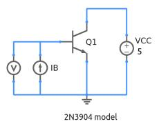
In a BJT, the current gain  $\beta$  varies as a function of the bias collector current  $I_C$  although we often ignore this dependence in circuit analysis. The purpose of this example is to illustrate this relationship.
