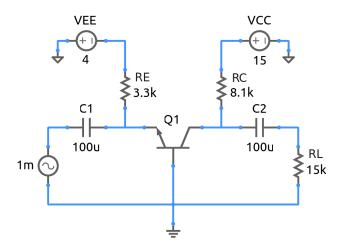
Shown in the figure is a common-base amplifier. We are interested in computing the mid-band gain of the amplifier. Assume that the BJT is working in the active mode.
